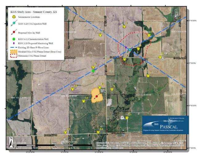
Image take from "Small scale field test demonstrating CO2 sequestration in Arbuckle saline aquifer and by CO2-EOR at Wellington field, Sumner County, Kansas", presentation given at DOE Carbon Storage R&D Project Review Meeting, August 21-23, 2012 by W. Lynn Watney & Jason Rush (Joint PIs).
