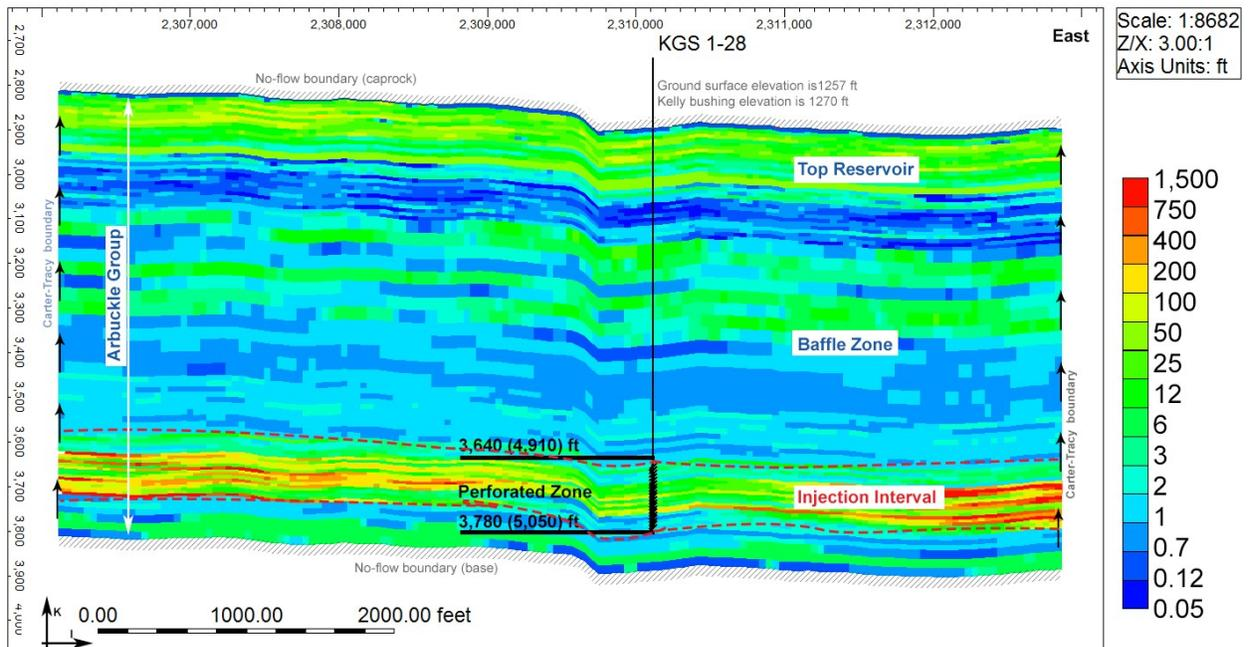
**Figure 16. Horizontal permeability (mD) distribution within an east-west cross section through the injection well (KGS 1-28), vertical cross-section A-A'. Location of cross section shown in Figure 13.**
