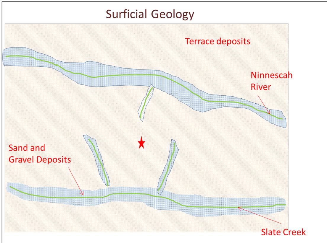
**Figure 6. Interfluvial area with thin, surficial Pleistocene terrace deposits and soil over Wellington in light tan color. Red star is location of Wellington Field. Generally, thick sand and gravel present in incised valleys that cut the older Pleistocene terraces. Incised valleys commonly lie beneath modern streams and alluvium and combine to form a viable shallow aquifer system.**
