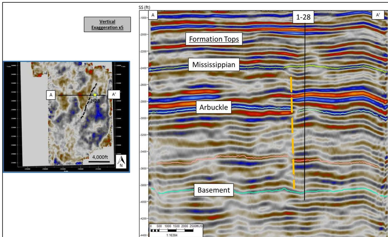
**Figure 10. Medial fault as viewed in a west-to-east seismic amplitude profile with 5x exaggeration. Fault delineated as the orange dashed line is approximately 530 feet west of (Class VI) well #1- 28 at the injection interval of 5000 ft, depth intermediate between the arbitrary mid Arbuckle marker horizon (solid orange line) and the basement (turquoise line). The Arbuckle injection well is the vertical black line. (Courtesy of D. Schwab, KGS/KU).**
