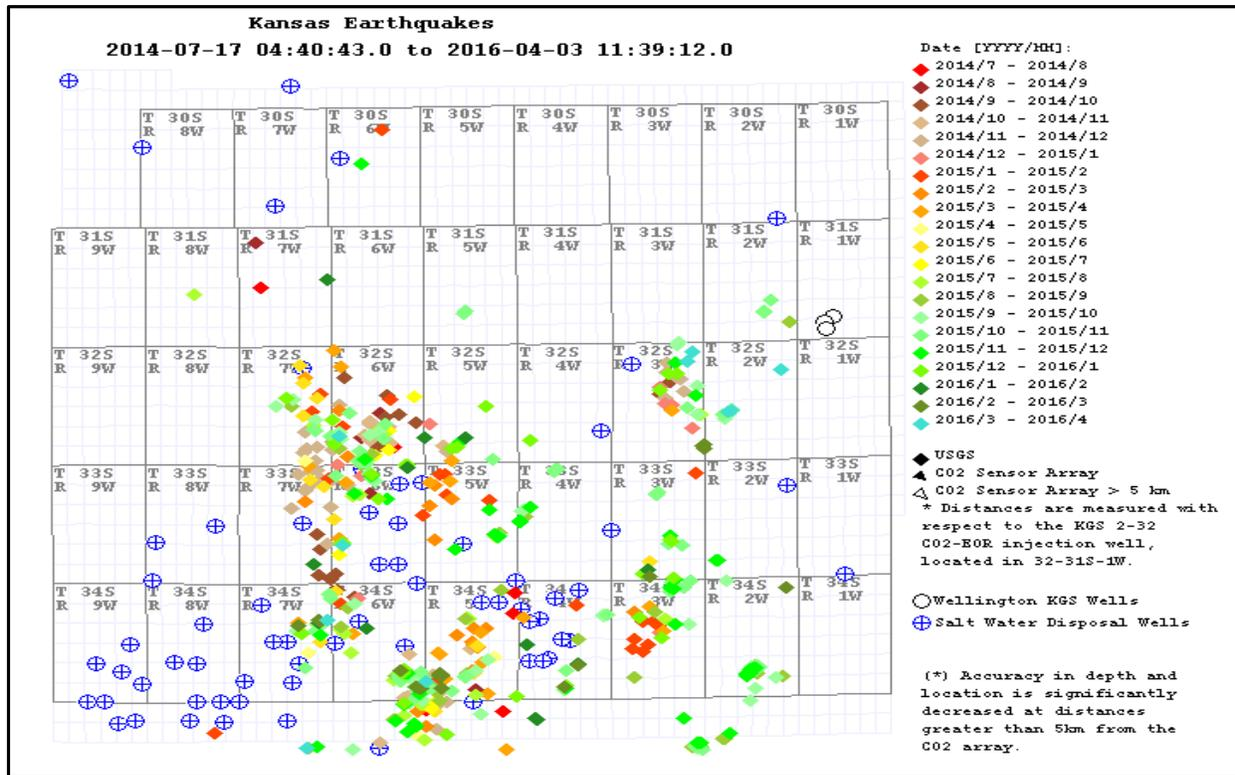
**Figure 31. Java based map showing dates of earthquakes in south-central Kansas from the NEIC catalog between July 17, 2014 and April 3, 2016. Three KGS wells drilled in Wellington field are shown by three open circles in T31s-R1w in northeast corner of the map. Map generated by KGS Java Applet, Kansas Earthquakes 3D Plot -- [http://www.kgs.ku.edu/PRS/Ozark/Software/KS\\_Earthquake\\_3DPlot/index.html](http://www.kgs.ku.edu/PRS/Ozark/Software/KS_Earthquake_3DPlot/index.html)**
