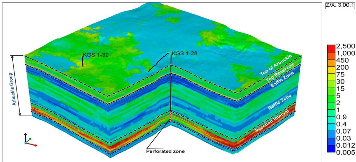
Figure 17. Upscaled vertical permeability (mD) distributions in the Arbuckle Group derived from Petrel geomodel.
