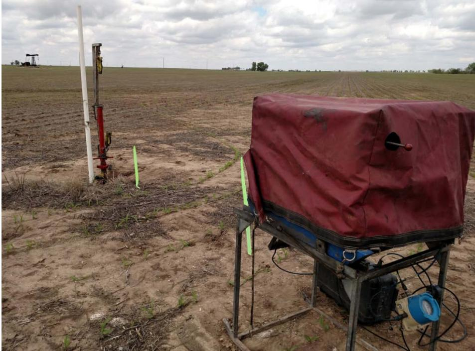
**Figure 39. Wellington KGS #1-28 equipped with pressure transducer to continuously record small pressure changes in the lower Arbuckle**
