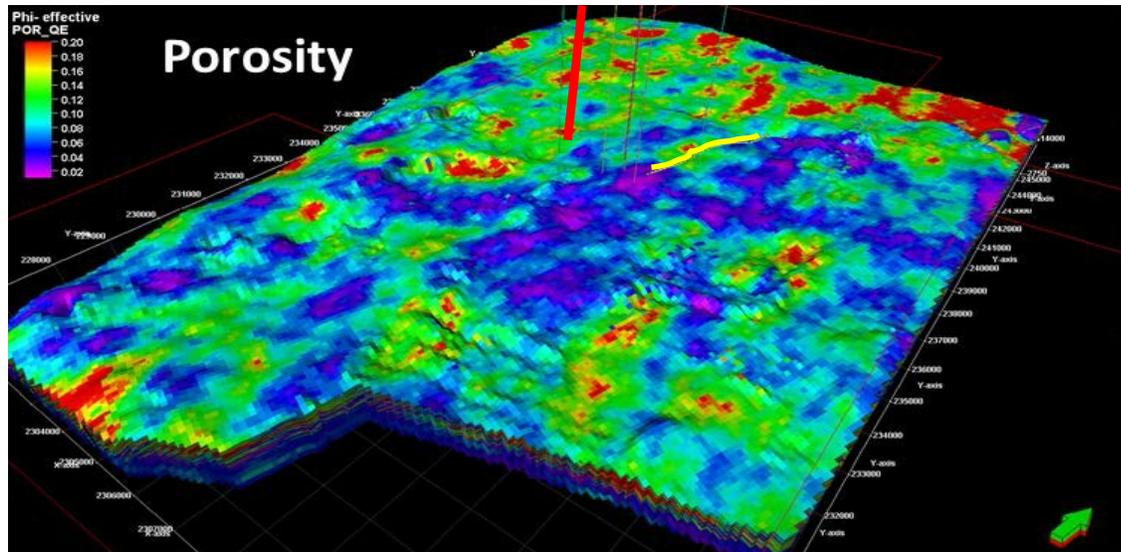
Figure 21. Petrel-based porosity map of the Mississippian reservoir at Wellington Field. CO2 injection well is red colored vertical line near middle of the map. Low porosity noted east and south of the injection well, KGS #2-32. Very thin north-northwest trending yellow line is the trace of the medial fault.
