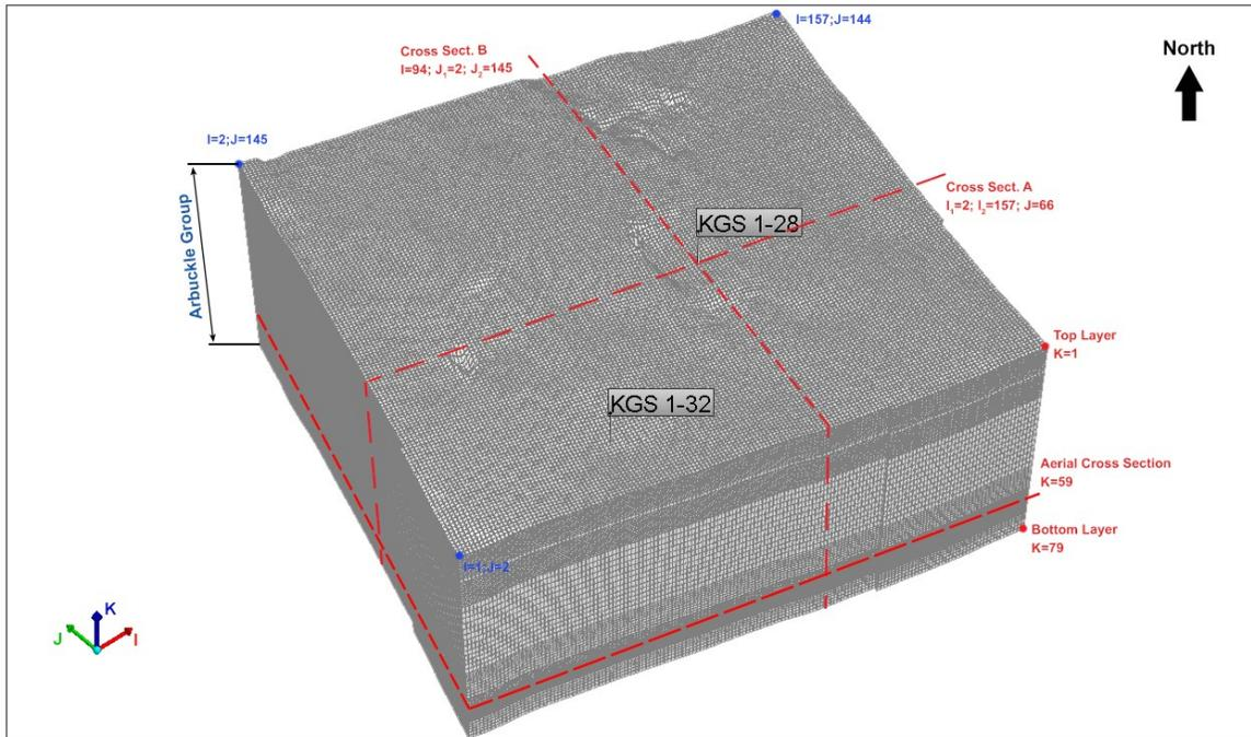
Figure 13. --Model mesh in 3-D showing location of Arbuckle injection and monitoring wells along with the east-west and north-south cross sections. Note the small declivity on the top of the Arbuckle produced by the medial fault.
