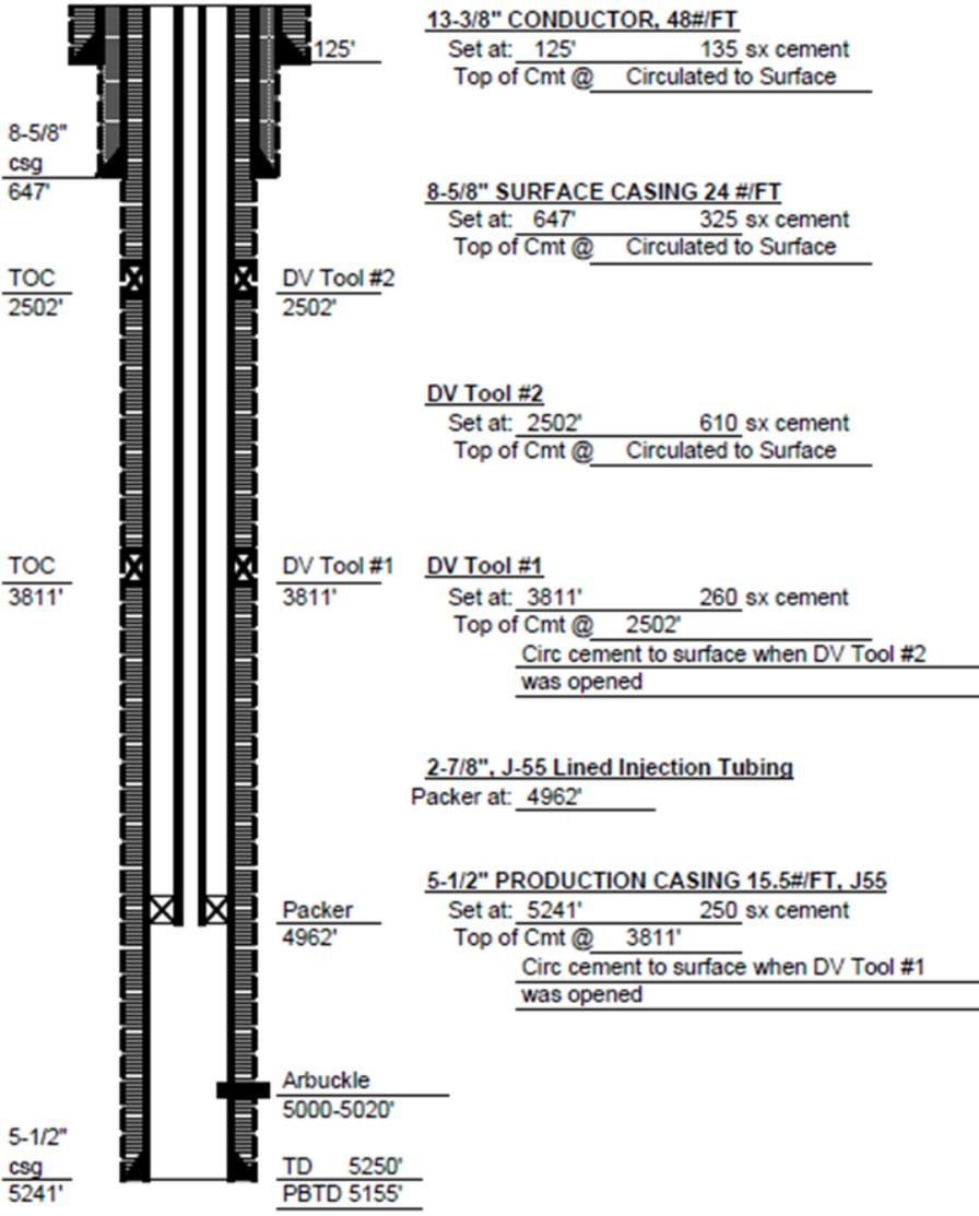
Figure 41. Wellbore schematic of well #1-28 showing perforation at depth of 5000 to 5020 ft.
