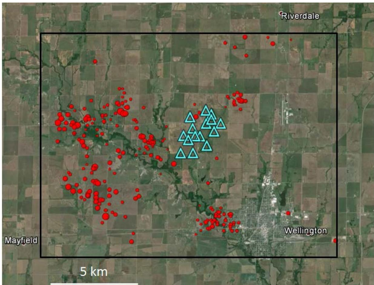
**Figure 33. Map showing all events within the approximate area of interest. Wellington stations are the blue triangles and earthquakes are the red circles with diameter proportional to event magnitude. All events in this area were used to calculate a preliminary Magnitude of Completeness (from Nolte et al., 2016).**
