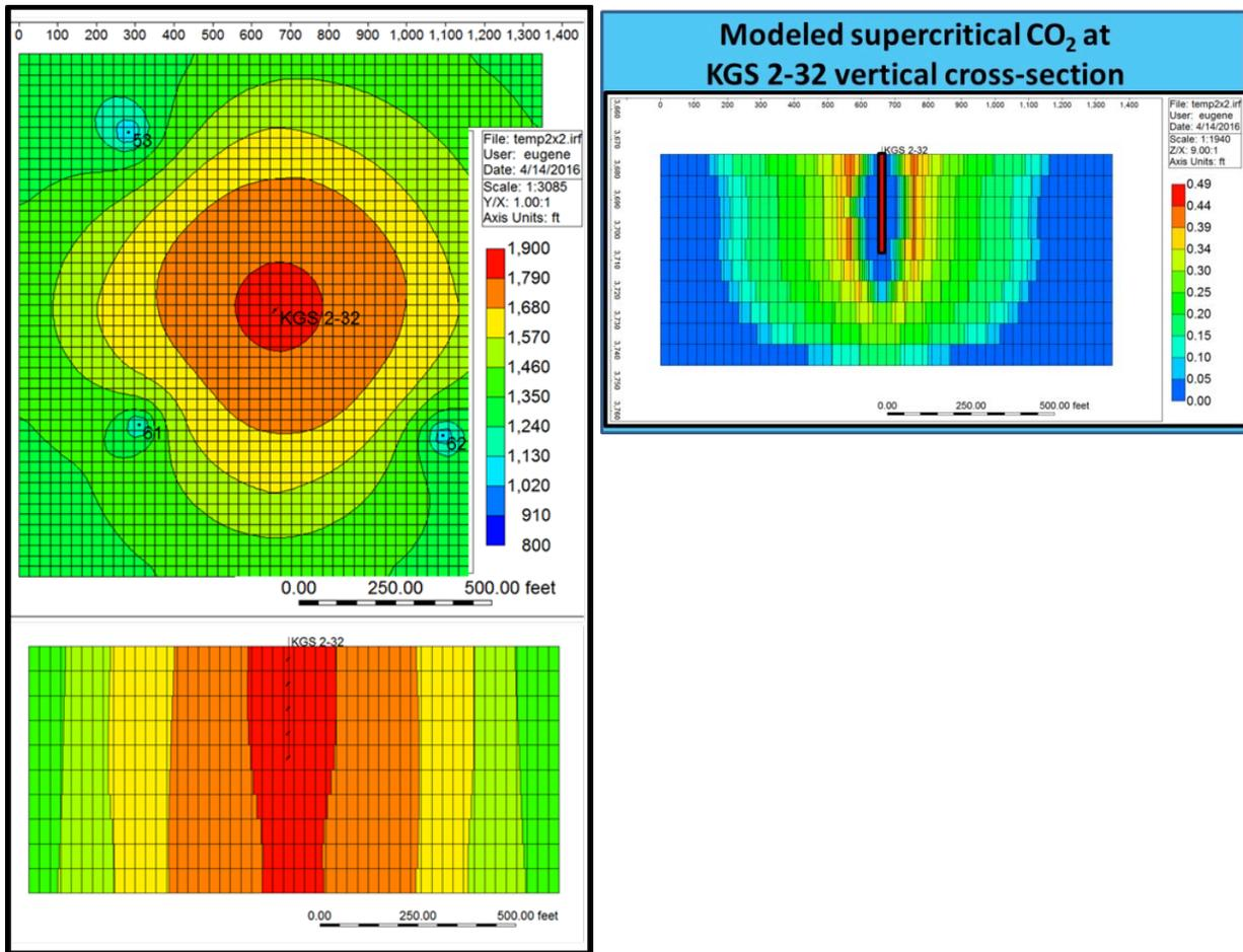
**Figure 58. Simulation of phase and pressures of the CO<sub>2</sub> injected into the Mississippian reservoir**
