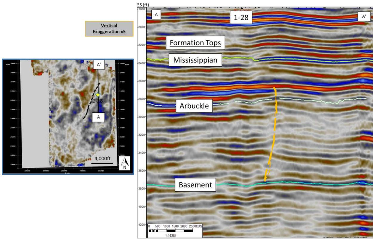
**Figure 11. Medial fault as viewed in a south-to-north seismic amplitude profile vertical exaggeration of 5x. This south-to-north seismic profile runs nearly parallel to the fault and is located near the northern terminus of the fault. The fault line is a projection of where it crosses this section. Class VI injection well #1-28 is shown by the vertical black line. (Courtesy of D. Schwab, KGS/KU).**
