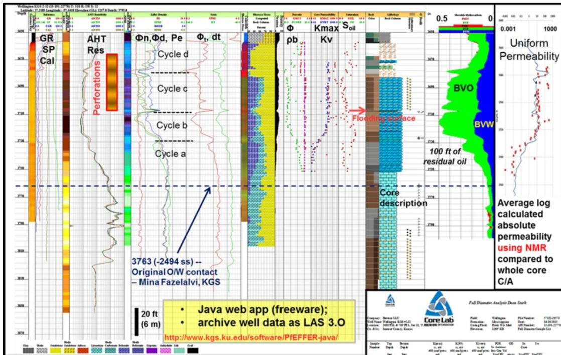
Figure 59. Wellbore profile the CO<sub>2</sub> injection well, Wellington KGS #2-32.
