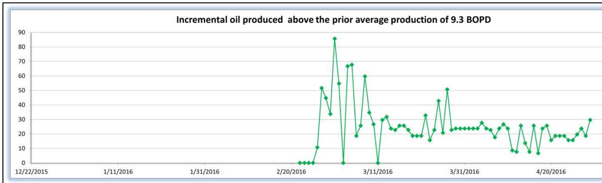
**Figure 52. Incremental oil recovery from the Nelson East tank battery. The slight increase in oil recovery in late April may have been in response to the increased CO<sub>2</sub> injection since late April.**
