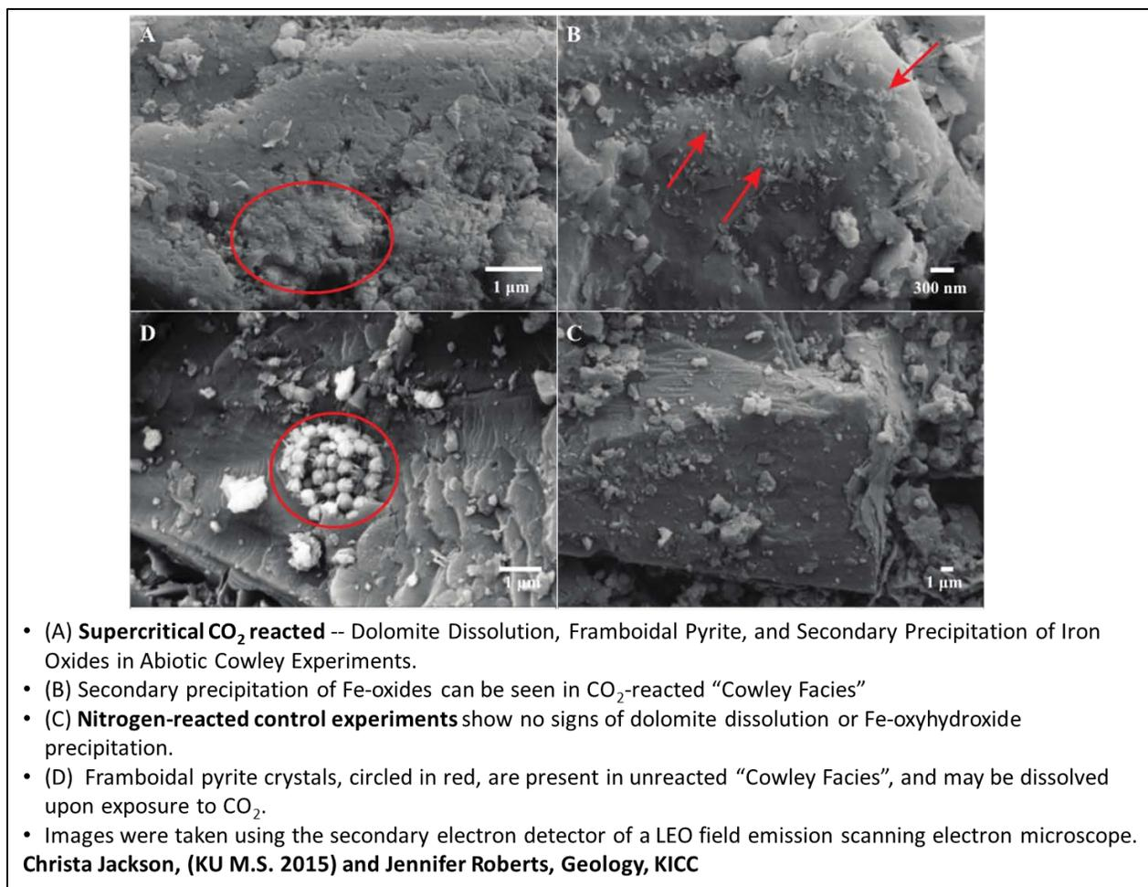
**Figure 65. Scanning electron microscopy was conducted on samples of Mississippian dolomite that were subjected to supercritical CO<sub>2</sub>. Dissolution of dolomite and pyrite and precipitation of iron oxides were noted.**
