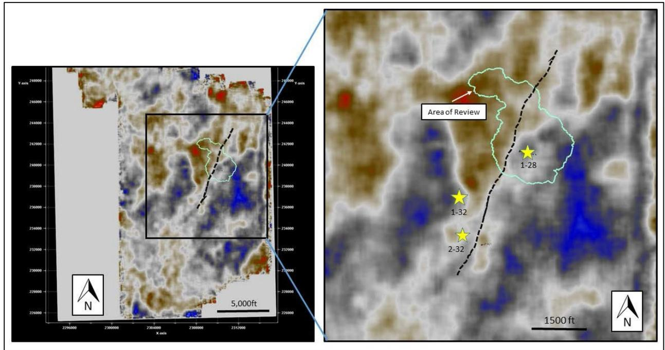
**Figure 8. Map view of the near vertical medial fault near the Class II (#2-32) and Class VI (#1-28) injection wells in Wellington Field as shown on a horizontal amplitude slice of the 3D Petrel model at the base of the Arbuckle at ~5000ft. (the depth of the proposed Class VI injection). The width of the fault as shown on the map is proportional to the vertical offset. (Courtesy of D. Schwab, KGS/KU).**
