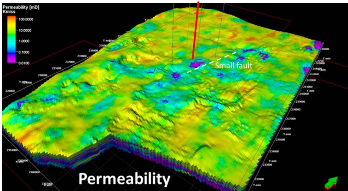
Figure 46. Petrel geomodel showing permeability distribution near the CO<sub>2</sub>-EOR injection well, Berexco KGS #2-32, identified by the red vertical line (Rush, Holubnyak, and Fazalalavi).
