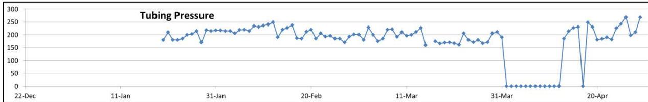
**Figure 50. Tubing pressure has increased since CO<sub>2</sub> injection was restarted (zero tubing pressure) on April 13<sup>th</sup>.**
