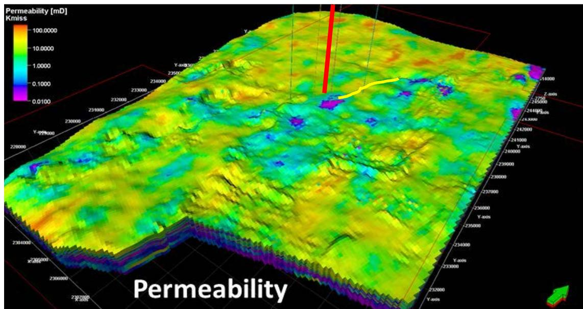
Figure 22. Petrel-based map of permeability for the Mississippian oil reservoir. CO2 injection well is red colored vertical line near middle of the map. Lower permeability noted east and
