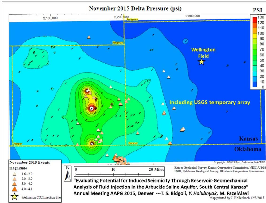
**Figure 38. Regional pressure produced in Arbuckle from large volume and rate brine disposal prior to 2014. Higher pressure in inner core of brine disposal.**
