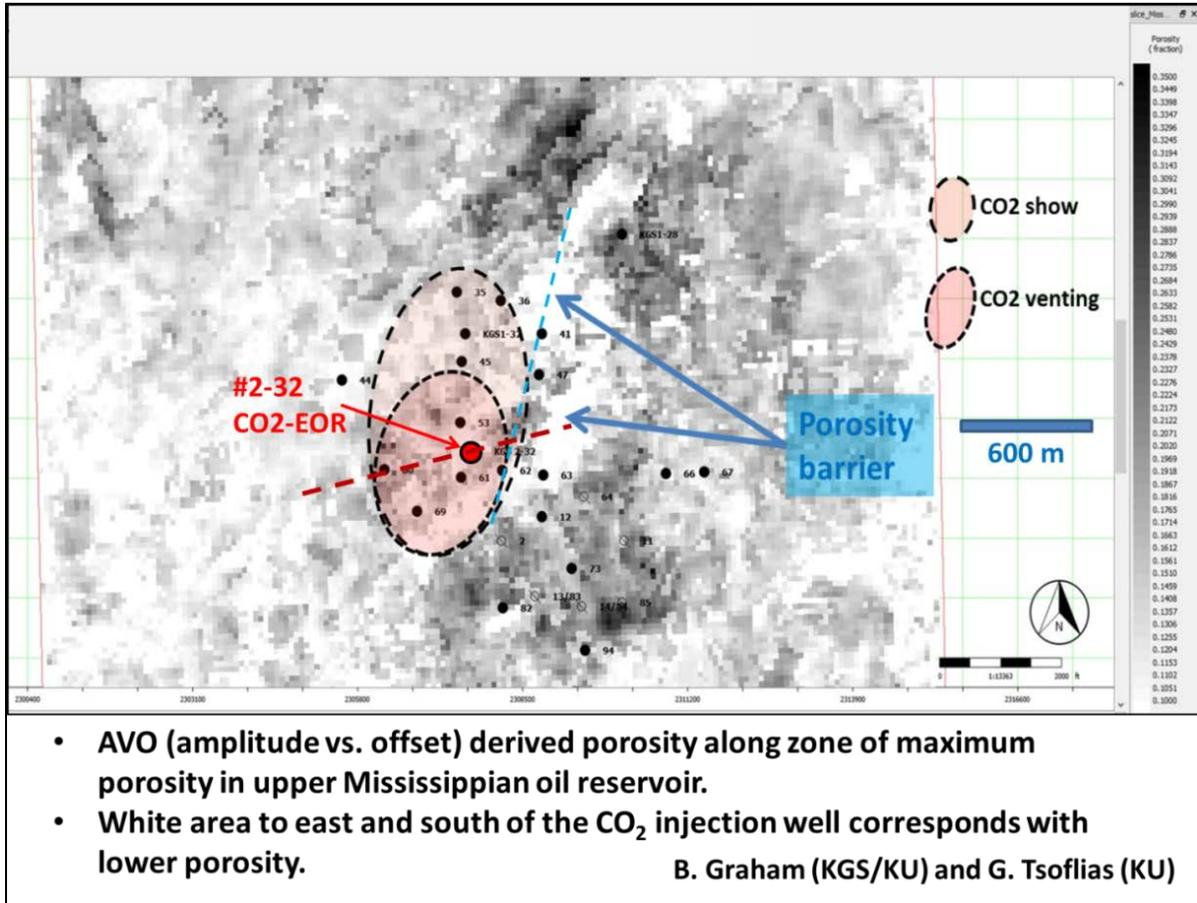
**Figure 60.** AVO map of the porosity along the maximum porosity illustrating the low porosity (area of more solid white) bordering the east and south sides of the CO<sub>2</sub> plume outlined in black dashed line.
