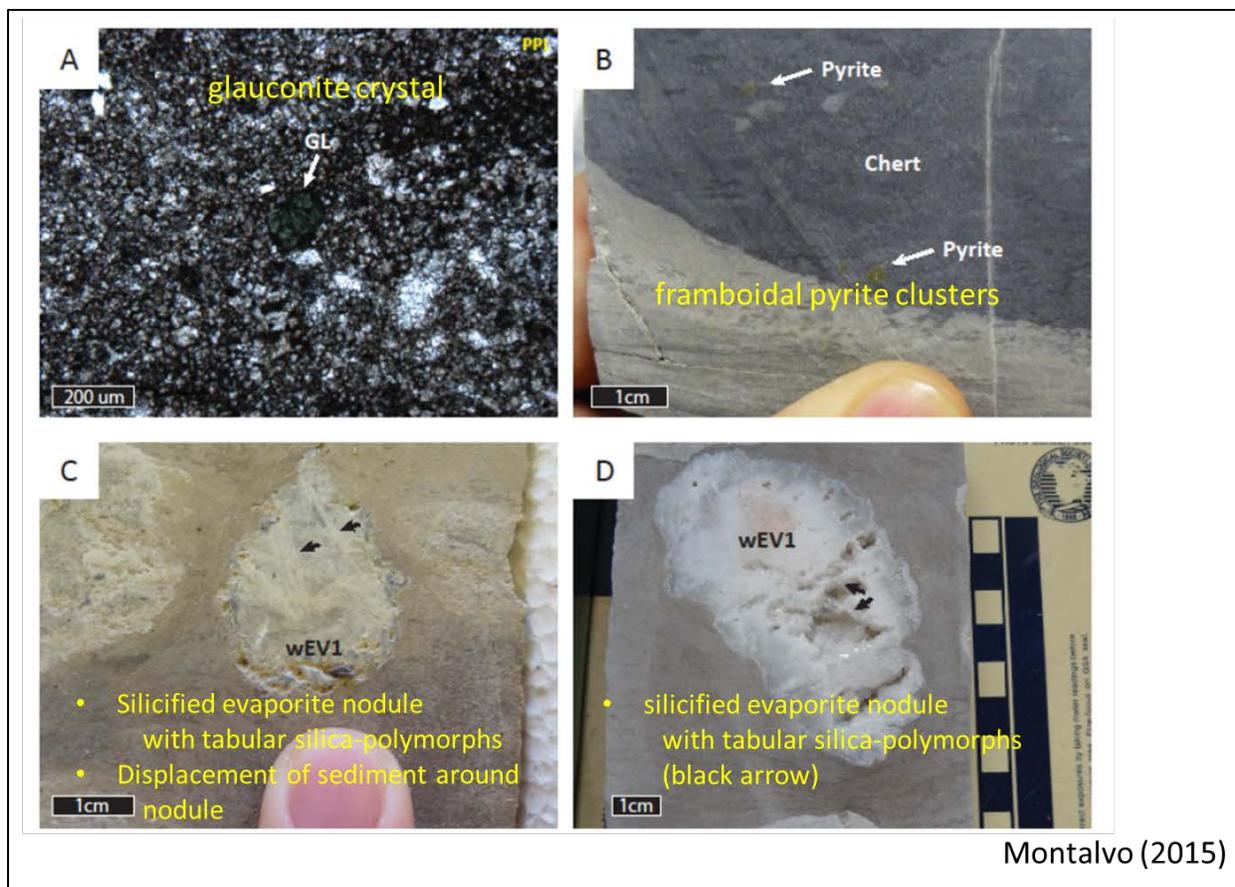
**Figure 64. Accessory minerals present in the Mississippian oil reservoir include pyrite, glauconite, and anhydrite, the later distributed as nodules in part replaced by silica.**
