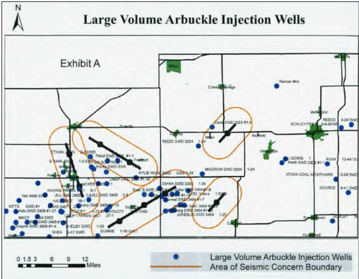
**Figure 26. Reduction of rates of injection into the Arbuckle applicable to wells in defined areas of increased seismic activity in Harper and Sumner Counties in KCC Order Reducing Saltwater (Docket No. 15-CONS-770-CMSC).**
