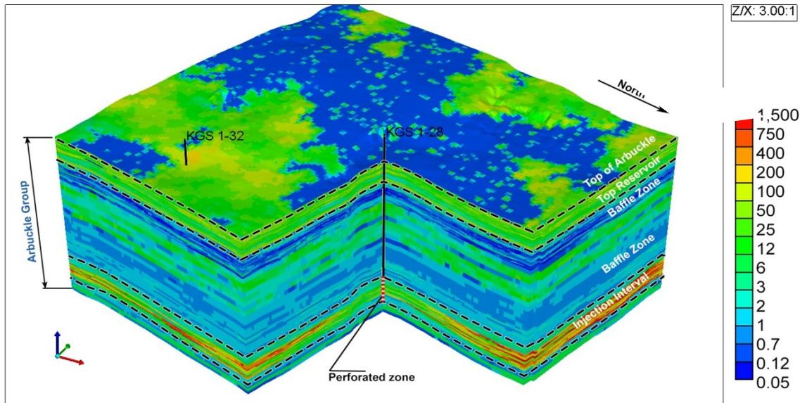
**Figure 15. Upscaled horizontal permeability (mD) distributions in the Arbuckle Group derived from Petrel geo-model. The permeability is reduced in the injection zone in the vicinity of KGS #1-28.**
