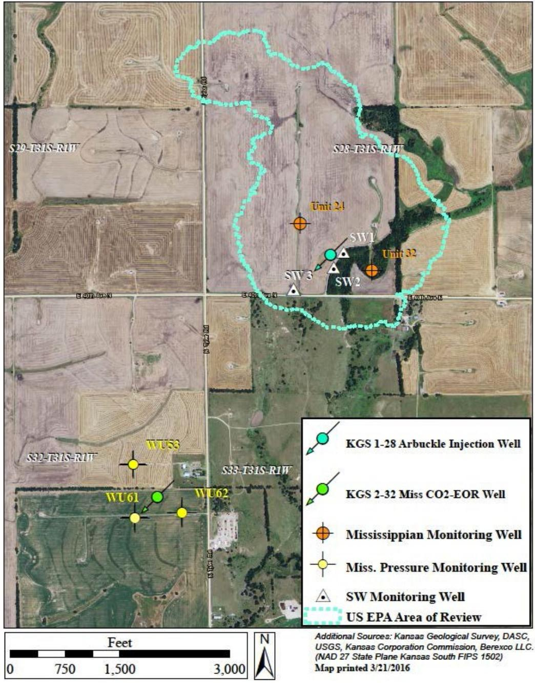
Figure 23. Location of observation wells that are continuously monitored for pressure at the Wellington Enhanced Oil Recovery (EOR) site.
