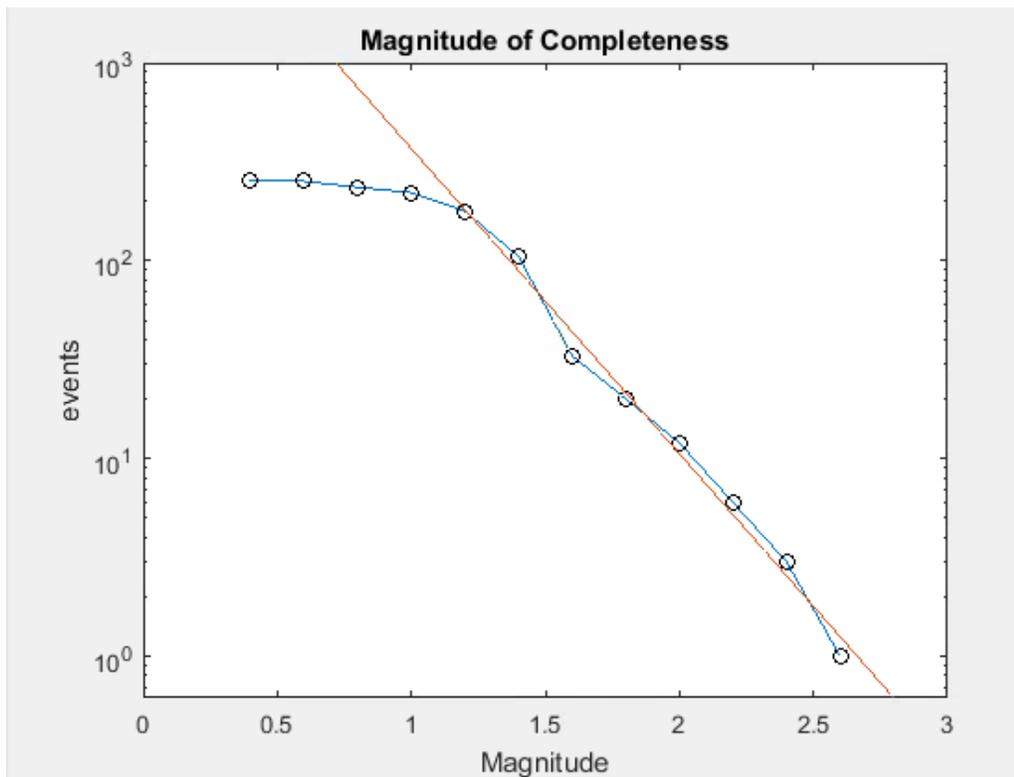
**Figure 35.** Graph showing the Magnitude of completeness, calculated from the Gutenberg-Richter law. The blue line with circles represents events recorded from the seismometer array and orange line represents predicted events using equation 1 from the Gutenberg-Richter law.
