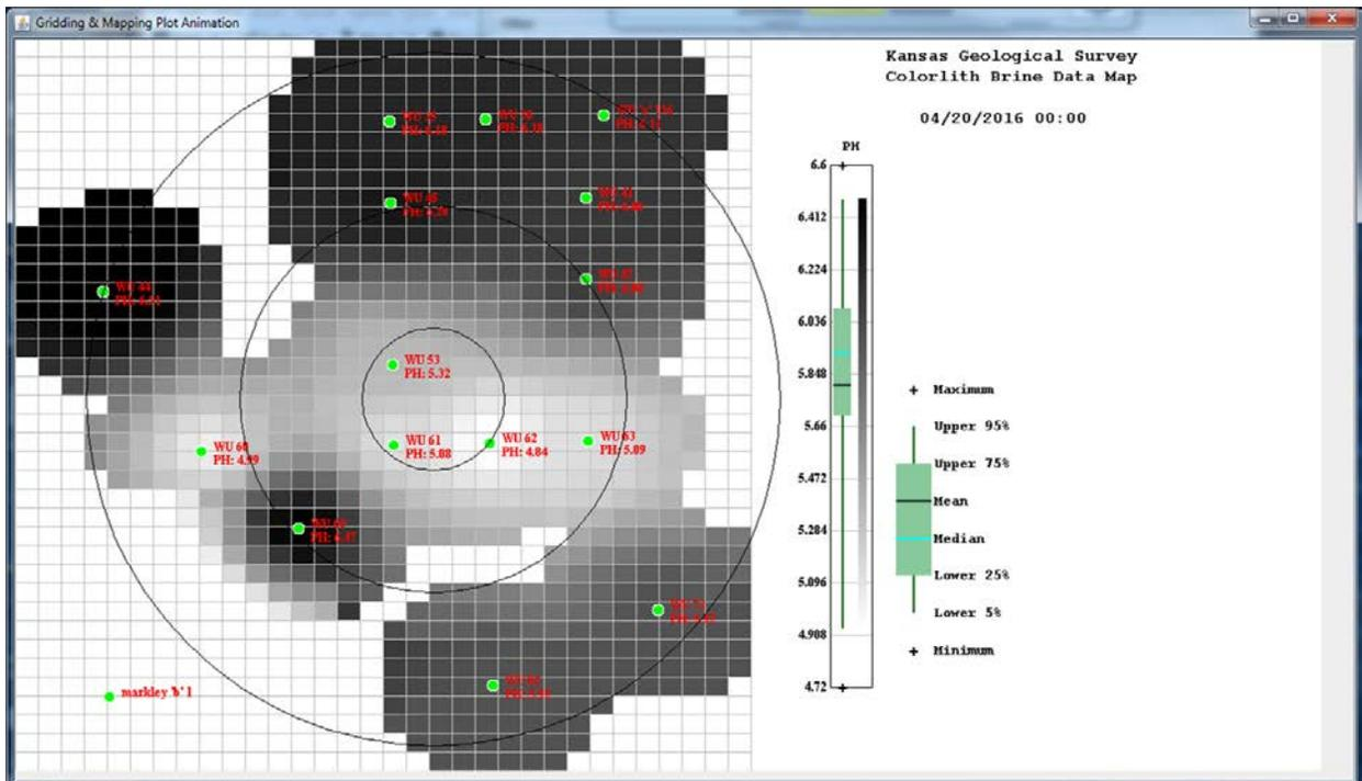
Figure 55. Brine pH taken on 4/20/16 indicates that pH began to fall in well #63 located to the east of the CO<sub>2</sub> injection well.
