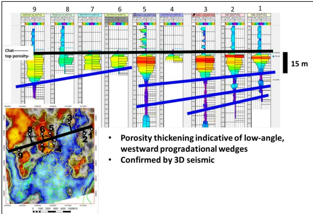
Figure 45. West to east gamma ray and porosity cross section with datum at the top of the Mississippian oil reservoir crossing near the CO<sub>2</sub>-EOR injection well (well #6).
