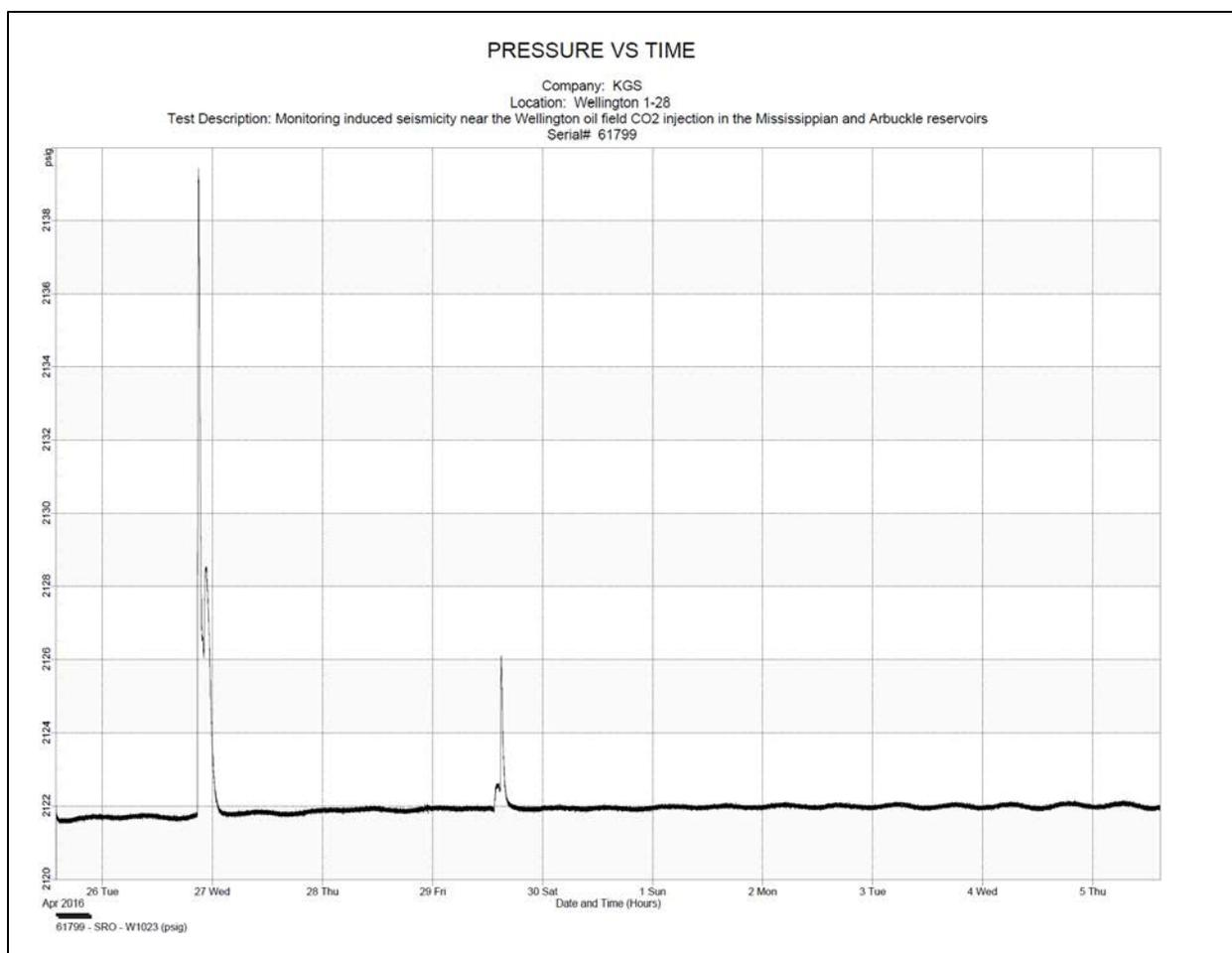
**Figure 42. Initial record of pressure vs. time from April 25 to May 5, 2016 in well #1-28 from lower Arbuckle at 5000 ft depth. Pressures are measured every second and data is transmitted by cable to surface recorder.**
