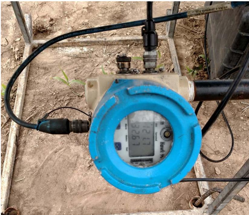
**Figure 40. Pressure readout along with time stamp and delta T.**
