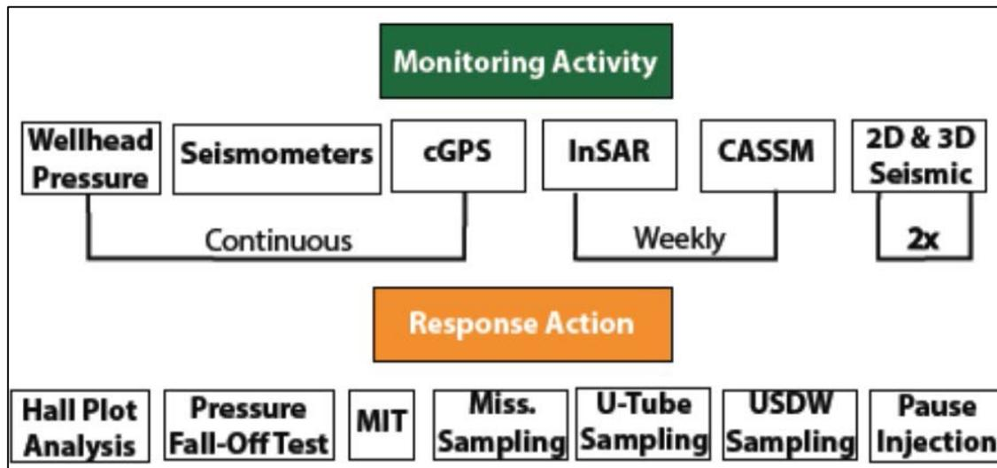
**Figure 37. Partial list of monitoring activities and response action in the Wellington Operating Plan for Safe and Efficient Injection (OPSEI).**
