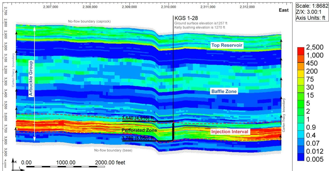
Figure 18. Vertical permeability (mD) distribution within an east-west cross section through the injection well (KGS 1-28), vertical cross-section A-A'. Location of cross section shown in Figure 13.
