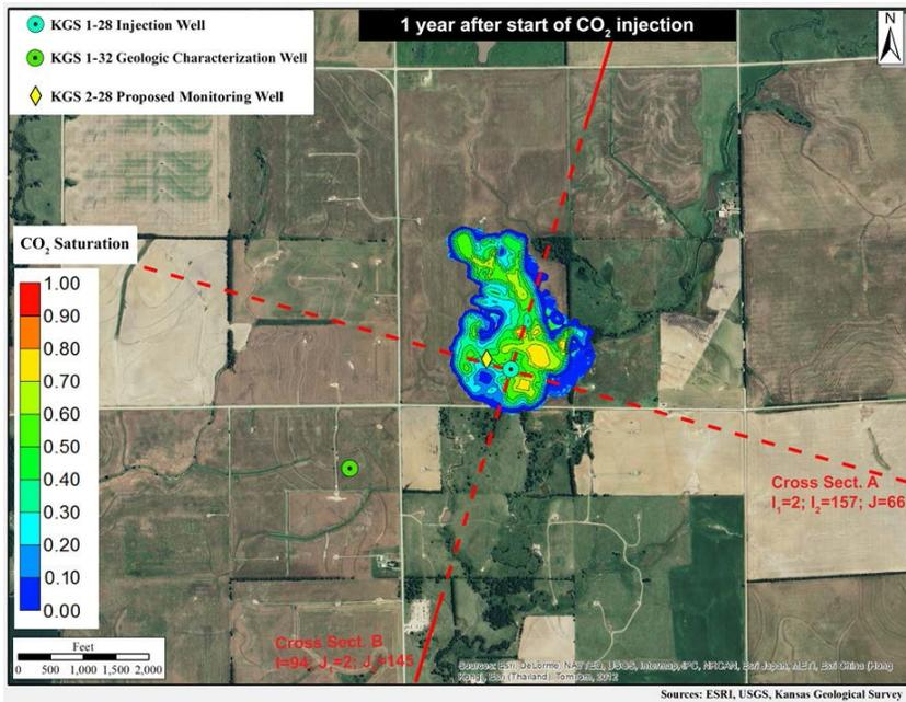
**Figure 19. CO<sub>2</sub> saturation of the CO<sub>2</sub> plume after 1 year of CO<sub>2</sub> injection of 40,000 metric tons.**
