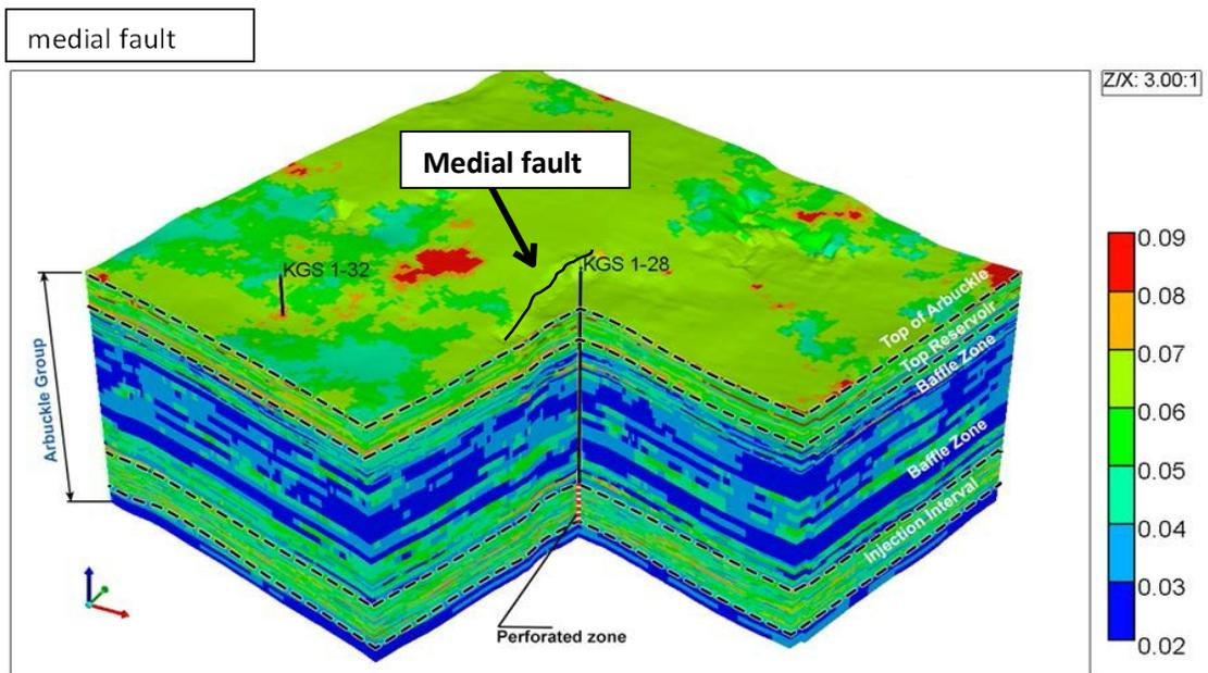
Figure 14. Upscaled porosity distribution in the Arbuckle Group based on the Petrel geomodel. Note the discontinuous relief on the surface of the Arbuckle west of KGS #1-28.
