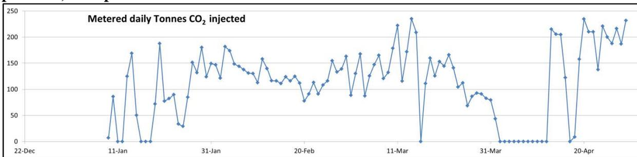
**Figure 51. Daily metered CO<sub>2</sub> injected tonnes/day.**
