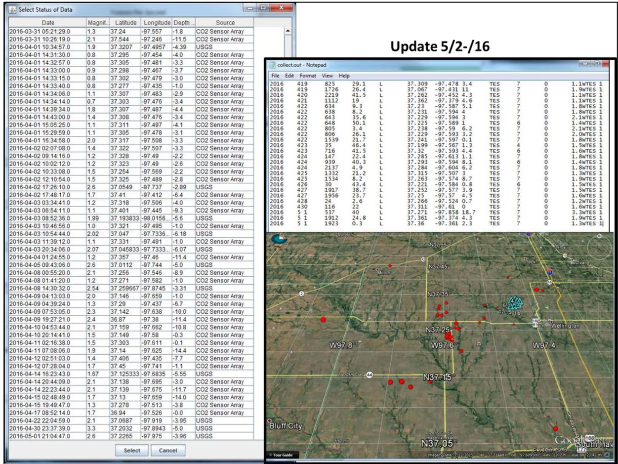
Figure 36. Example of the earthquake catalog of the Wellington Array (aka CO2 Sensor Array). Full catalog is on the left, upper right are the weekly additions, and the Google Earth map on the lower right shows the epicenters of the weekly additions as of 5-1-16.
