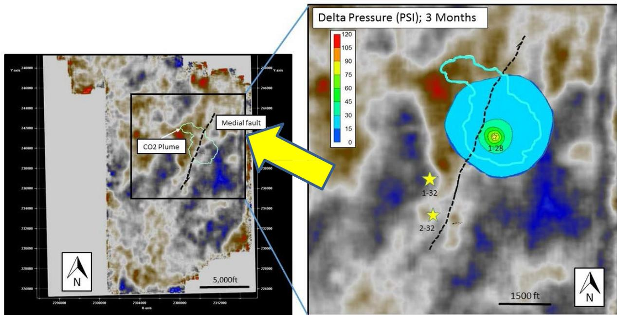
**Figure 20. Delta pore pressure (filled color according to the scale bar) after 9 months injection of 40,000 metric tons of CO<sub>2</sub> in well #1-28. Outline (light blue solid line) of CO<sub>2</sub> saturation after 1 year of CO<sub>2</sub> injection. The medial fault is the black dashed line. Locations of the three KGS wells including the Class II CO<sub>2</sub>-EOR injection well, #2-32, southwest of the Class VI well and near the medial fault shown in the figure.**
