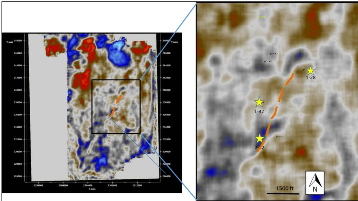
**Figure 9. Seismic amplitude slice near the top of the Mississippian at around 3750 feet. The location of fault is the SW-NE curvilinear that delimits the discontinuous fault. The NW termination of the fault at the top of the Mississippian is due west of the Class VI injection well, #1-28. The southern termination is just southeast of the operating Class II CO<sub>2</sub>-EOR well, #2-32. (Courtesy of D. Schwab, KGS/KU).**
