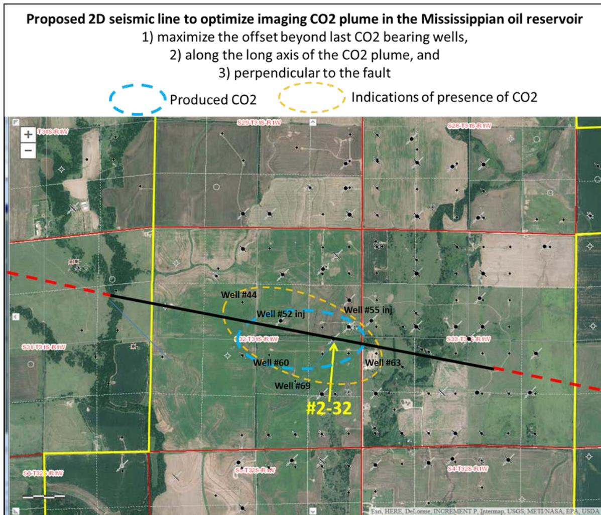
**Figure 68.** A repeat 2D seismic survey is being considered. The final processed line is shown as the black solid line. In order to get the long offsets needed for AVO the actual survey footprint (i.e. locations occupied by the vibroseis trucks on land) will have to extend 4,000 feet longer on both ends of the black line, approximated by the red dashed line segments.
