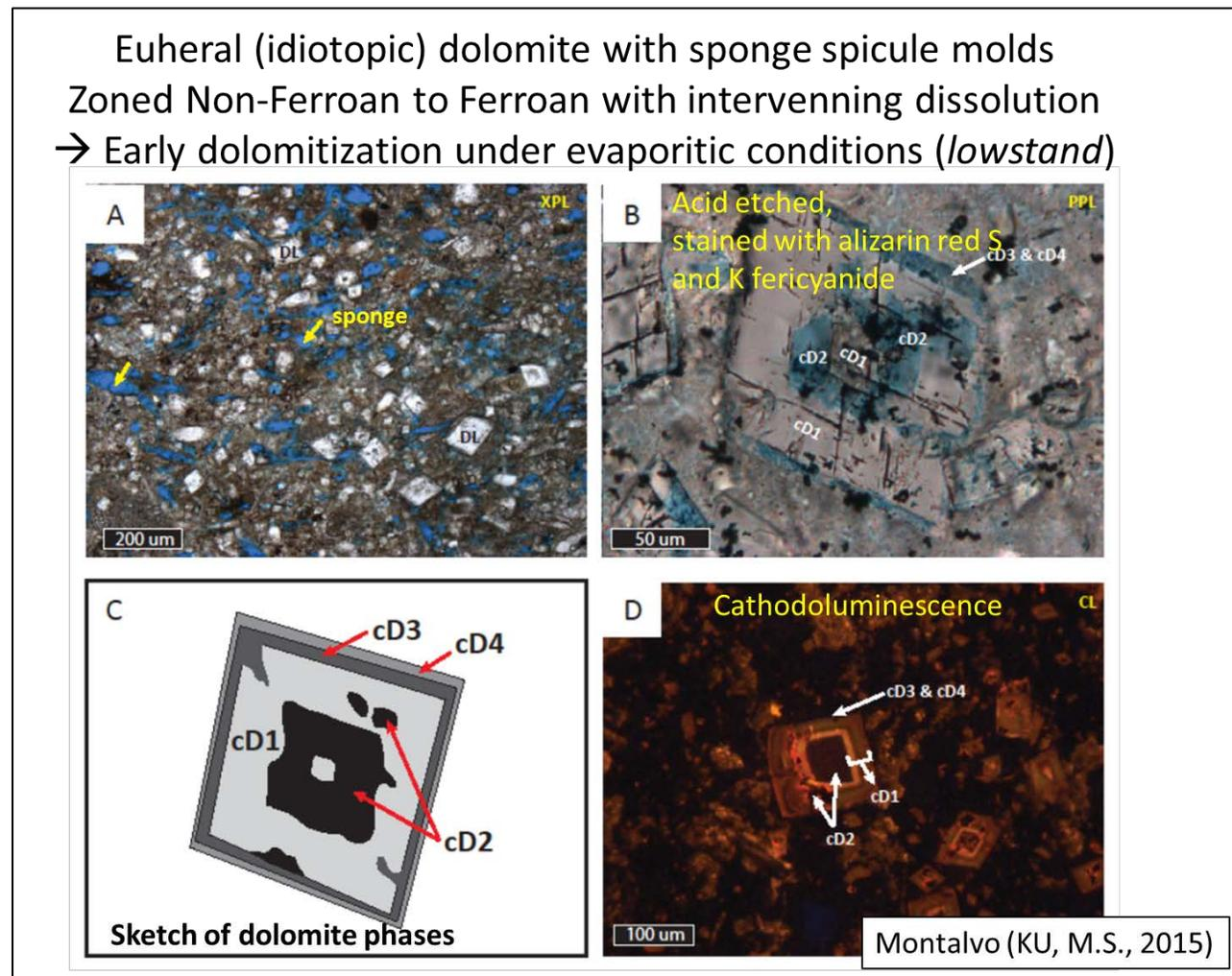
**Figure 63.** Thin section petrography, staining, and cathodoluminescence were used to characterize the Mississippian dolomite.
