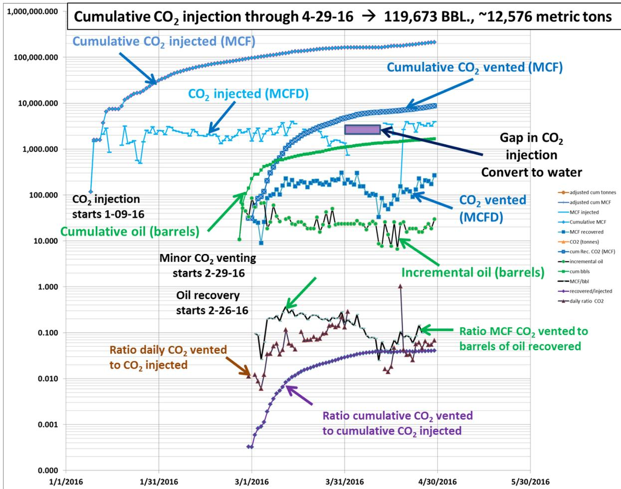
**Figure 48. Combined semi-log plot of the CO<sub>2</sub> injected and recovered and the oil produced from the Wellington CO<sub>2</sub>-EOR through the end of April, 2016**
