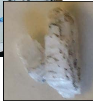
Figure 5. Representative sample below 14 ft. consisting of dark gray silty clay to claystone containing scattered gypsum as noted in the inset photo.
