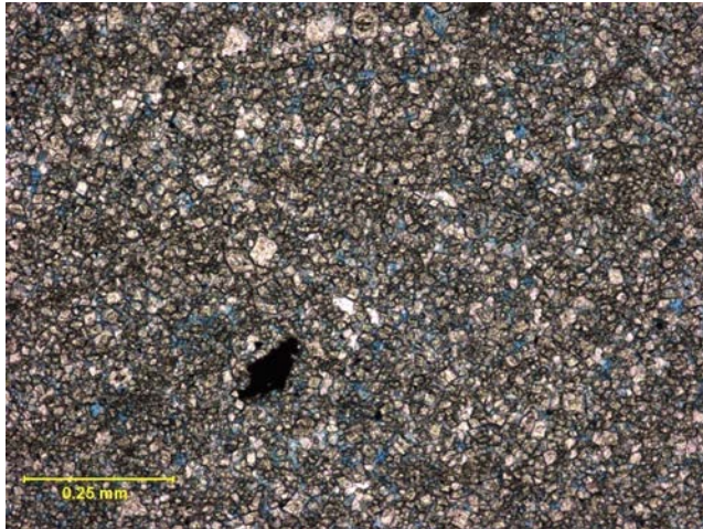
Figure 9. Thin section photomicrograph with blue epoxy impregnation of Mississippian oil reservoir from Wellington KGS #1-32 borehole. Reservoir is a finely crystalline dolomite with mottling of silica cement and replacement of the dolomite.
