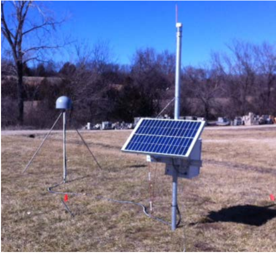
Figure 12. CGPS and seismometer training station installed at KU campus for instruction and testing of equipment before deploying to the field.
