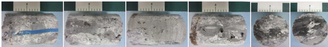
Figure 46. Properties of core plugs taken to LLNL lab for in situ studies of reactions with injection of CO 2 saturated brine.
