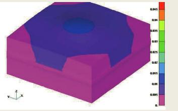
Simulated vertical displacement (in meter) after 3 years of CO2 injection (top) without and (below) with a permeable fault intersecting the caprock.
