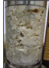
Core plug 31-19 between platens at the NETL before being wrapped for CO 2 flow
