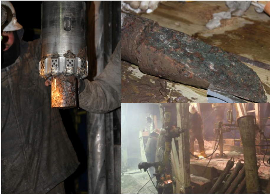
Figure 3. Last core run (#42) into granite basement.
