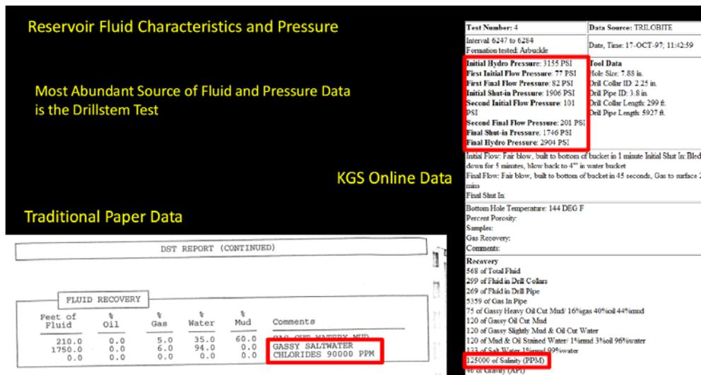
Figure 8. Paper and electronic records of DST measurements.
