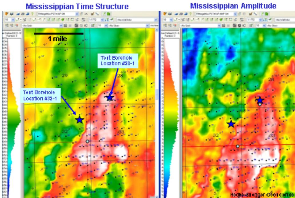
Figure 39. Test borehole #1-32 is located off the highest structure on the top of the Mississippian limestone, the oil reservoir for Wellington Field. Seismic maps including Mississippian time and converted depth structure indicate highs in warm colors and lows in cooler colors.
