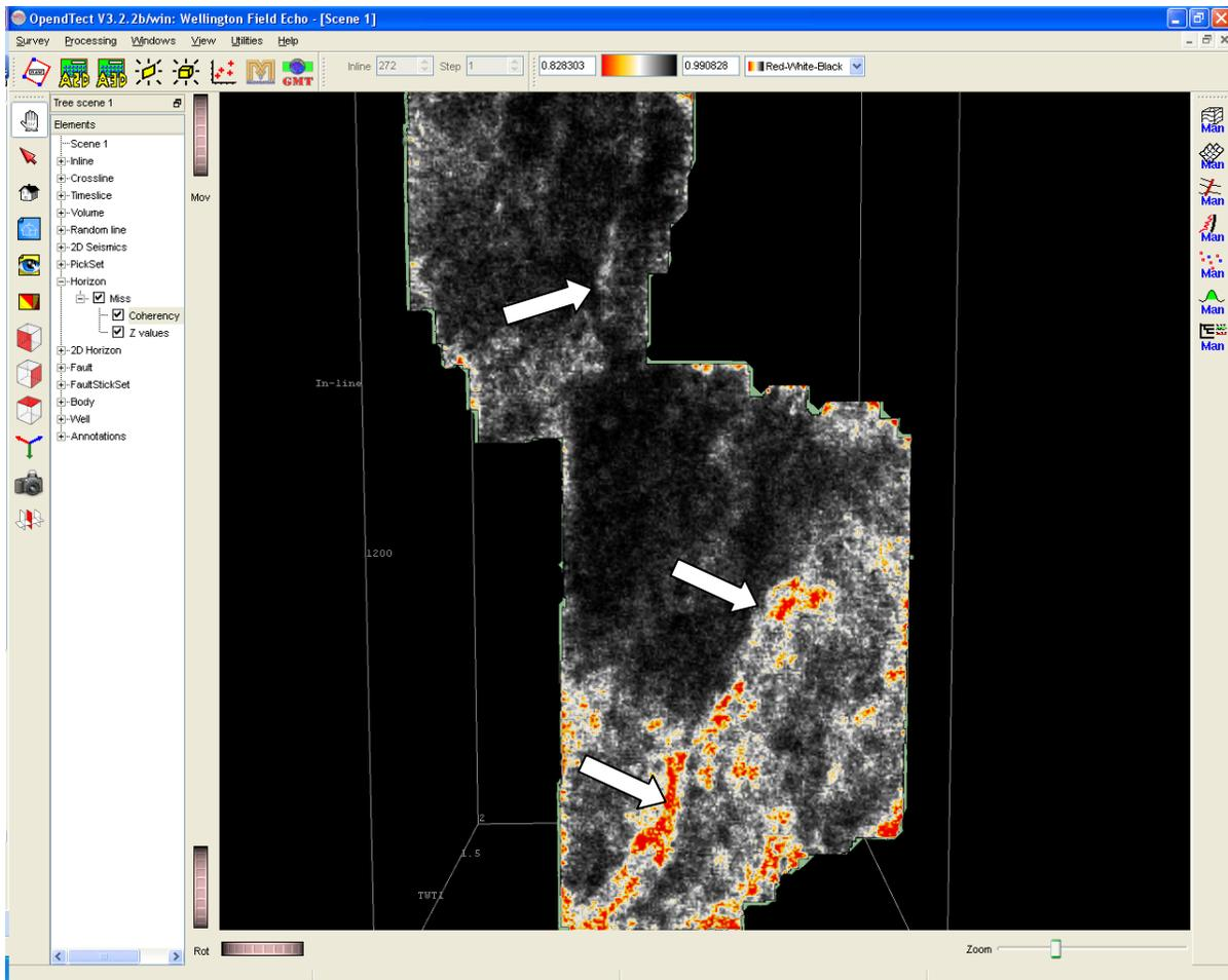
Figure 23. Mississippian horizon (Echo processing) with coherency extracted along the top of it.
