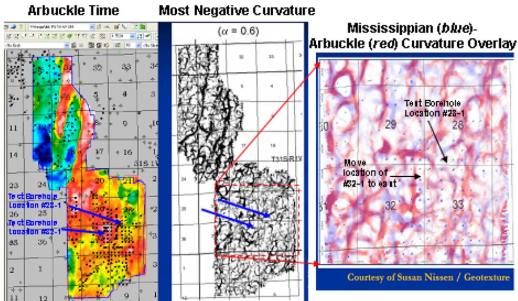
Figure 41. (Top) Volumetric coherency and curvature were used to help refine the location of the tests boreholes. (Bottom) Arbuckle time, most negative curvature for Arbuckle and combined curvature of Mississippian (blue) and Arbuckle (red) showing locations of new test boreholes.
