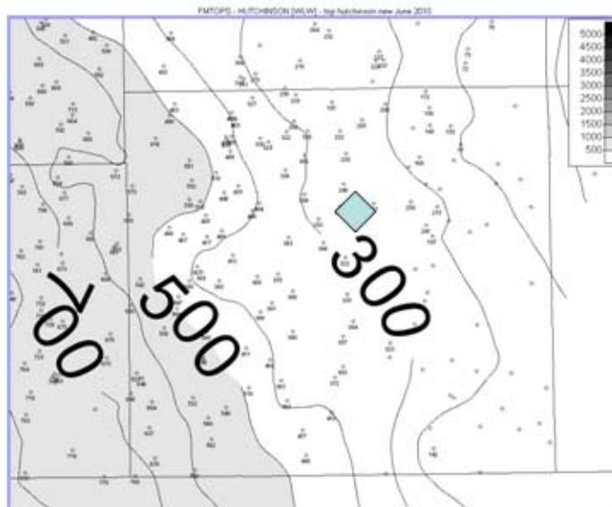
Measured depth to top of salt in Wellington Co.
