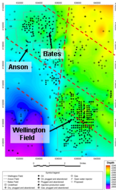
Configuration on top of the Mississippian (regional unconformity) in Wellington and Bates Field area. Fields are part of a subcrop play with the chat reservoir preserved in what appears to be structural blocks bounded by NE- and NW-trending lineaments. Warmer colors represent higher elevation.
