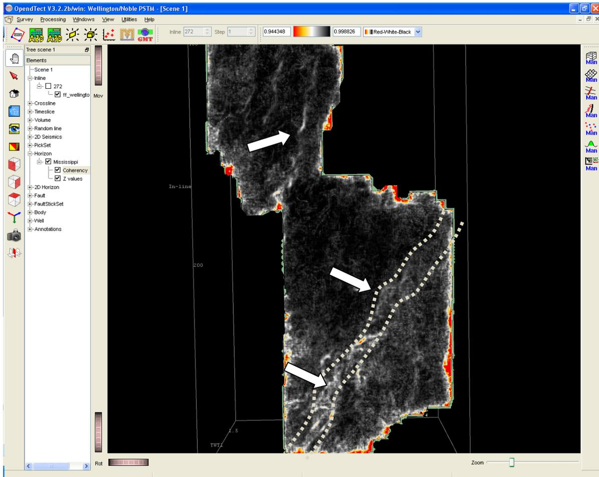
Figure 22. Mississippian horizon (Fairfield processing) with coherency attribute extracted along the top of it.
