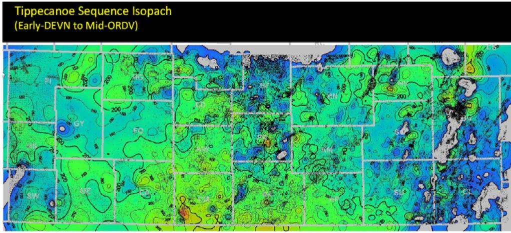
Figure 57. Tippecanoe cratonic sequence of interval between Kaskaskia cratonic sequence (Figure 56) and the Arbuckle including the Simpson Group. Thickening is in south central region bounded by distinct edges trending northwest and northeasterly.
