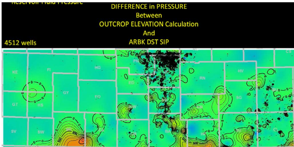
Figure 12. Difference between the pressures estimated from surface exposure of Arbuckle and the Arbuckle shut-in pressures suggest that the subsurface pressure in the Arbuckle is tied to the outcrop.
