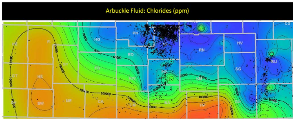
Figure 14. Chloride concentration determined from fluid recovery from Arbuckle DSTs. Chloride concentration increases with depth.
