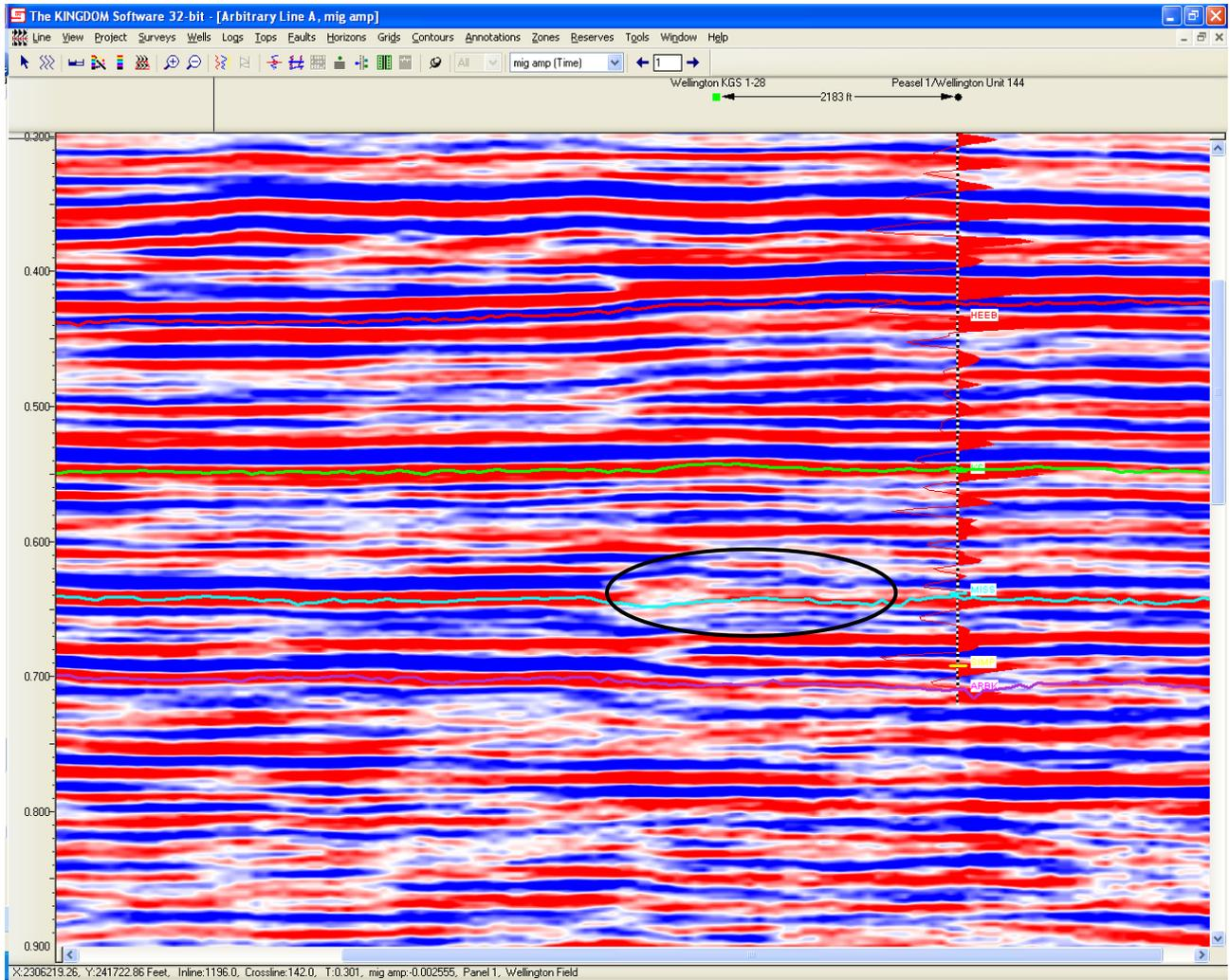
Figure 19. Cross-section A showing the amplitude anomaly circled in black.
