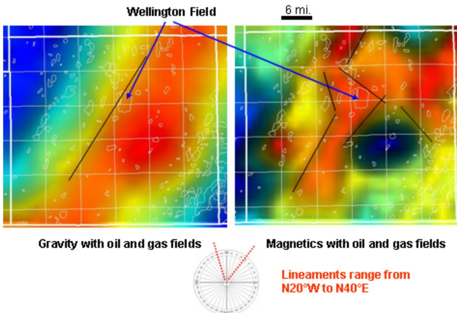
Figure 30. For comparison, entire Sumner County is shown with – **(Left side)** Bouguer anomaly gridded with a two-pass, 8-directional gridding algorithm. A second-order polynomial surface was calculated to remove a regional westward decrease in gravity values caused in part by thickening of the crust resulting in second-order residual grid as shown. **(Right side)** Total
