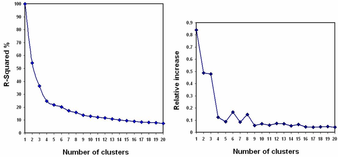
Figure 7. Scree and slope plots of clustered zonation of log-processed volumes of dolomite, chert, and calcite in the Mississippian section.
