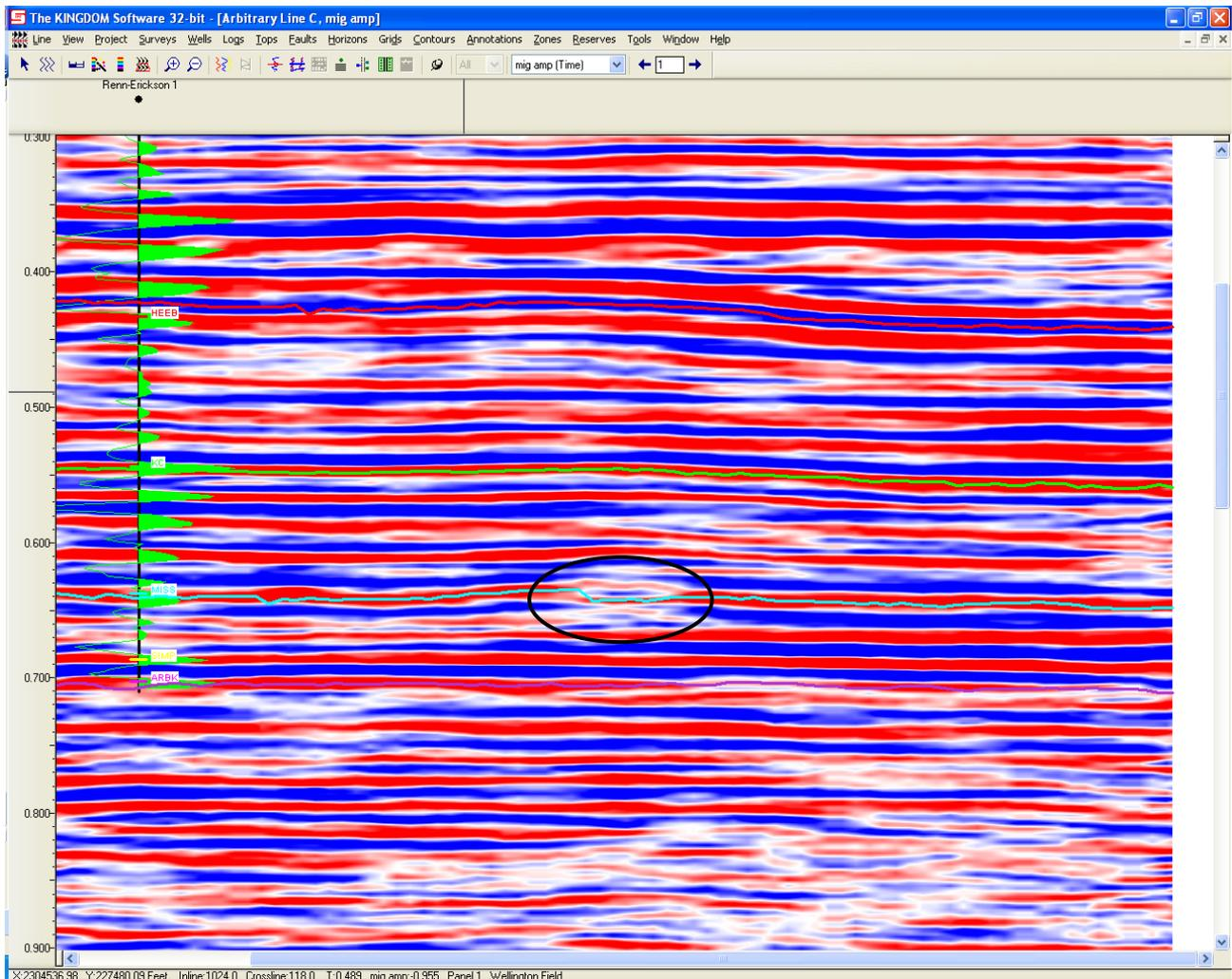
Figure 21. Cross-Section C showing the amplitude anomaly circled in black.
