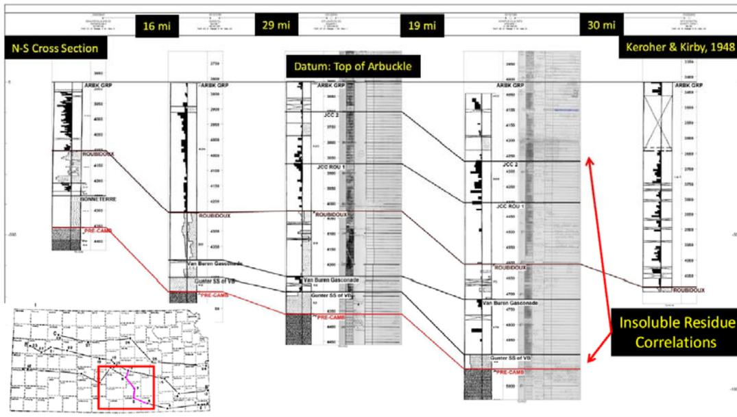
Figure 49. Example of related insoluble residue (black and white depth plot) with sample log descriptions. Petrophysical logs can similarly be compared via curves and lithologic interpretation.
