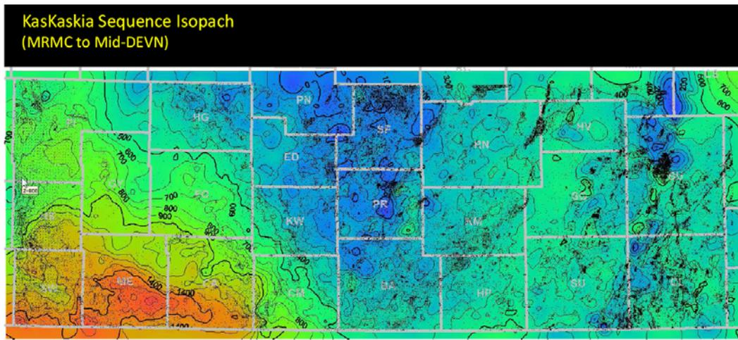
Figure 56. Isopach of a major cratonic depositional sequence that includes the Mississippian to Mid-Devonian, an interval overlying the Arbuckle. Thickness greatly increases in area of Western Annex. Blue area of thinning primarily reflects post Mississippian, pre-Pennsylvanian erosion.
