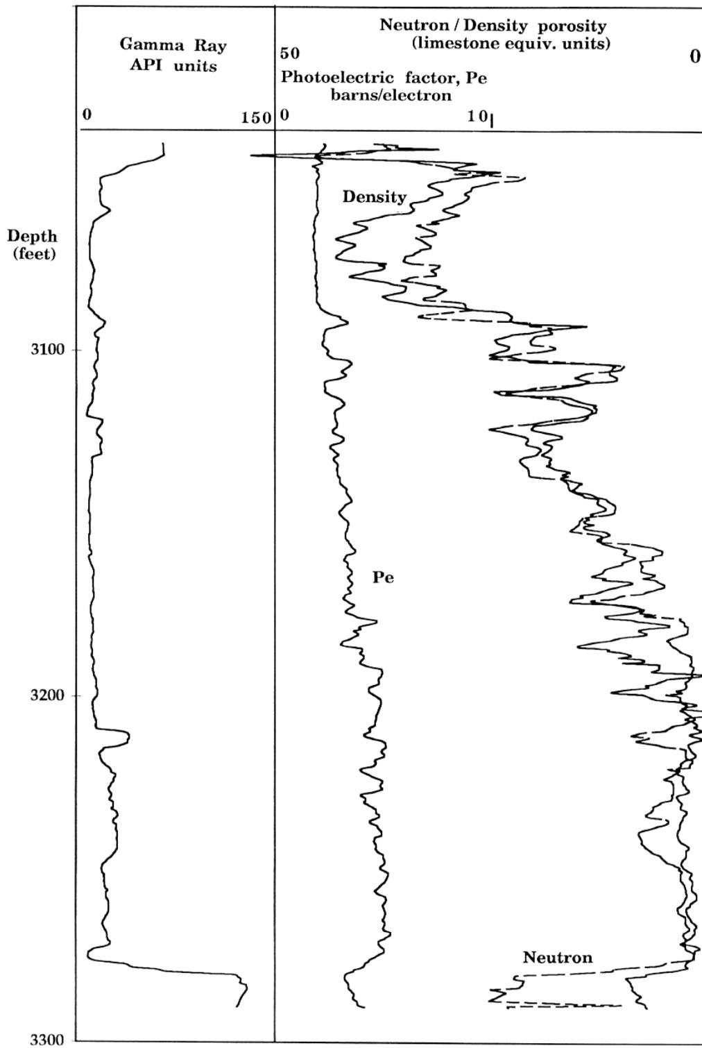
Figure 6. Gamma-ray, neutron, density and photoelectric factor logs of a Mississippian section in a case-study well.
