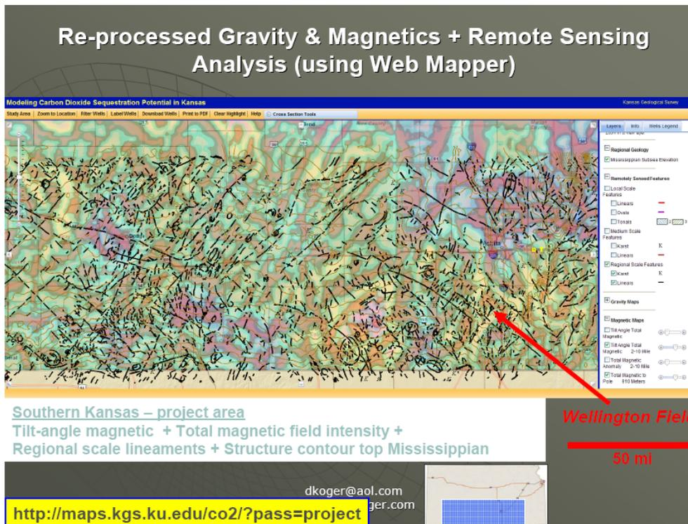
Figure 16. Combined lineaments from remote sensing analysis (dark lines) and reprocessed magnetic including tilt angle (colored linear trends) and total magnetic field intensity (broad areas of tonal color change). Note regional scale.
