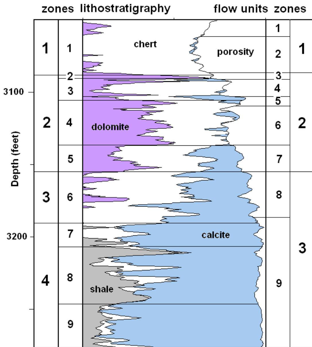
Figure 8. Comparison of nine lithostratigraphic units with nine flow units in Mississippian section estimated from depth-constrained clustering
