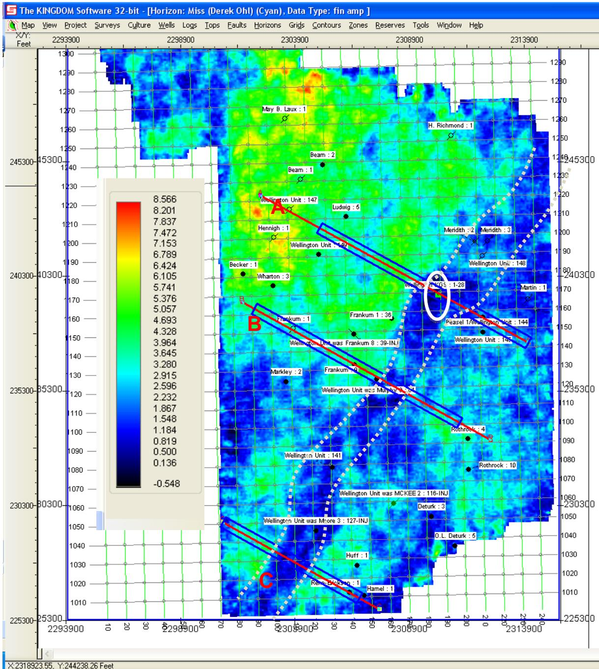
Figure 18. Mississippian horizon (amplitude from Echo) shows the location of three cross-sections running through the amplitude anomaly. The white circle along cross-section A shows the location of the new well that is being drilled.
