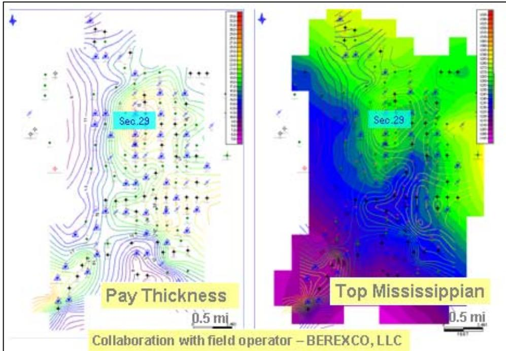
Figure 32. Initial mapping of pay thickness and structure of Wellington Field. Left – pay thickness with warmer contours equal to thicker pay. Right – Structure map with higher elevation depicted by warmer colors.
