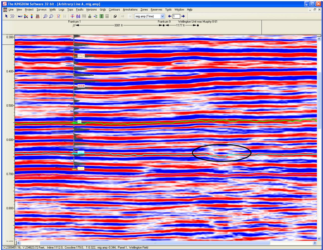
Figure 20. Cross-section B showing the amplitude anomaly circled in black.
