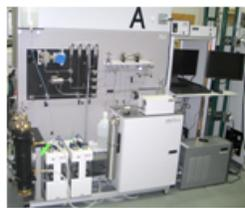
Flow through to examine flow-through fractured seal materials
