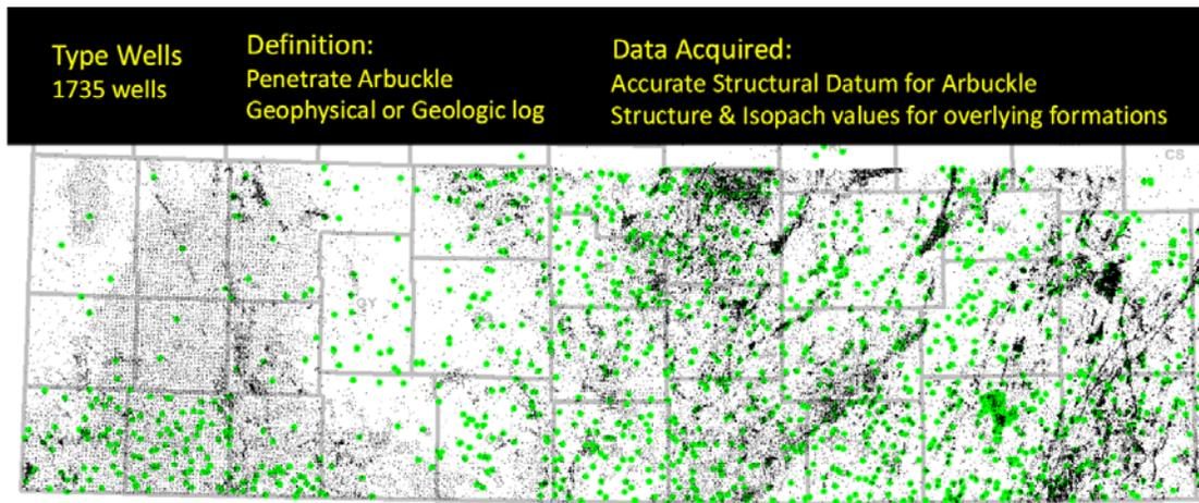
Figure 46. Type wells (as defined in this figure heading) shown in study area by green dots. This subset of wells serve as keys for correlation and provide properties for the strata being modeled as do the supertype wells that have even more complete information. Many of these wells will have wireline logs and sample descriptions digitized to LAS format.
