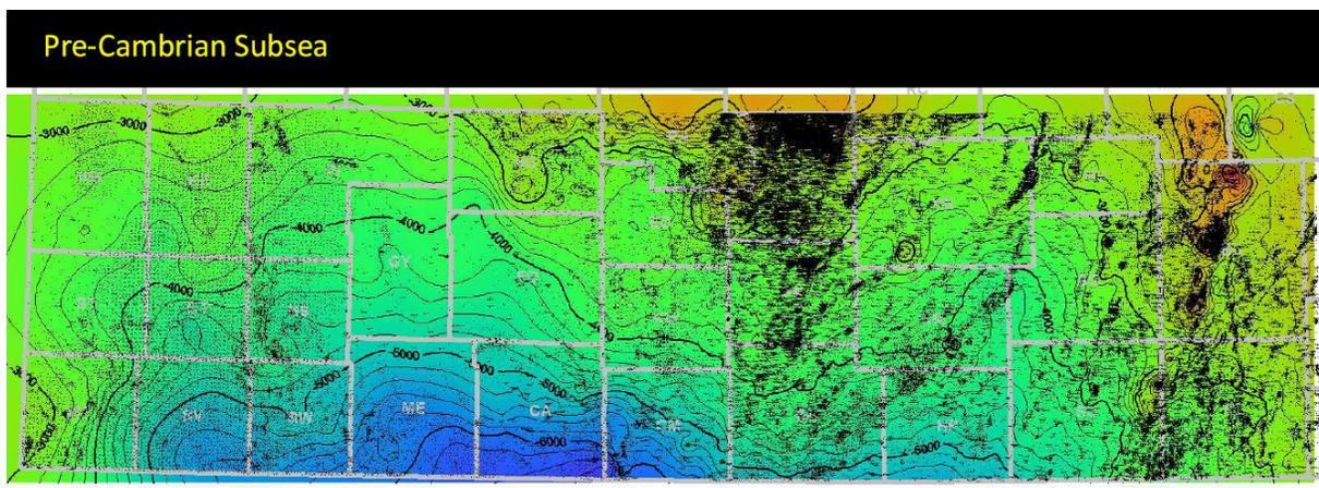
Figure 51. Structure map of Precambrian surface now delimited Hugoton Embayment in western area, Pratt Anticline in central, Sedgwick Basin in east central bordered by Nemaha Uplift on the east. Blue color indicates greater depths and orange is higher elevation.
