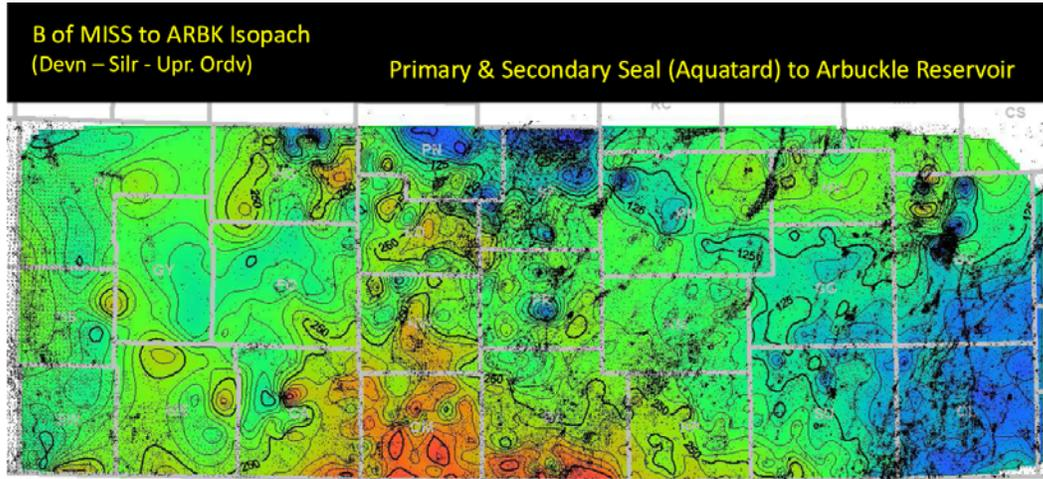
Figure 55. Base of Mississippian to Arbuckle isopach showing areas of thickening in orange in south-central mapped area. Interval contains the primary and secondary caprocks of the Chattanooga Shale and shales in the Simpson Group. Eastern thin is related to what was an active Chautauqua Arch and related erosion during this period of deposition.
