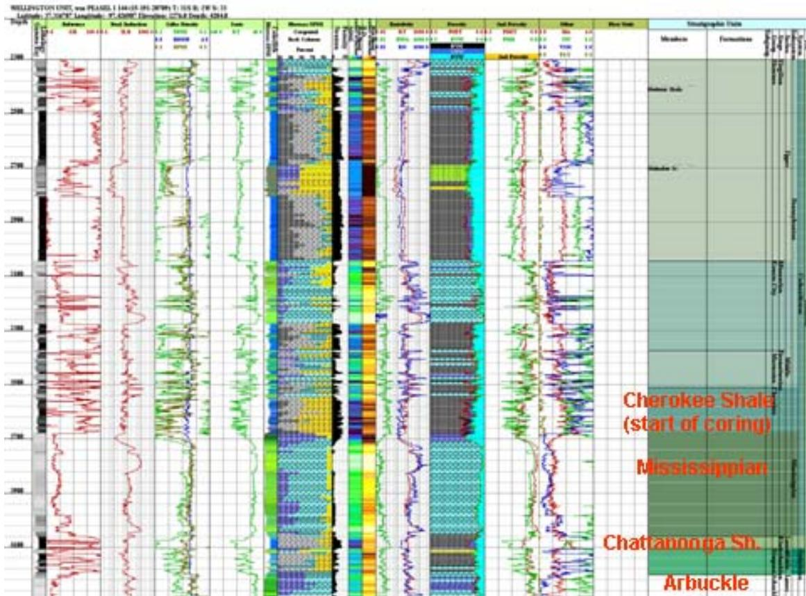
Figure 42. Peasel Wellington Unit #144 showing lithologies of stratigraphic section above the Arbuckle and location where coring will commence.
