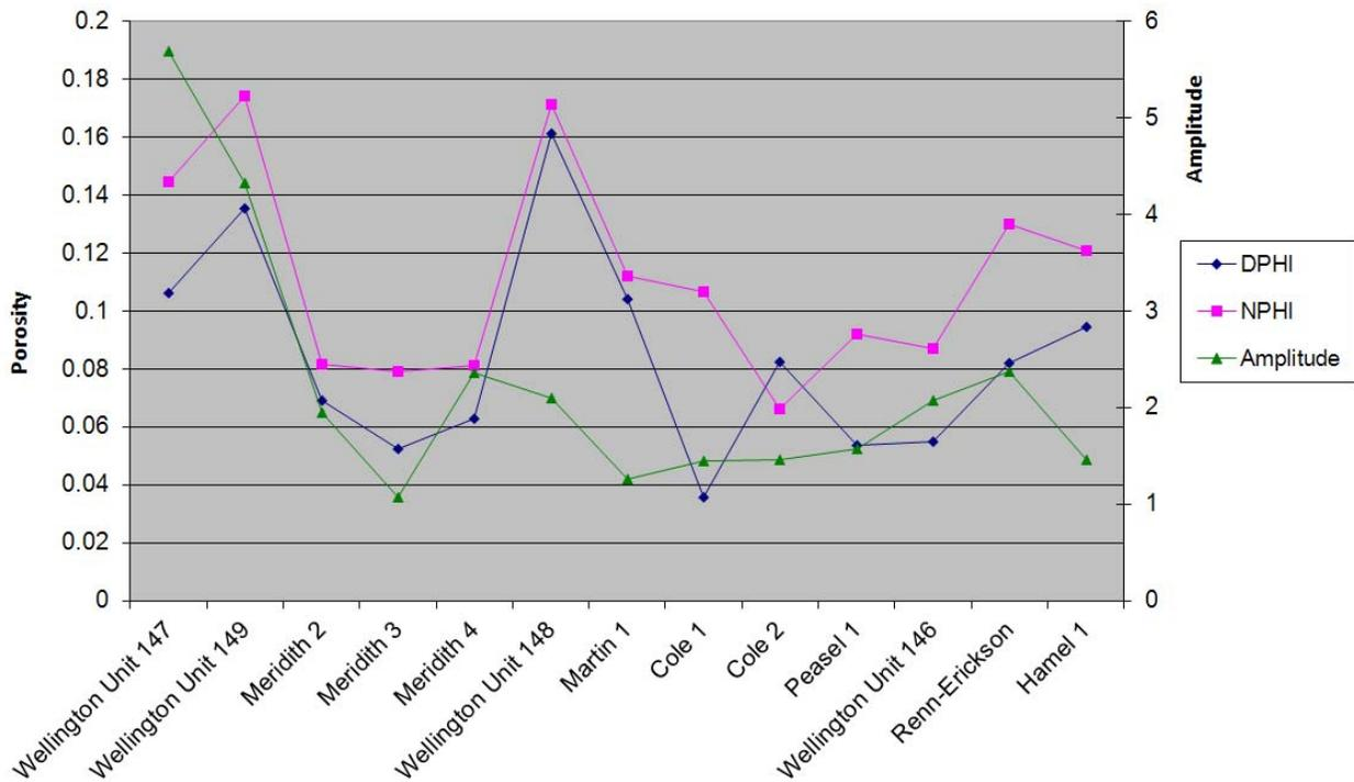
Figure 24. Porosity prediction from amplitude compared to neutron-density porosity logs in Wellington Field.
