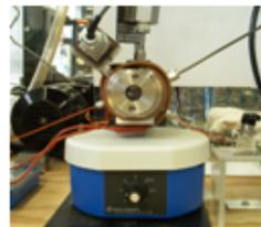
Stainless steel view cell (5 mL) for batch/semi-batch studies
