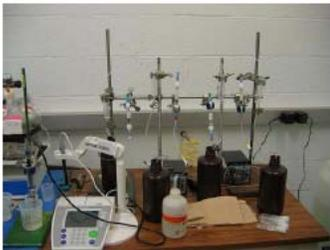
Flow Cell set up at GCSU with crushed Basalt
