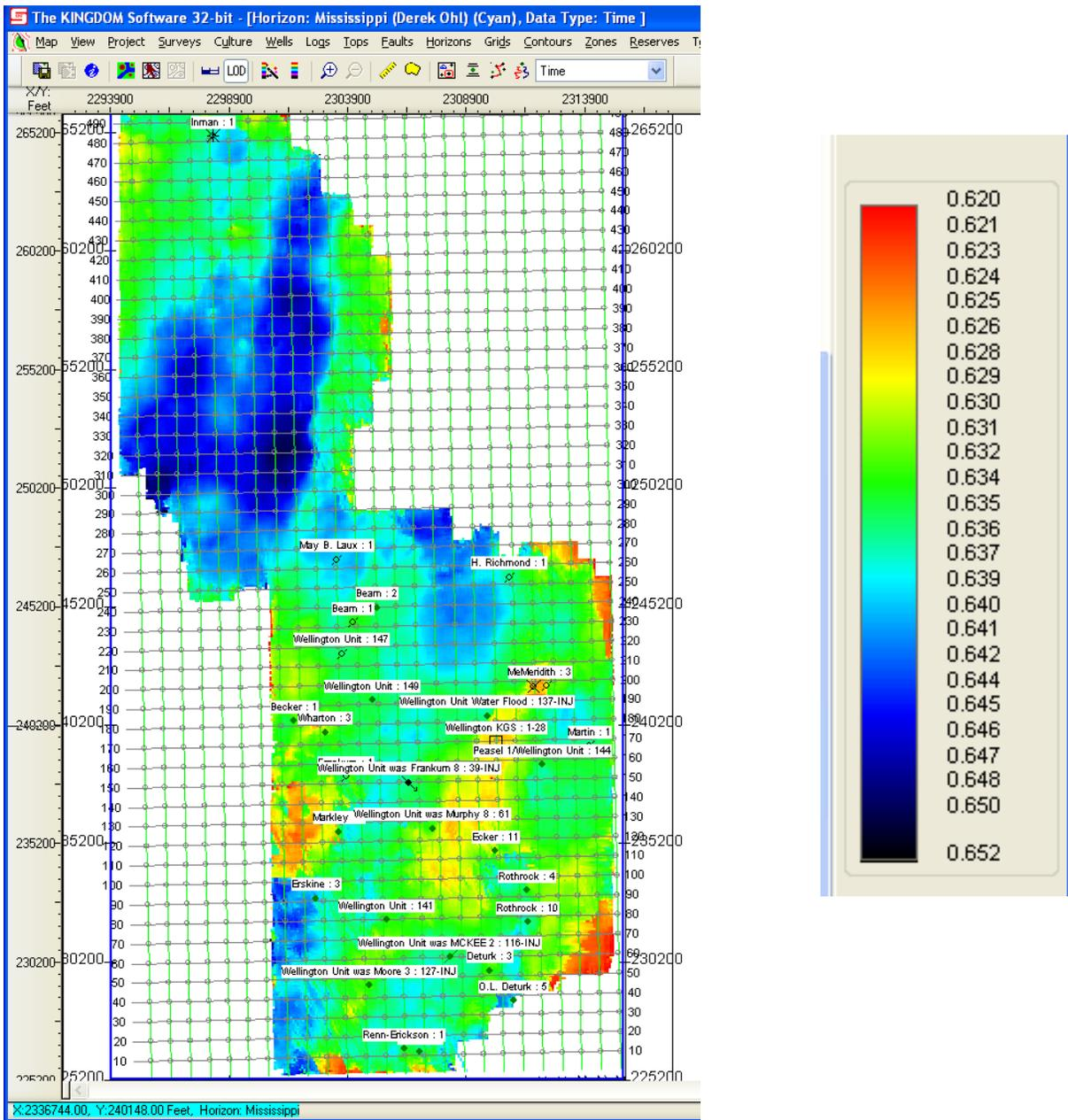
Figure 17. Structural time map with no evident and coherent anomaly in match to the coherency and amplitude anomalies shown below; below-temporal resolution faulting/folding will not cause temporal anomaly.
