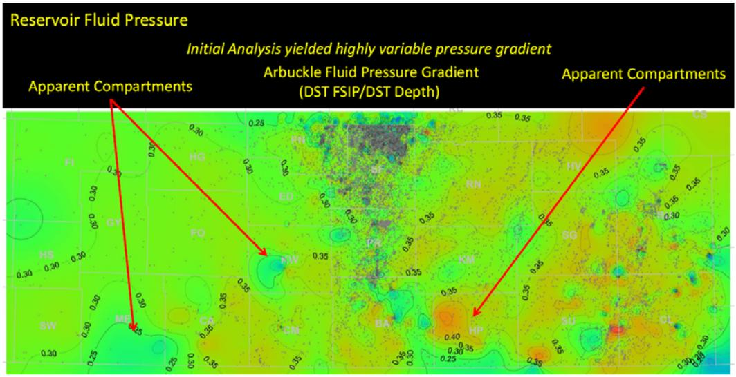
Figure 10. DST final shut-in pressure divided by depth of DST measurement showing apparent anomalies.
