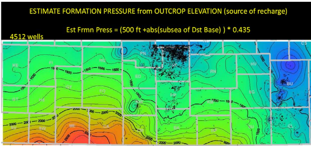
Figure 11. Estimated formation pressures in Arbuckle based on minimum elevation of surface exposures of the Arbuckle Group in Missouri. Hydrostatic head estimated here is proportional to the depth of the DST below the water level defined by elevation of free water level at surface exposure.
