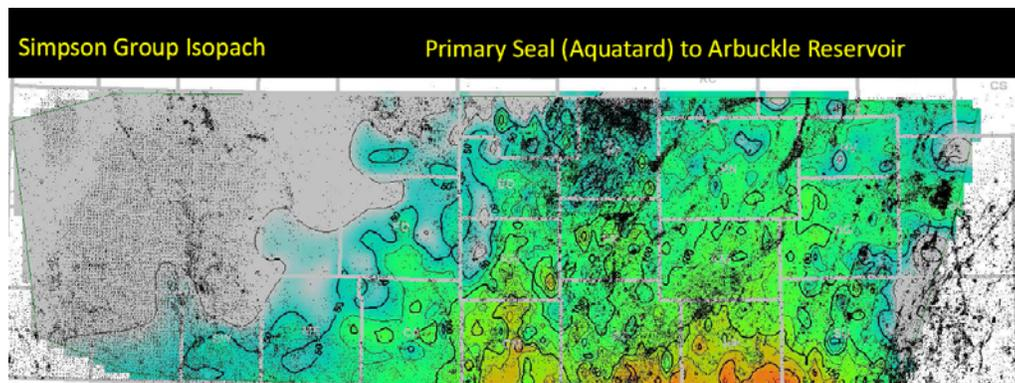
Figure 54. Simpson Group isopach. Shale and sandstone strata overlie the Arbuckle in the eastern 2/3<sup>rd</sup> of the area.
