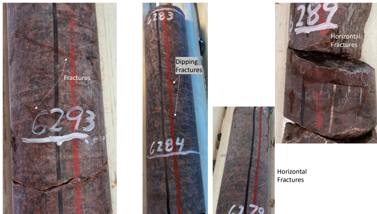
Figure 70: Core photos showing both horizontal and angled fractures that cross-cut the whole cores.
