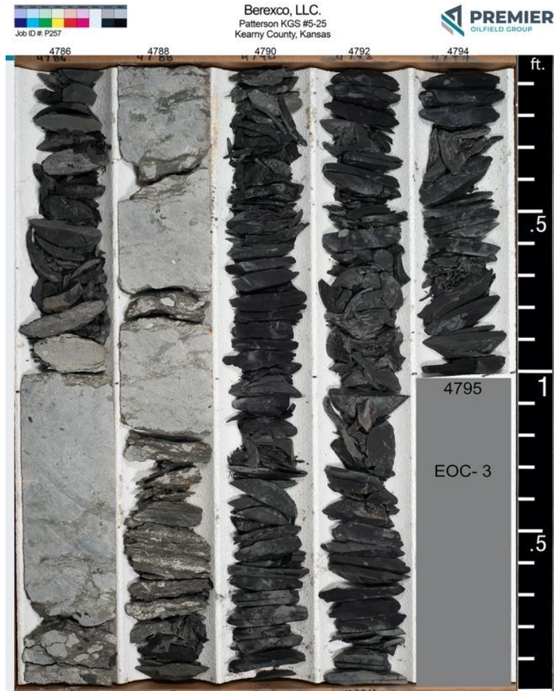
Figure 37: Representative core from the Morrow Shale interval showing black shale with calcite-cemented interval from 4787-4789.5 ft.
