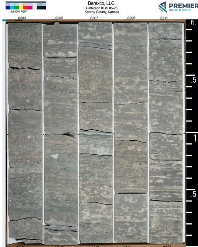
Figure 63: Representative core from the interval of the Bonneterre from 6200-6214 ft showing clotted algal boundstone texture, glauconite, and shale interbed.
