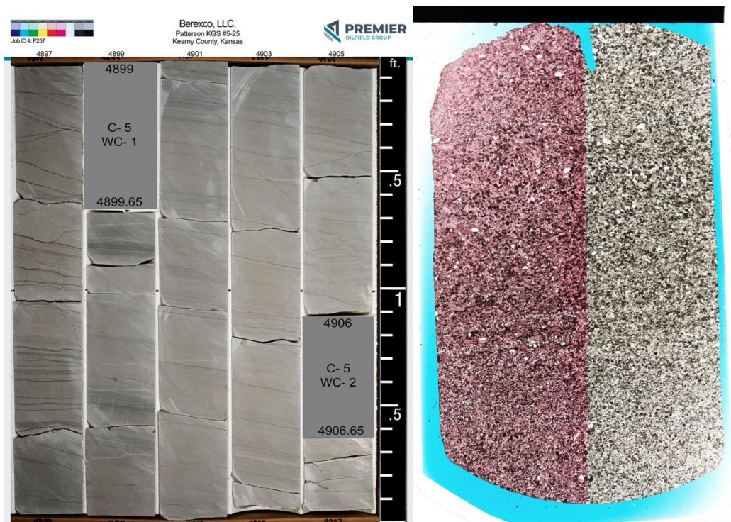
Figure 38: A) Representative core from the Meramec interval showing crossbedded skeletal grainstone. B) Representative thin section image of Meramec from 4890.00 ft.
