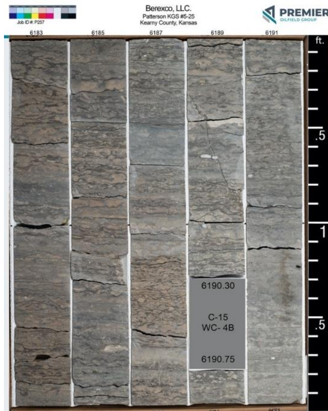
Figure 62: Representative core from the interval of the Bonneterre from 6170-6200 ft showing clotted algal boundstone texture.
