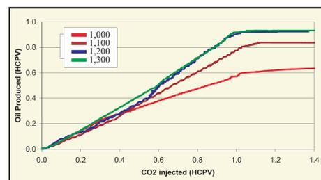
Oil recovery results in slim-tube experiment with CO<sub>2</sub> displacing Indiana oil sample at 101°F.
