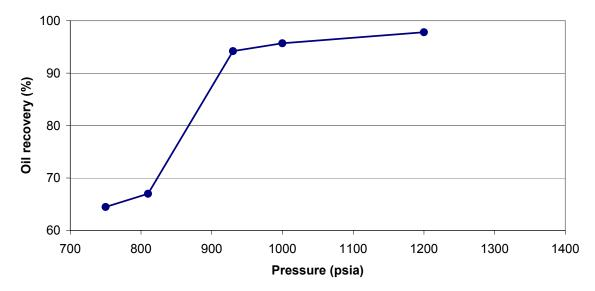
**Figure A4** - Oil recovery (at 1.2 HCPV injection of  $CO_2$ ) as a function of pressure for Kentucky oil sample #22 at 79 °F.
