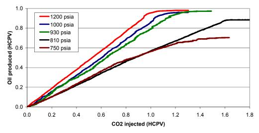
Figure A3 - Oil recovery results in slim-tube experiment with  $CO_2$  displacing Kentucky oil sample #22 at 79 °F.
