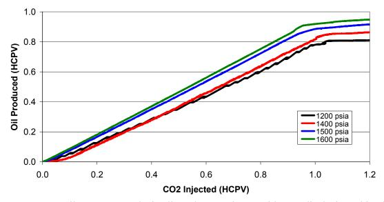
**Figure A7 -** Oil recovery results in slim-tube experiment with CO<sub>2</sub> displacing Ohio oil sample at 107 °F.
