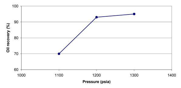
Figure A6 - Oil recovery (at 1.2 HCPV injection of  $CO_2$ ) as a function of pressure for Illinois oil sample at 111 °F.
