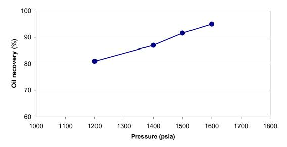
**Figure A8** - Oil recovery (at 1.2 HCPV injection of  $CO_2$ ) as a function of pressure for Ohio oil sample at 107 °F.
