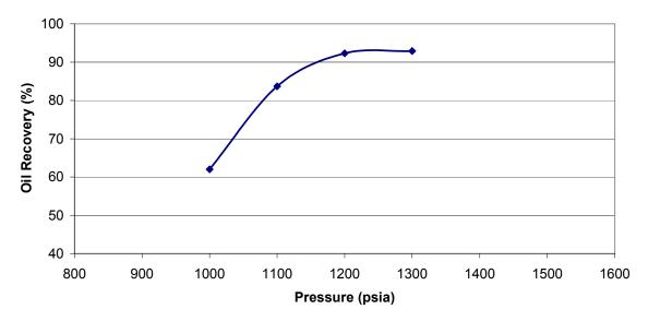
**Figure A2** - Ultimate oil recovery as a function of pressure for Indiana oil sample at 101 °F.
