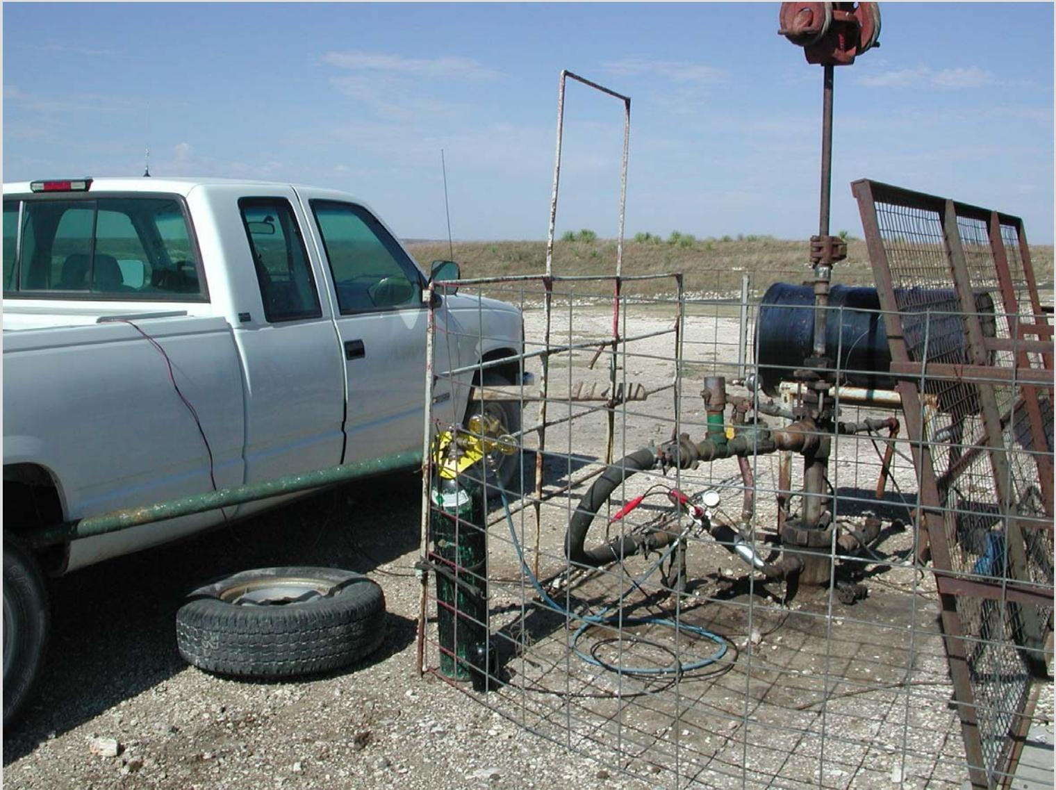
Build-up Test on Vess Oil's McCord A #4
