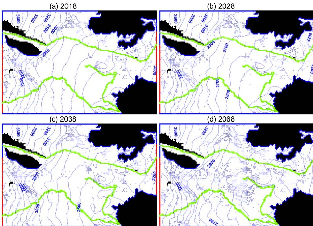
**Figure 55.** Distribution of wells that have a pumping rate reduction by more than 75% at different years in scenario 3b: (a) 2018, (b) 2028, (c) 2038, and (d) 2068.
