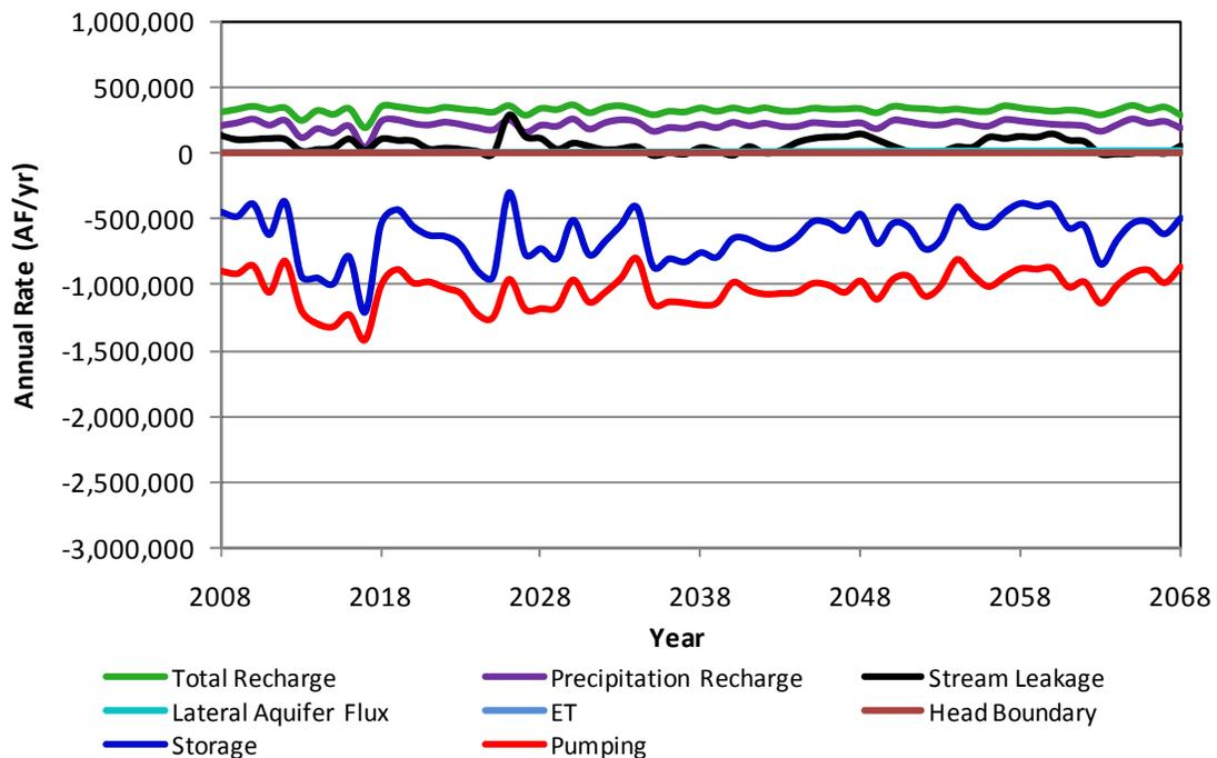
**Figure 49.** Components of the simulated aquifer budget for the GMD3 area in scenario 3a.
