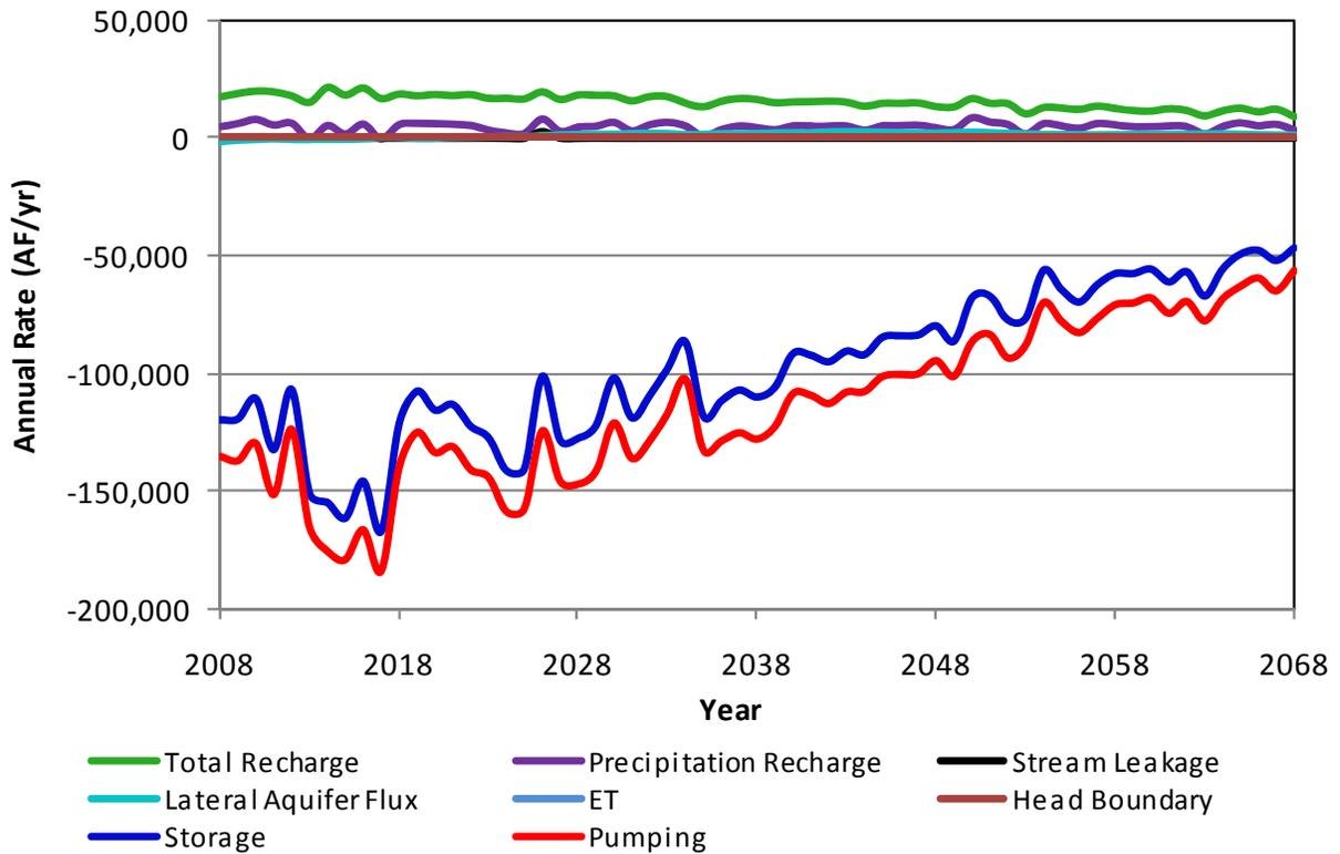
**Figure A17.** Components of the simulated aquifer budget for Grant County in scenario 1b.
