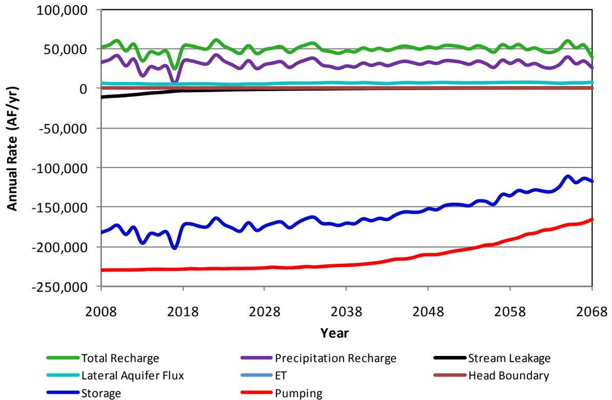
**Figure A47.** Components of the simulated aquifer budget for Seward County in scenario 3b.
