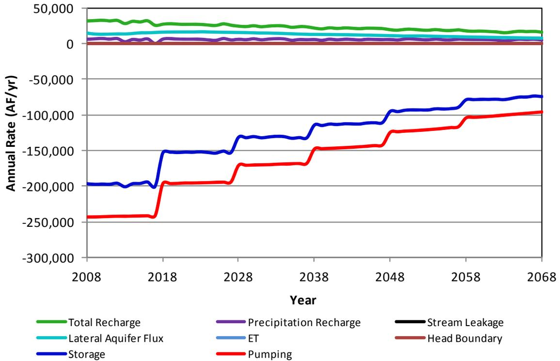
**Figure A56.** Components of the simulated aquifer budget for Haskell County in scenario 3c.
