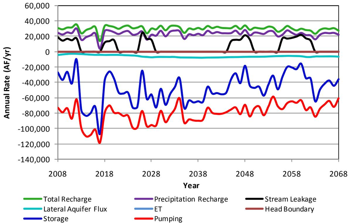
**Figure A34.** Components of the simulated aquifer budget for Gray County in scenario 3a.
