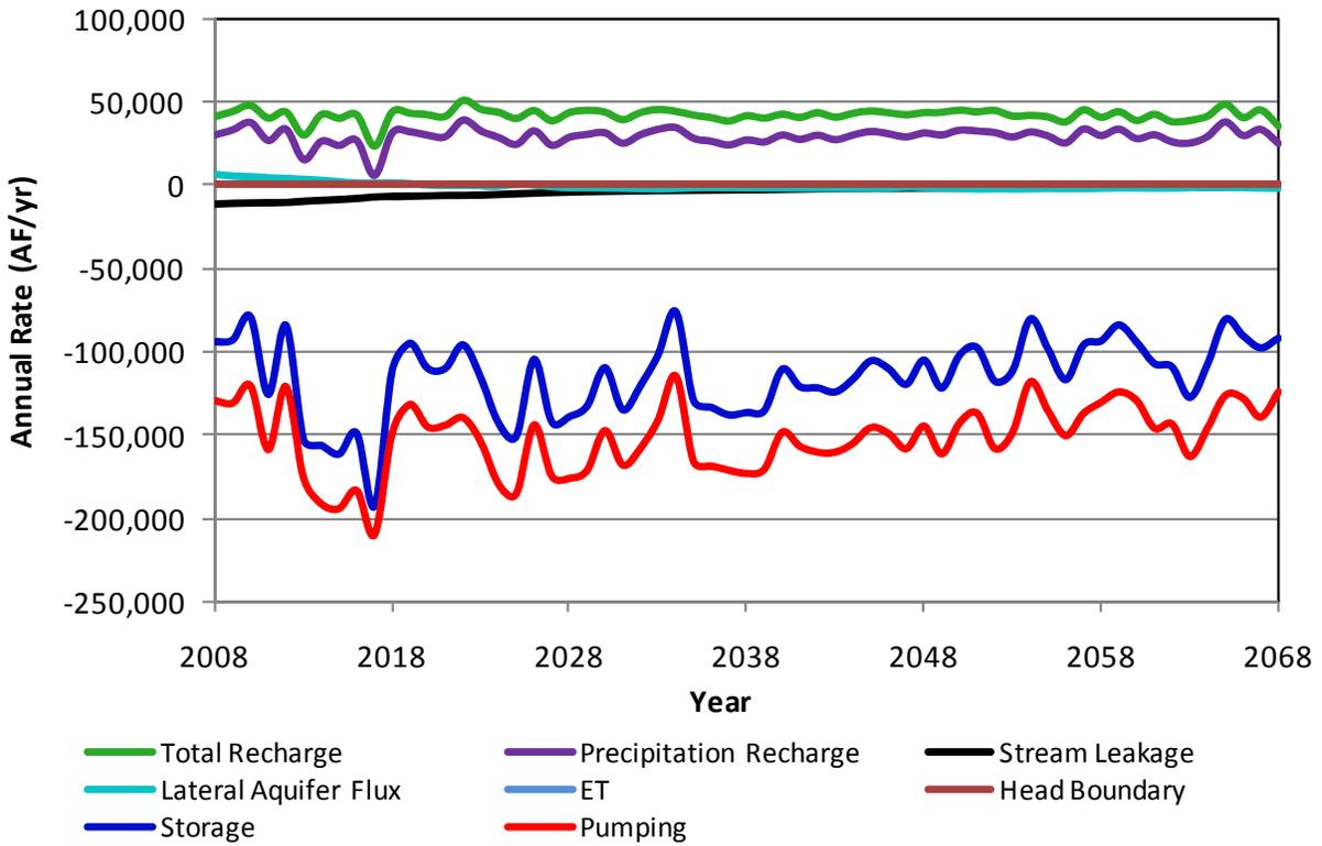
**Figure A11.** Components of the simulated aquifer budget for Seward County in scenario 1a.
