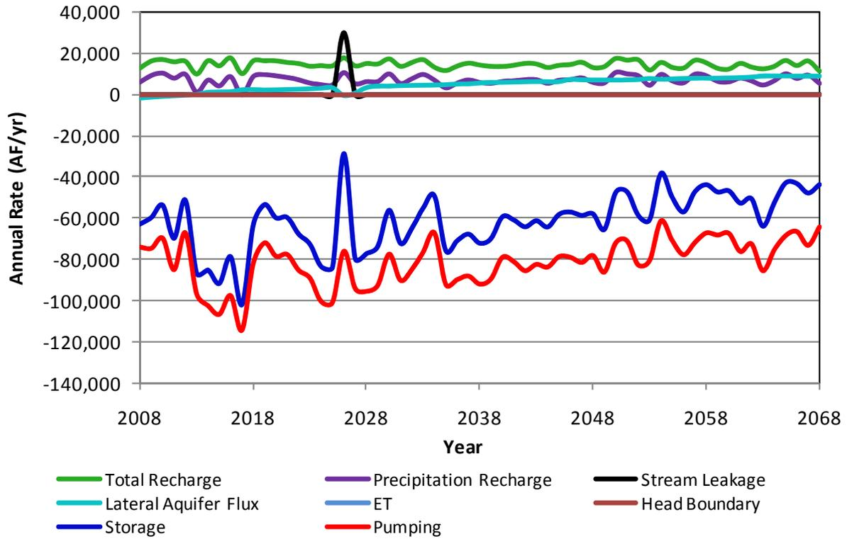
Figure A29. Components of the simulated aquifer budget for Grant County in scenario 3a.
