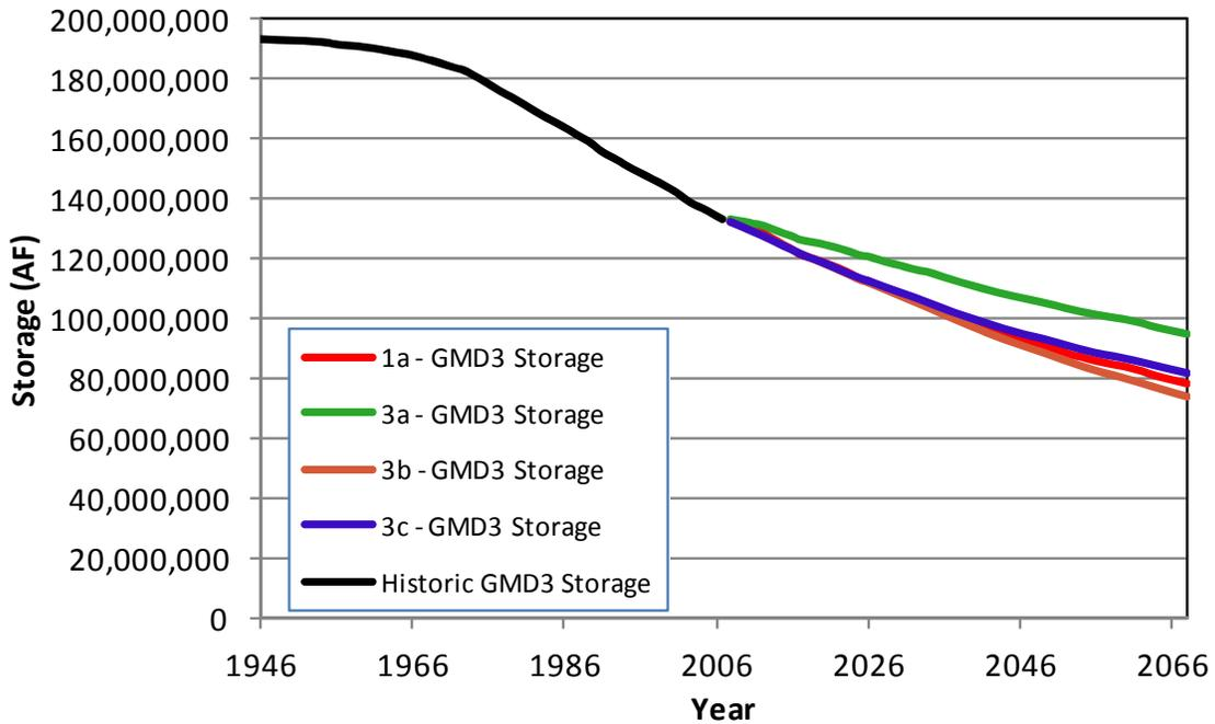
**Figure 72.** Change in simulated aquifer storage in GMD3 in scenario 3c.
