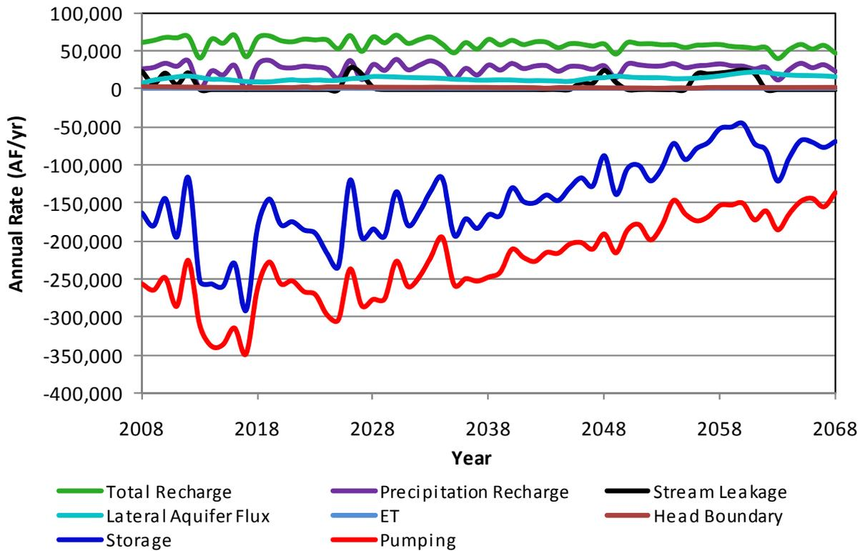
**Figure A19.** Components of the simulated aquifer budget for Finney County in scenario 1b.
