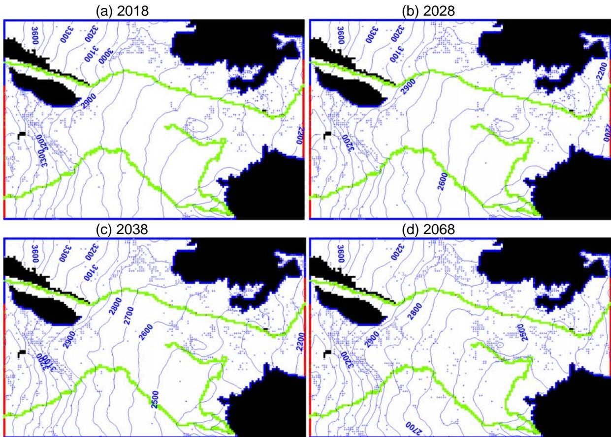
**Figure 68.** Distribution of wells that have a pumping rate reduction by more than 75% at different years in scenario 3c: (a) 2018, (b) 2028, (c) 2038, and (d) 2068.
