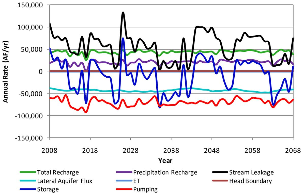
**Figure A28.** Components of the simulated aquifer budget for Kearny County in scenario 3a.
