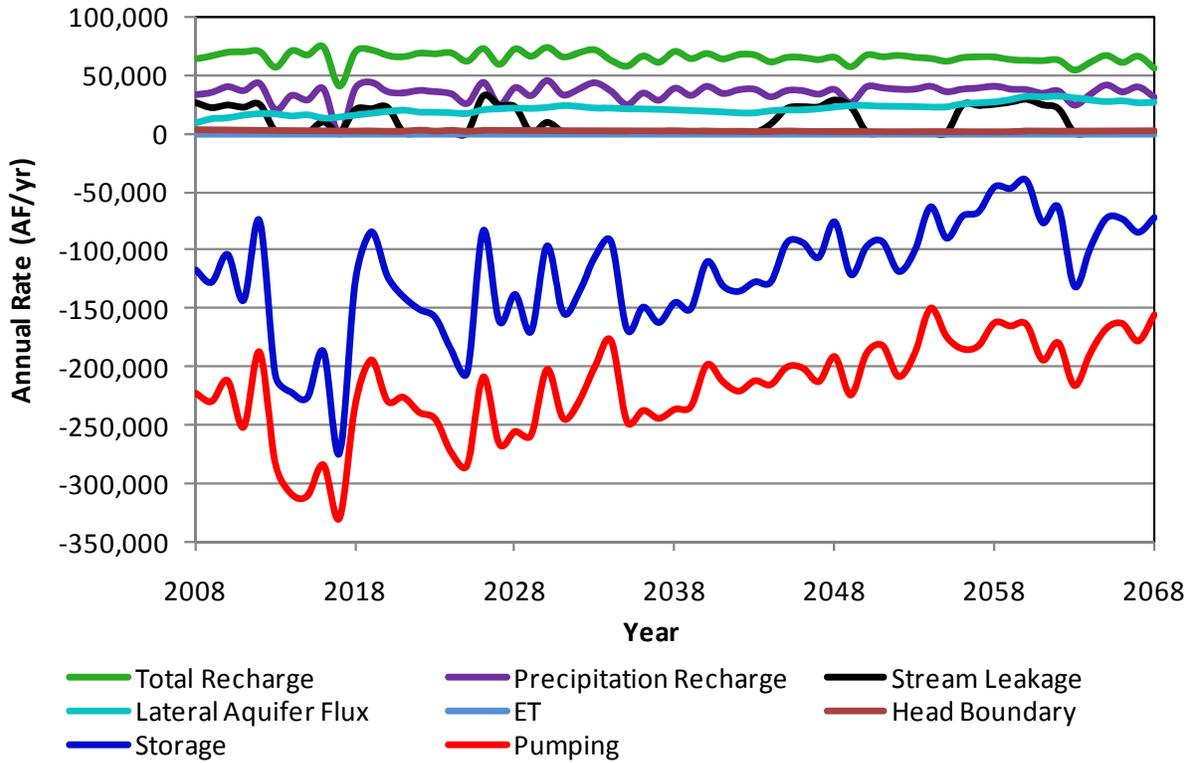
**Figure A7.** Components of the simulated aquifer budget for Finney County in scenario 1a.
