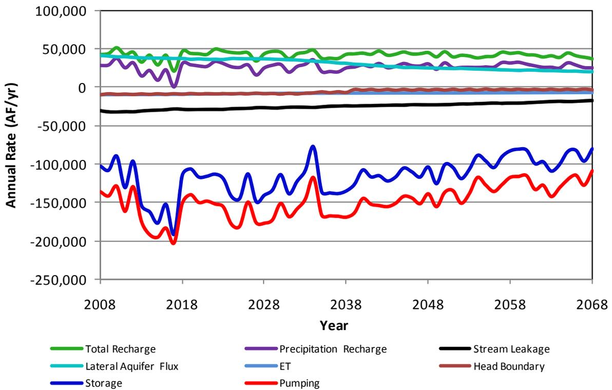
**Figure A21.** Components of the simulated aquifer budget for Meade County in scenario 1b.
