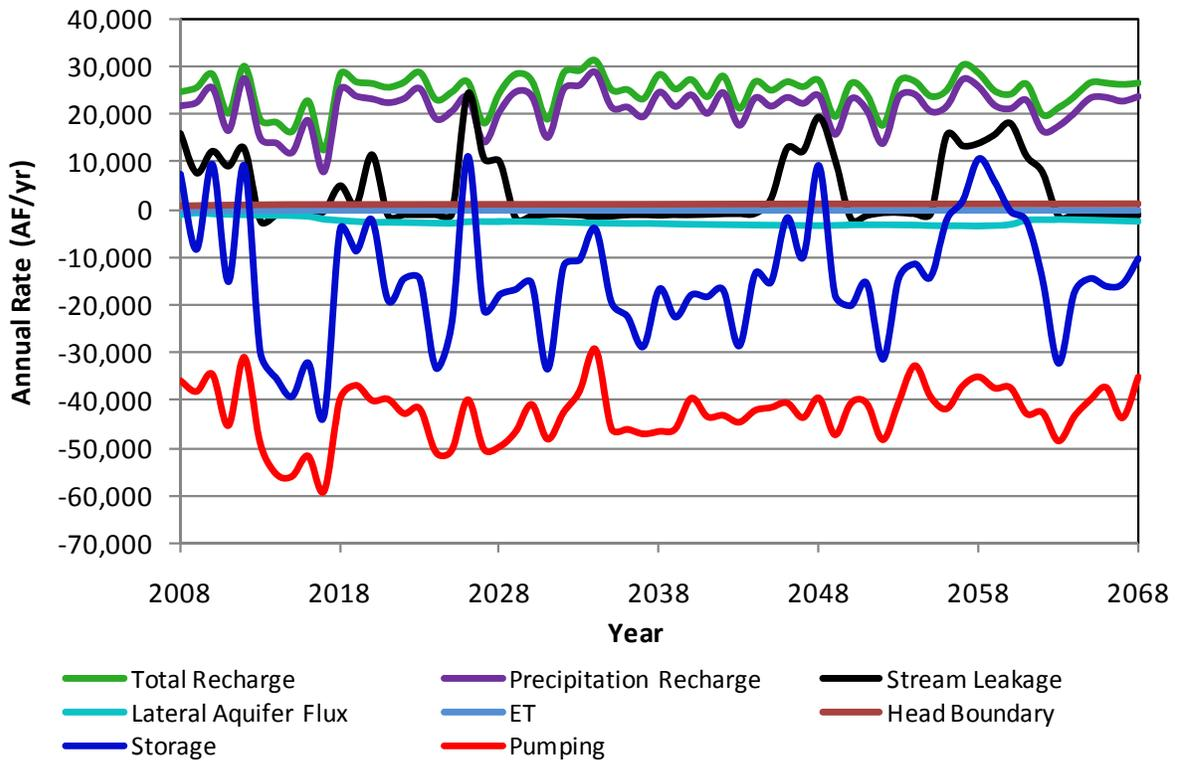
**Figure A36.** Components of the simulated aquifer budget for Ford County in scenario 3a.
