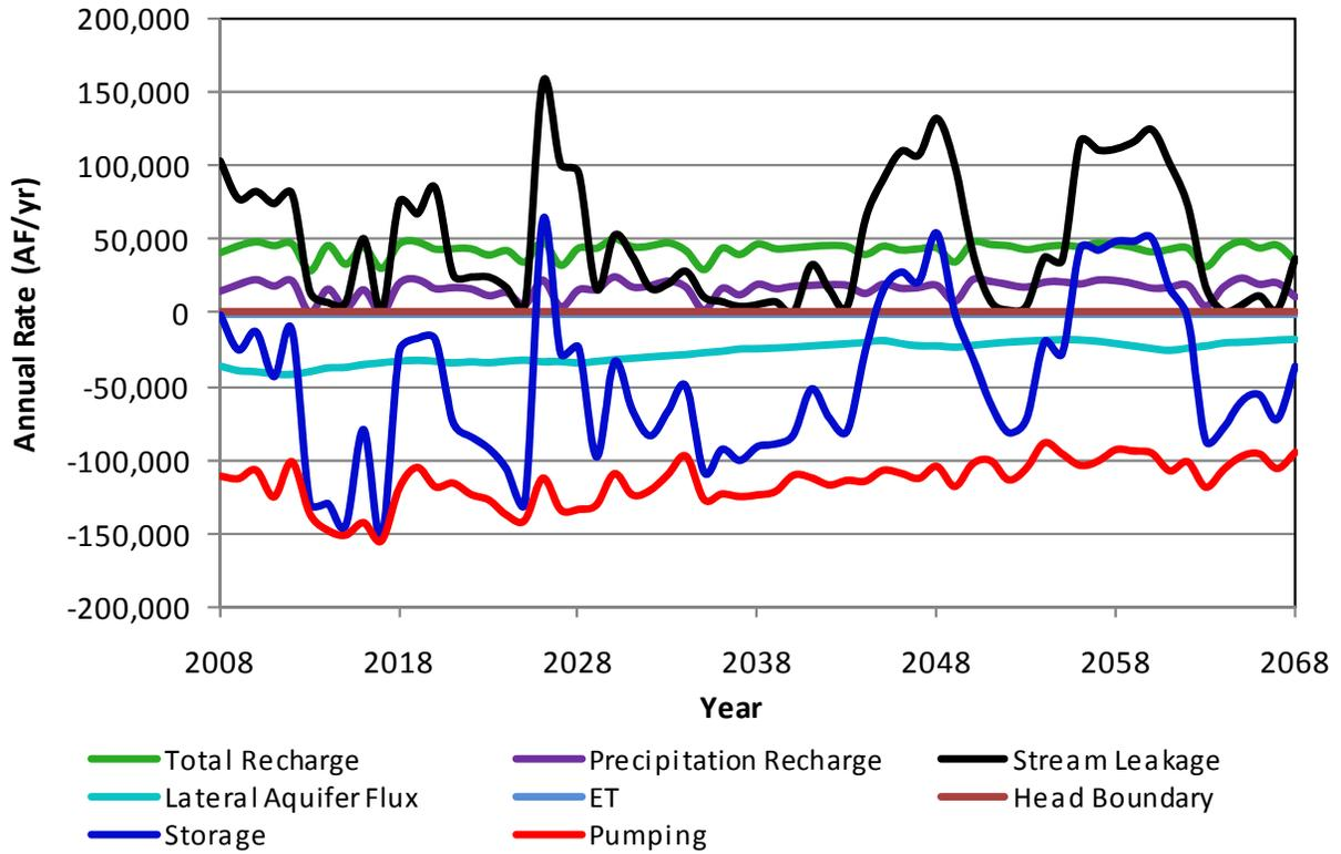
**Figure A16.** Components of the simulated aquifer budget for Kearny County in scenario 1b.
