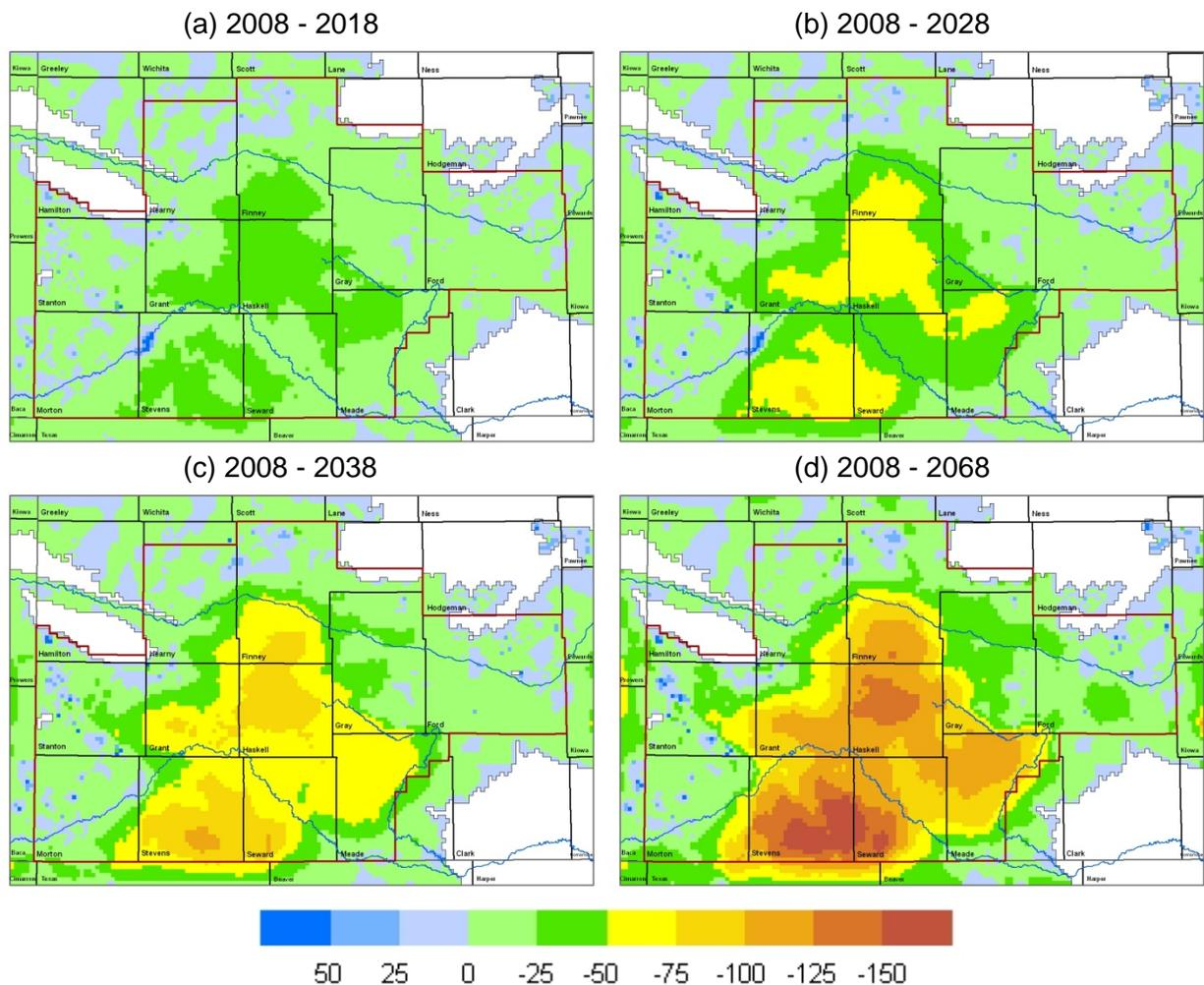
**Figure 70.** Simulated water level changes (in ft) for different time intervals in scenario 3c: (a) 2008 - 2018, (b) 2008 - 2028, (c) 2008 - 2038, and (d) 2008 - 2068.
