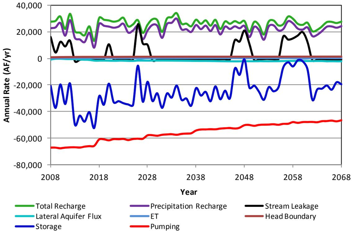
**Figure A60.** Components of the simulated aquifer budget for Ford County in scenario 3c.
