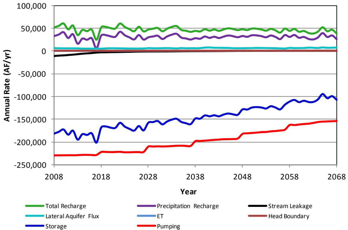
**Figure A59.** Components of the simulated aquifer budget for Seward County in scenario 3c.
