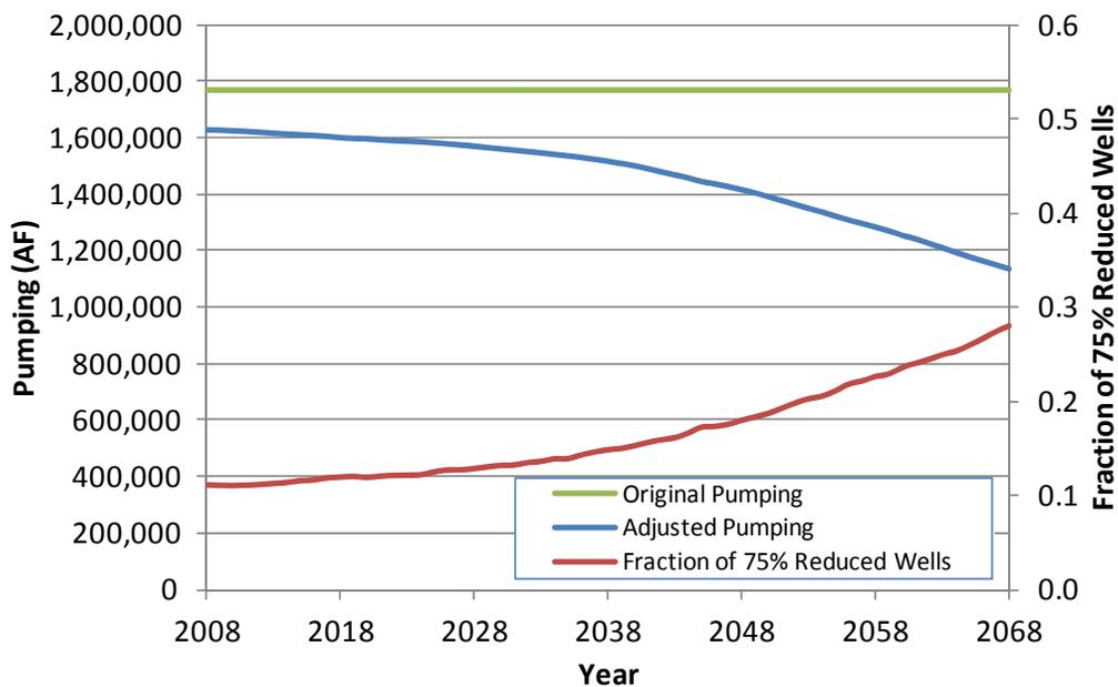
**Figure 56.** Adjusted versus original model pumping, and the fraction of wells with rate reduced greater than 75% in GMD3 in scenario 3b.
