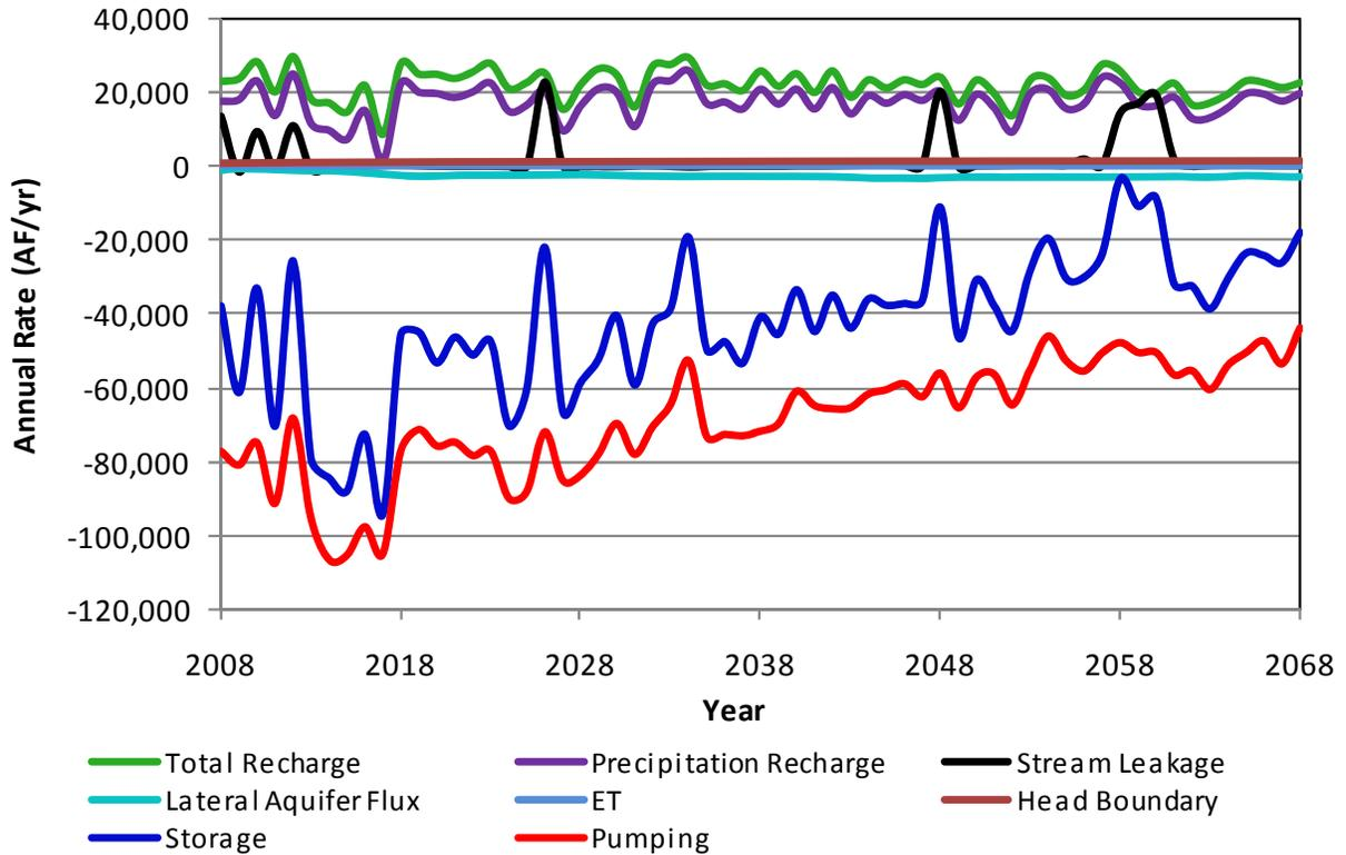
**Figure A24.** Components of the simulated aquifer budget for Ford County in scenario 1b.
