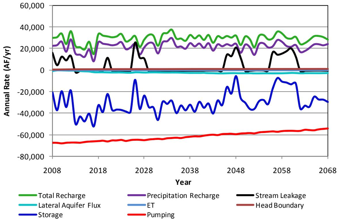
**Figure A48.** Components of the simulated aquifer budget for Ford County in scenario 3b.
