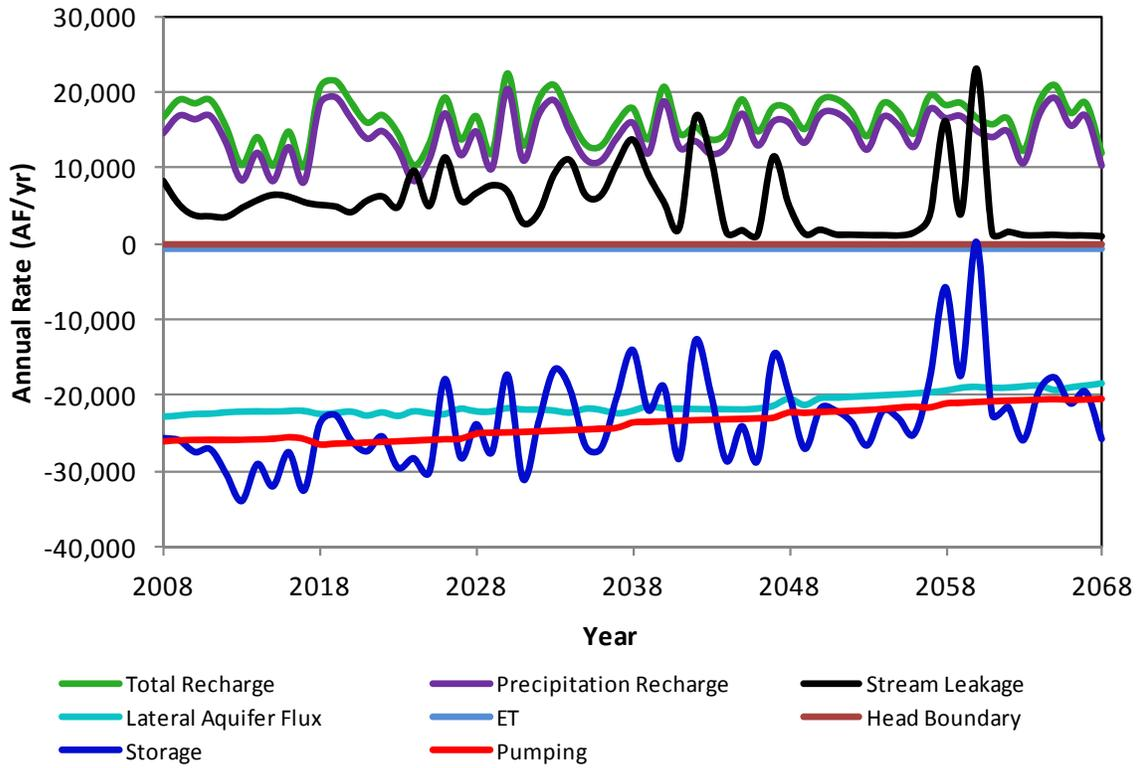
**Figure A50.** Components of the simulated aquifer budget for Morton County in scenario 3c.
