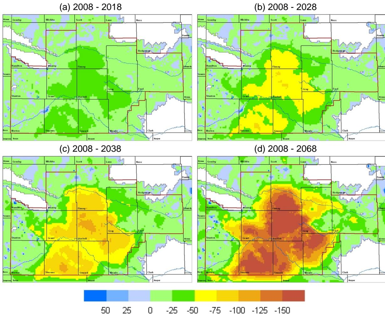
**Figure 57.** Simulated water level changes (in ft) for different time intervals in scenario 3b: (a) 2008 - 2018, (b) 2008 - 2028, (c) 2008 - 2038, and (d) 2008 - 2068.
