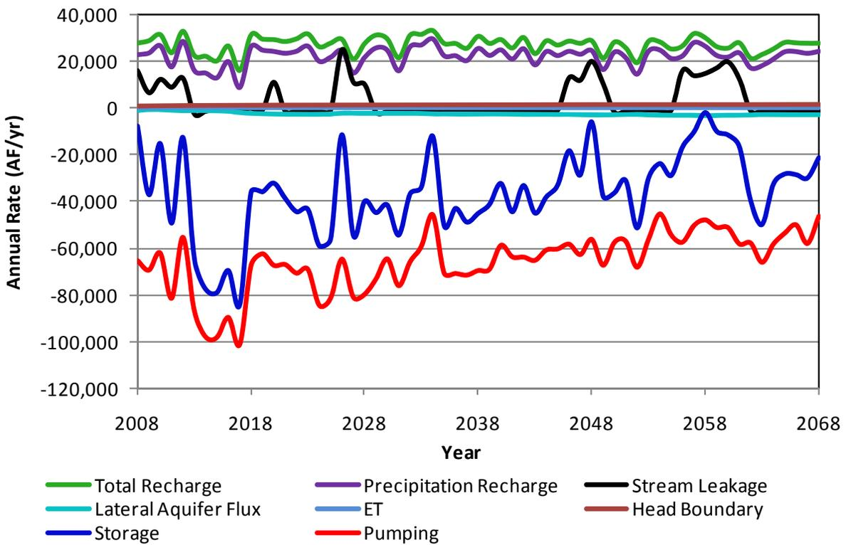
**Figure A12.** Components of the simulated aquifer budget for Ford County in scenario 1a.
