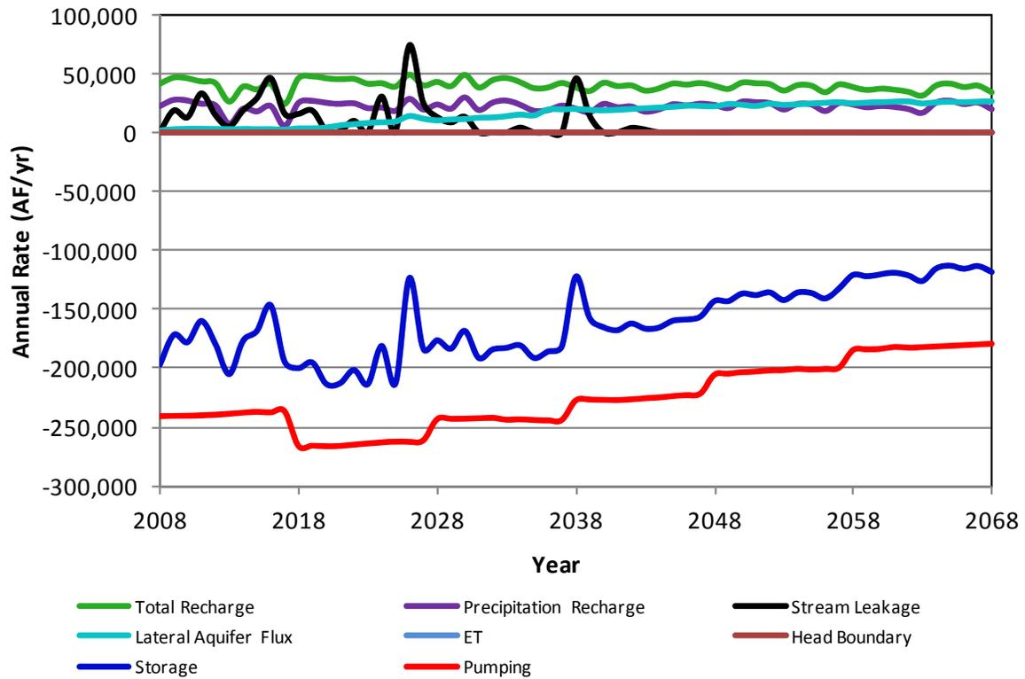
**Figure A54.** Components of the simulated aquifer budget for Stevens County in scenario 3c.
