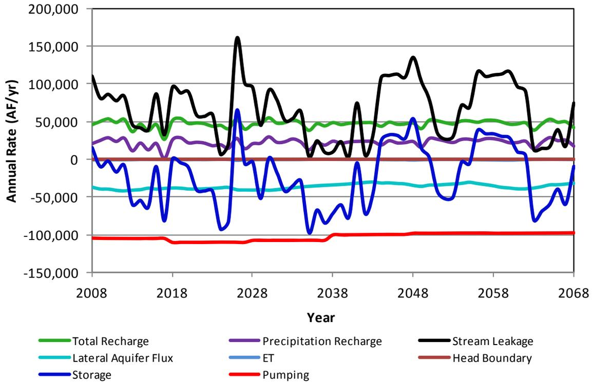
**Figure A52.** Components of the simulated aquifer budget for Kearny County in scenario 3c.
