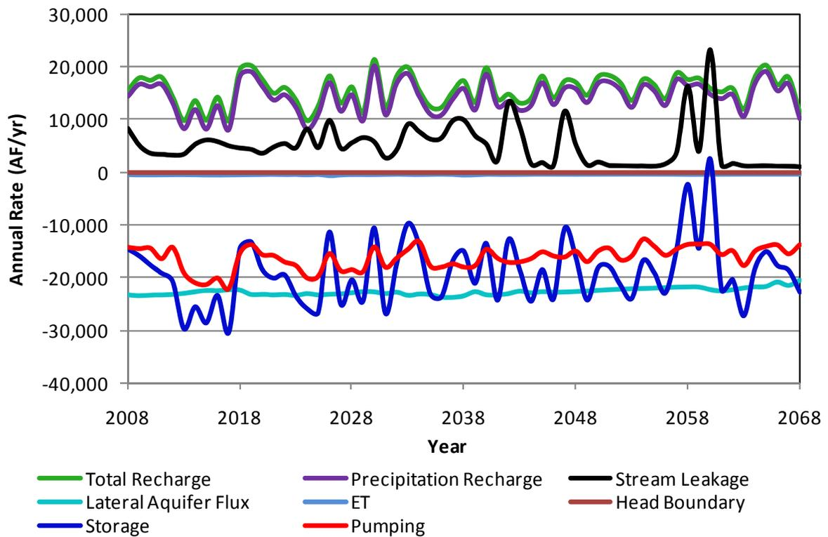
**Figure A2.** Components of the simulated aquifer budget for Morton County in scenario 1a.
