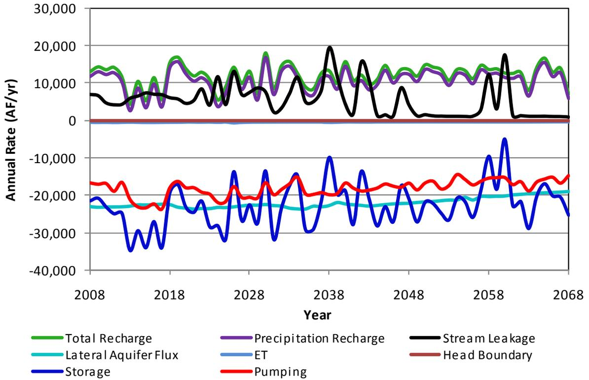
**Figure A14.** Components of the simulated aquifer budget for Morton County in scenario 1b.
