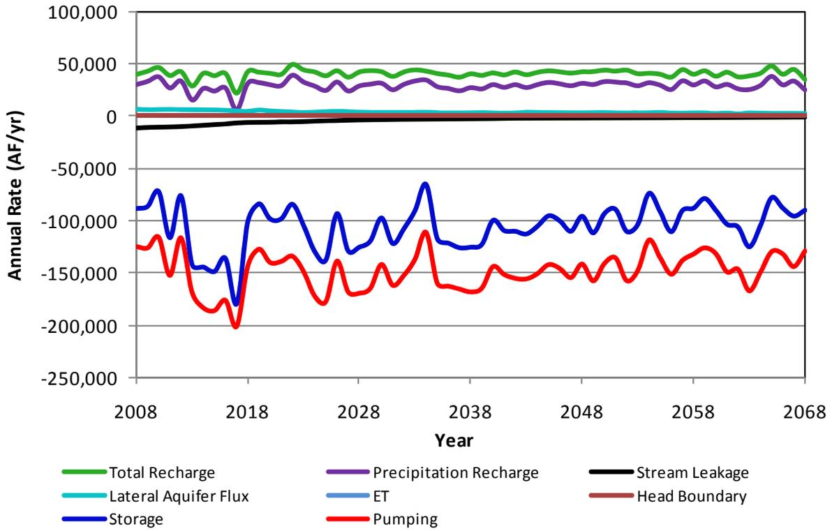
**Figure A35.** Components of the simulated aquifer budget for Seward County in scenario 3a.
