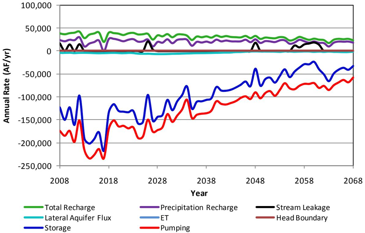
**Figure A22.** Components of the simulated aquifer budget for Gray County in scenario 1b.
