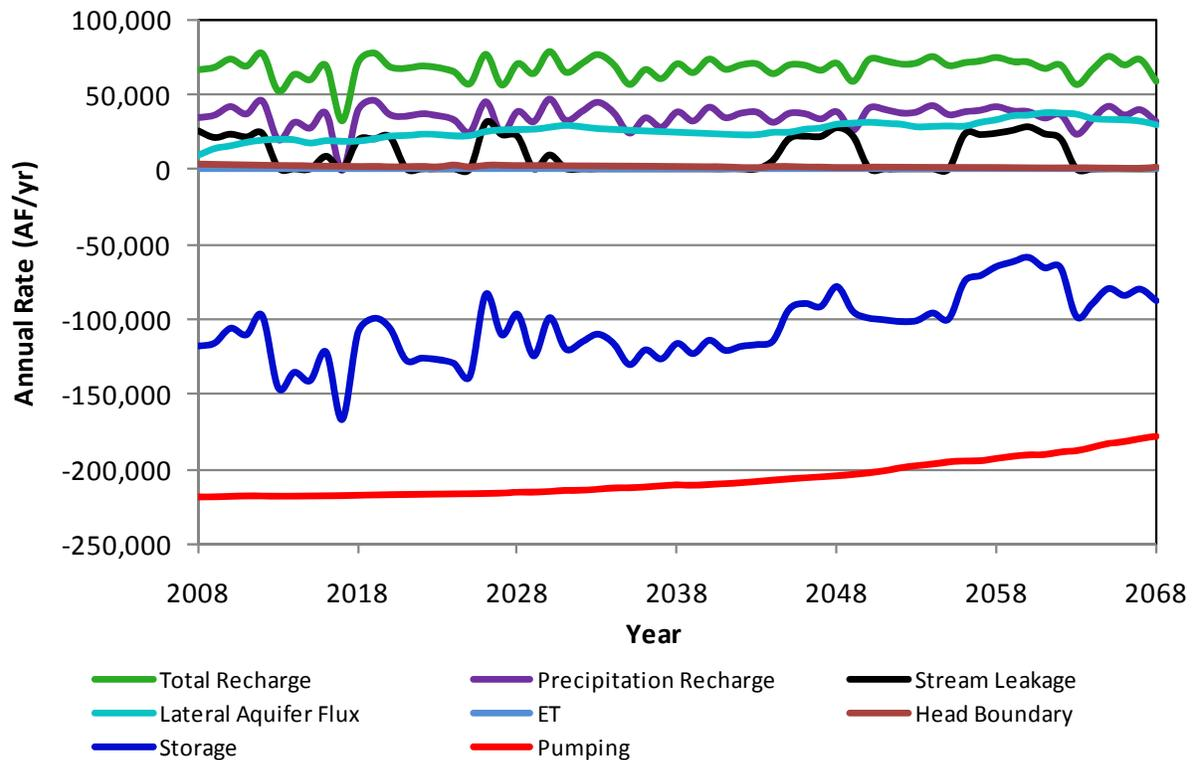
**Figure A43.** Components of the simulated aquifer budget for Finney County in scenario 3b.
