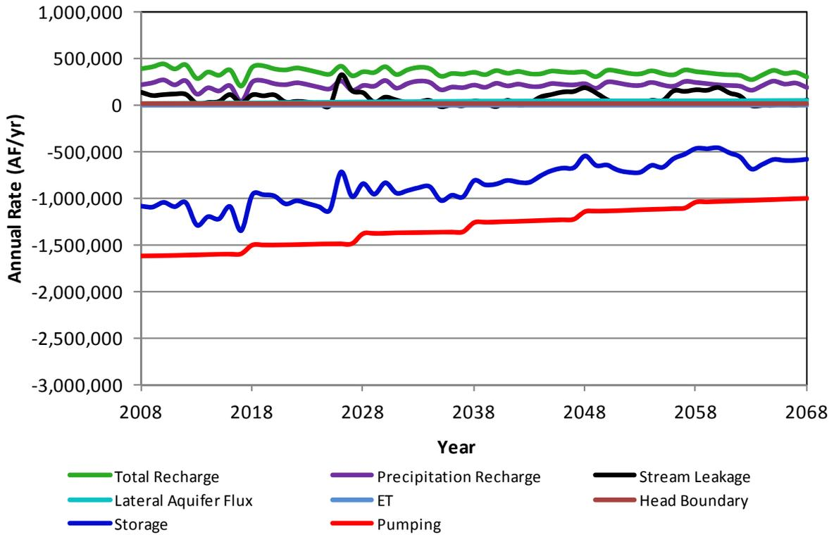
**Figure 75.** Components of the simulated aquifer budget for the GMD3 area in scenario 3c.
