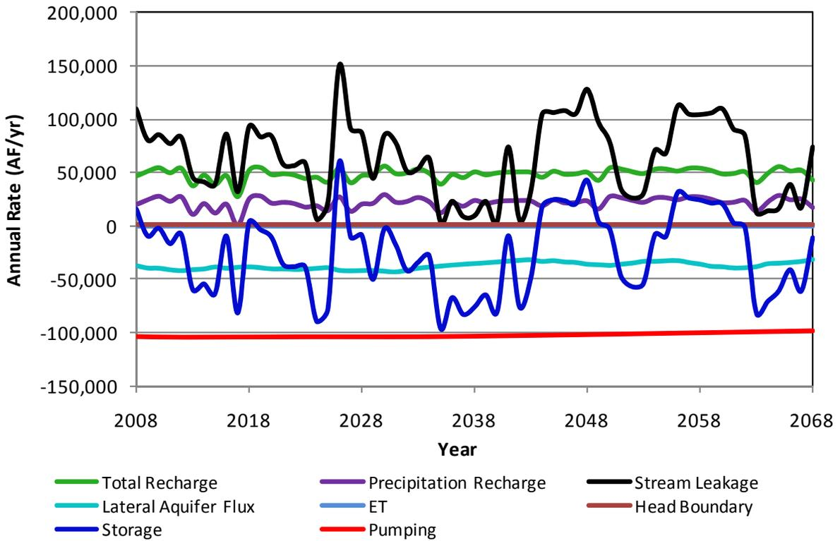
**Figure A40.** Components of the simulated aquifer budget for Kearny County in scenario 3b.
