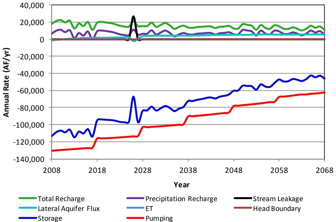
**Figure A53.** Components of the simulated aquifer budget for Grant County in scenario 3c.
