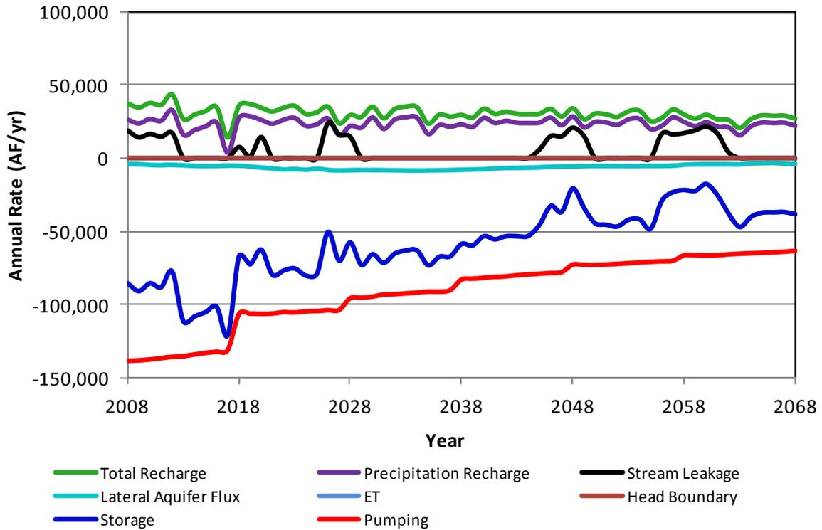
**Figure A58.** Components of the simulated aquifer budget for Gray County in scenario 3c.
