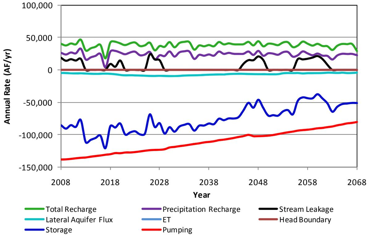
**Figure A46.** Components of the simulated aquifer budget for Gray County in scenario 3b.
