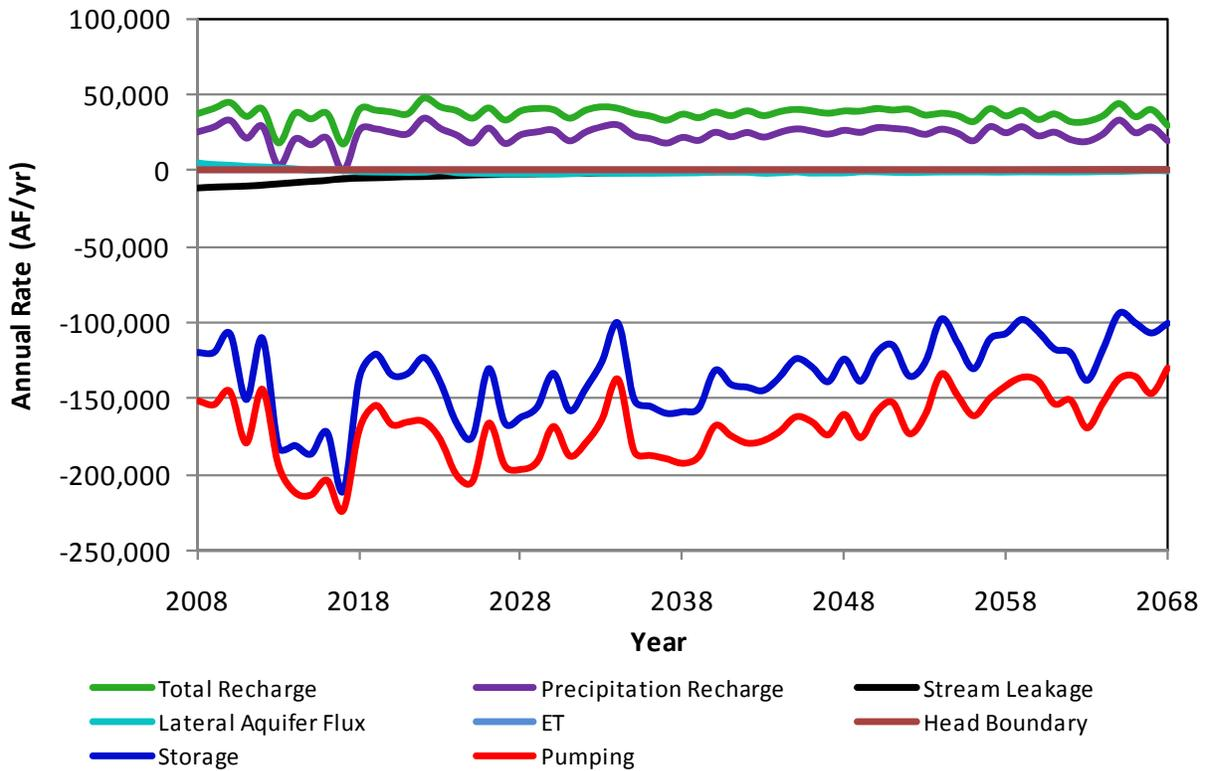
**Figure A23.** Components of the simulated aquifer budget for Seward County in scenario 1b.
