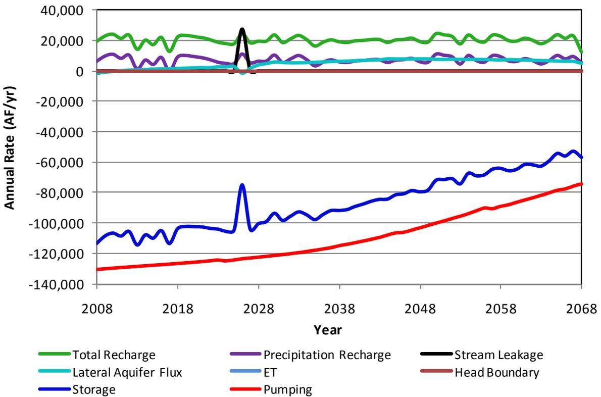
**Figure A41.** Components of the simulated aquifer budget for Grant County in scenario 3b.
