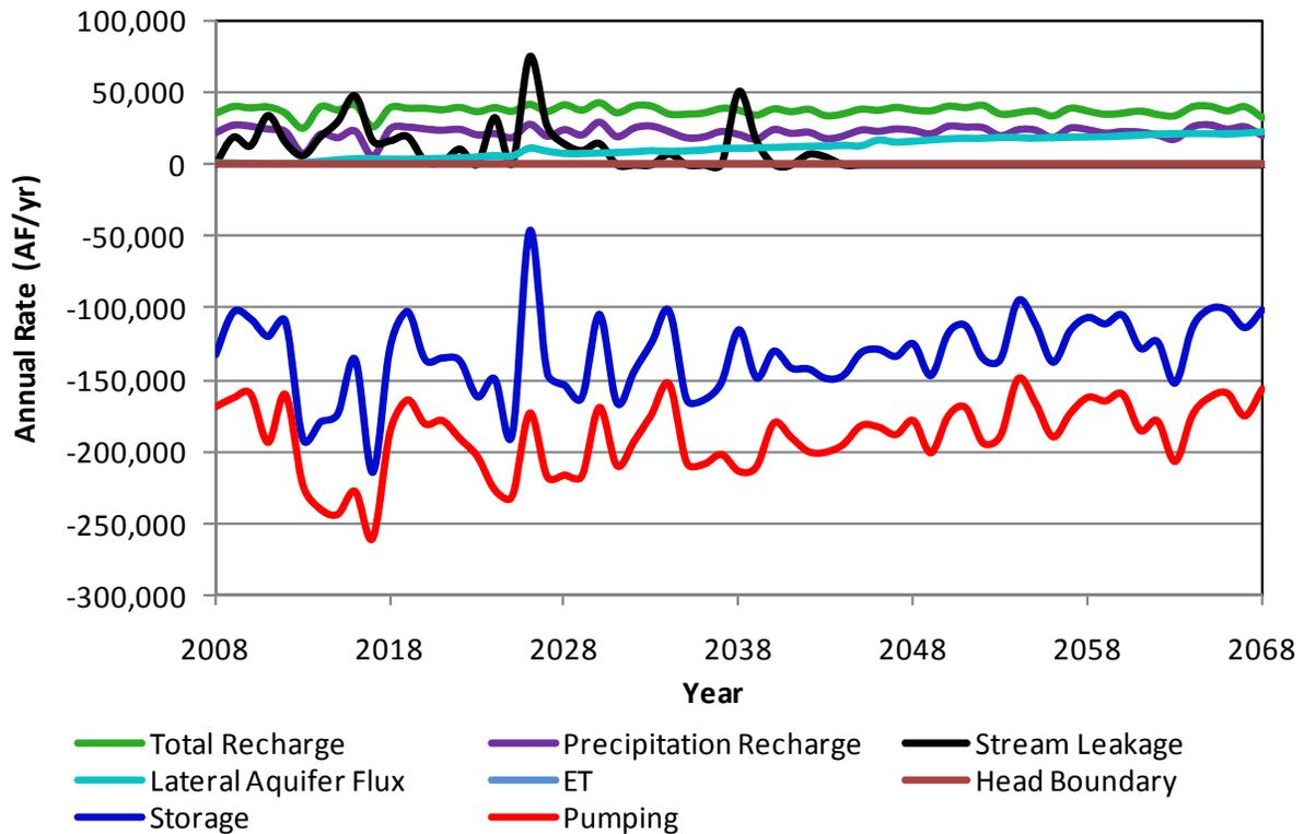
**Figure A6.** Components of the simulated aquifer budget for Stevens County in scenario 1a.
