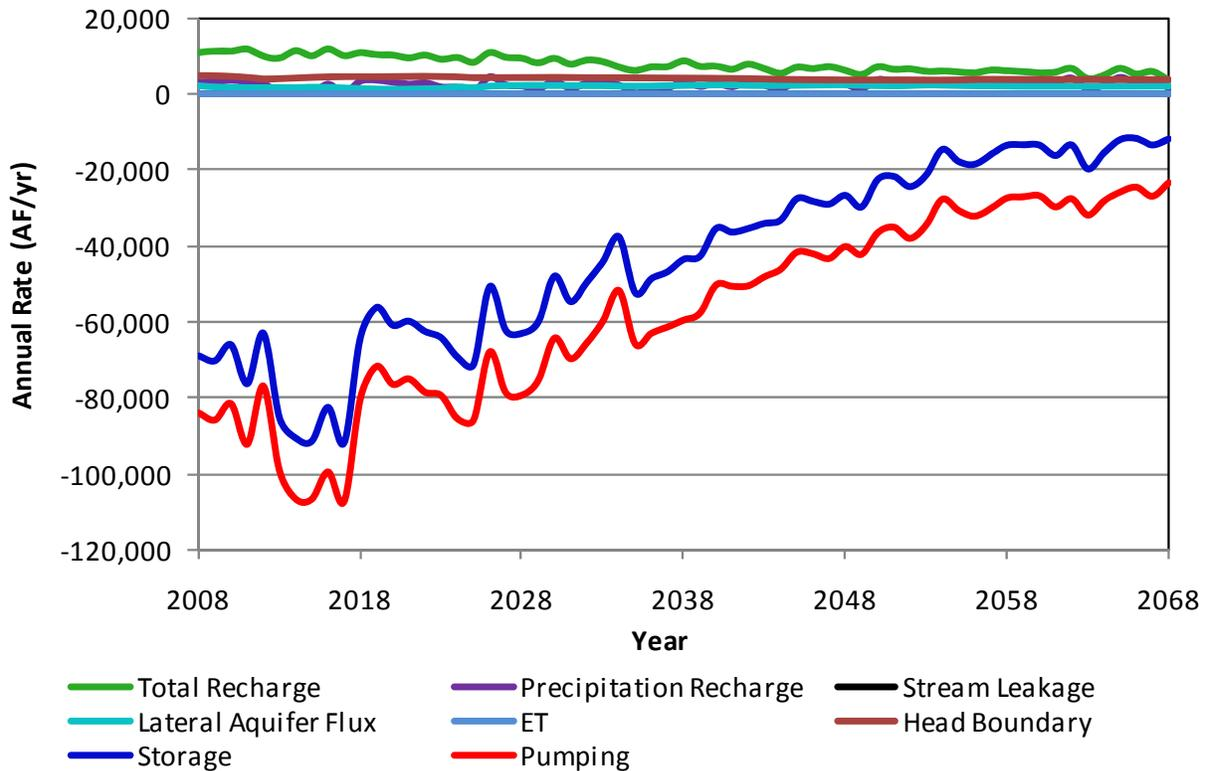
**Figure A15.** Components of the simulated aquifer budget for Stanton County in scenario 1b.
