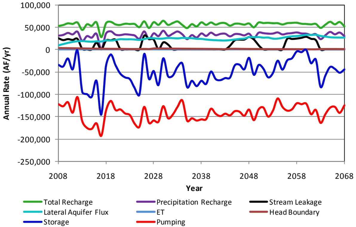
**Figure A31.** Components of the simulated aquifer budget for Finney County in scenario 3a.
