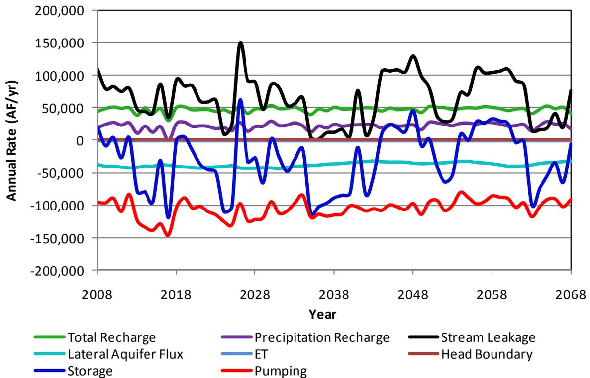
**Figure A4.** Components of the simulated aquifer budget for Kearny County in scenario 1a.
