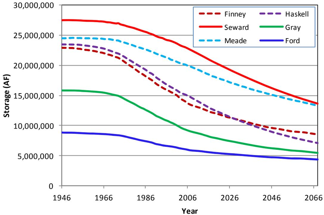
**Figure 74.** Changes in simulated aquifer storage for the six eastern counties in scenario 3c.
