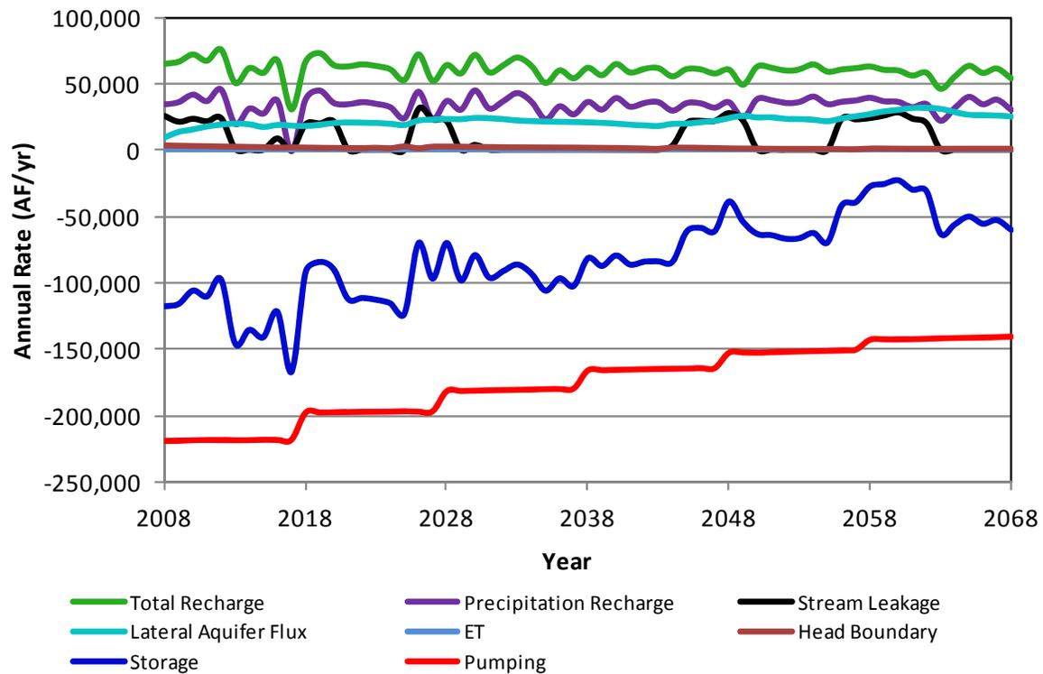
**Figure A55.** Components of the simulated aquifer budget for Finney County in scenario 3c.
