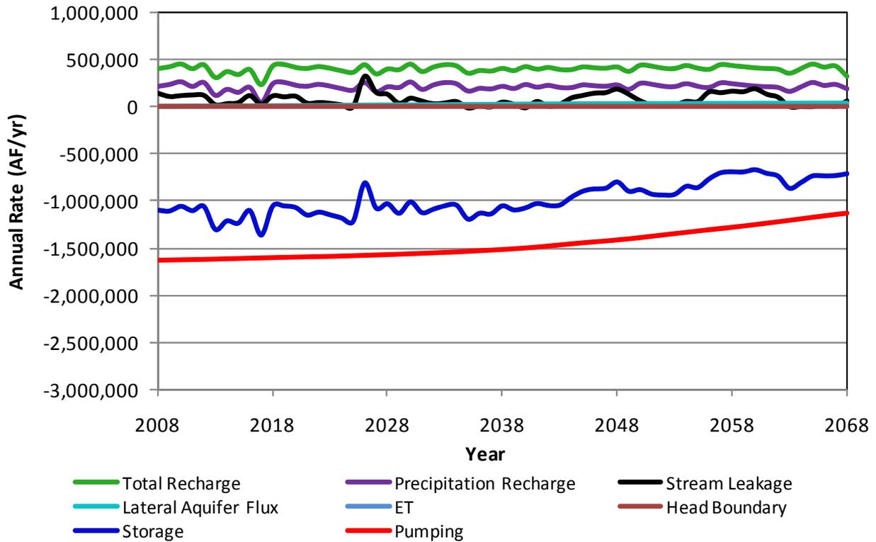
**Figure 62.** Components of the simulated aquifer budget for the GMD3 area in scenario 3b.
