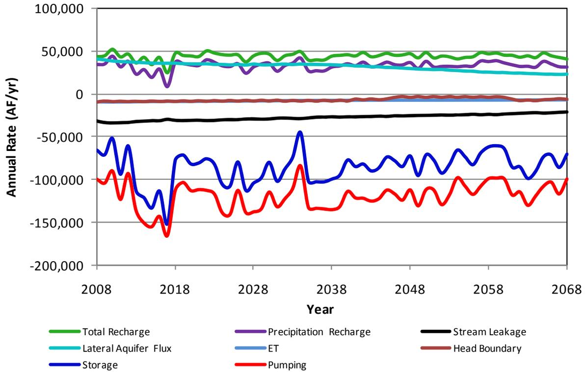
**Figure A33.** Components of the simulated aquifer budget for Meade County in scenario 3a.
