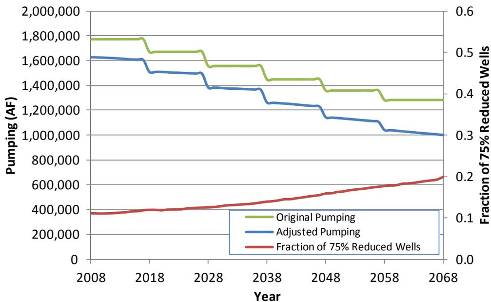
**Figure 69.** Adjusted versus original model pumping, and the fraction of wells with rate reduced greater than 75% in GMD3 in scenario 3c.
