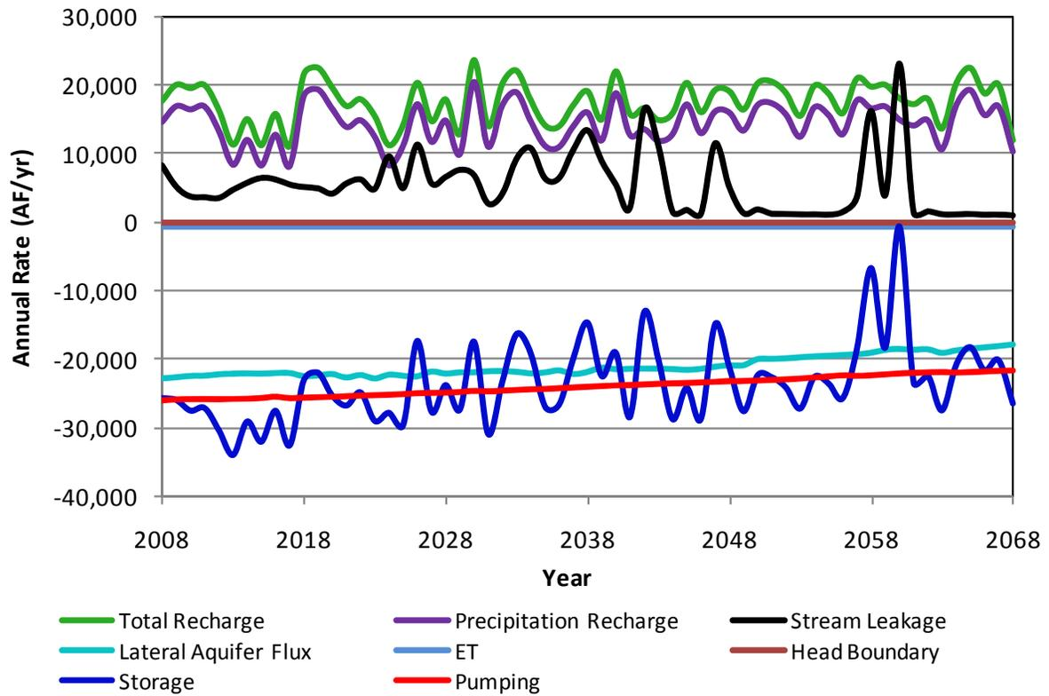
**Figure A38.** Components of the simulated aquifer budget for Morton County in scenario 3b.
