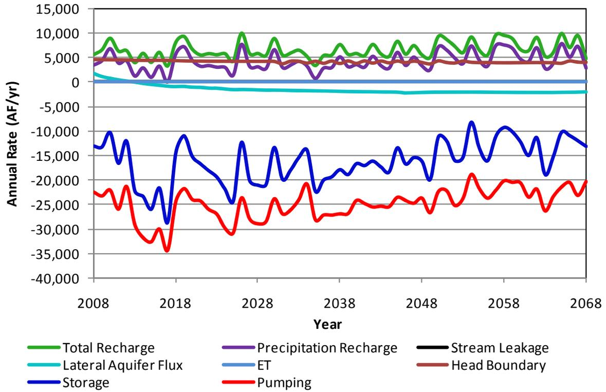
**Figure A27.** Components of the simulated aquifer budget for Stanton County in scenario 3a.
