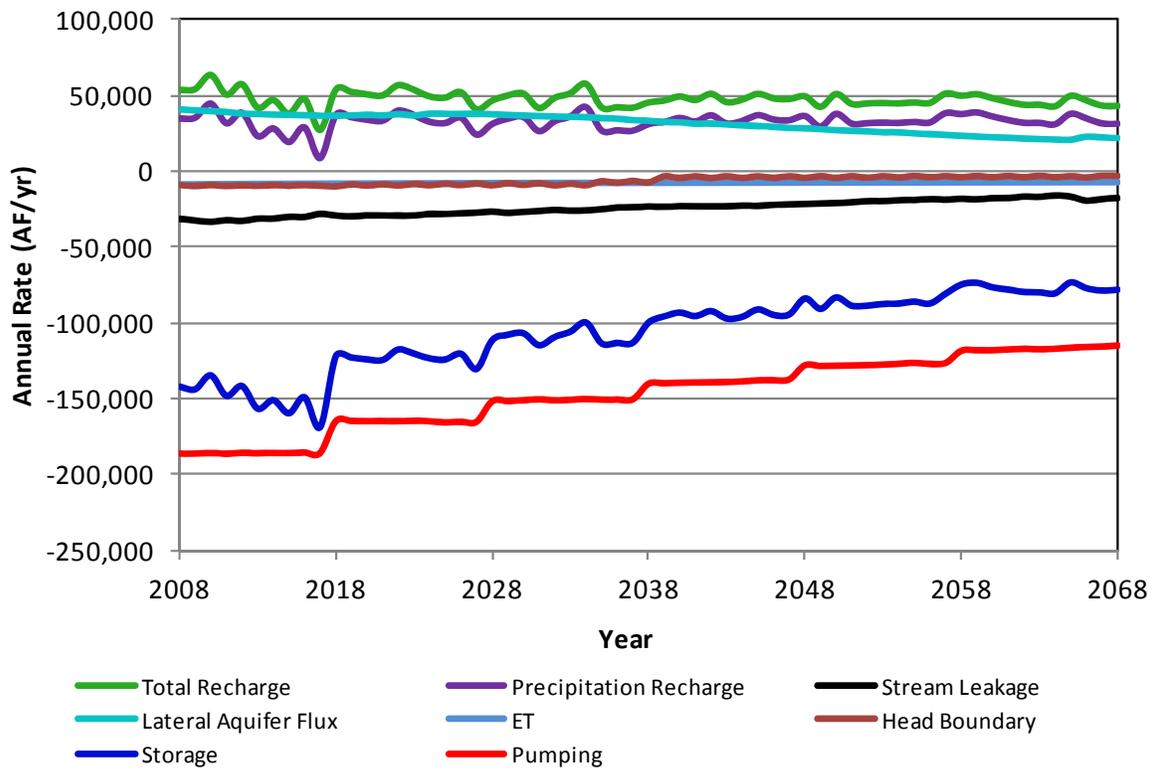
**Figure A57.** Components of the simulated aquifer budget for Meade County in scenario 3c.
