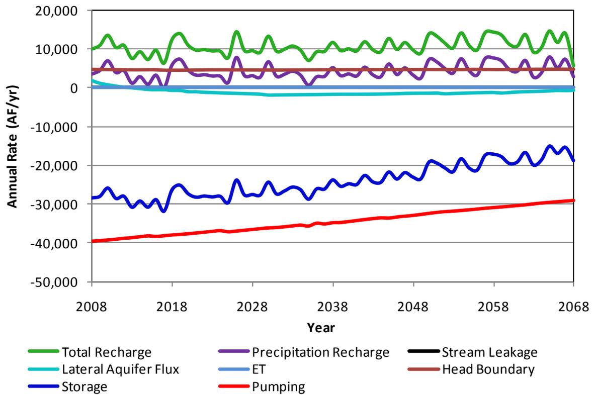
**Figure A39.** Components of the simulated aquifer budget for Stanton County in scenario 3b.
