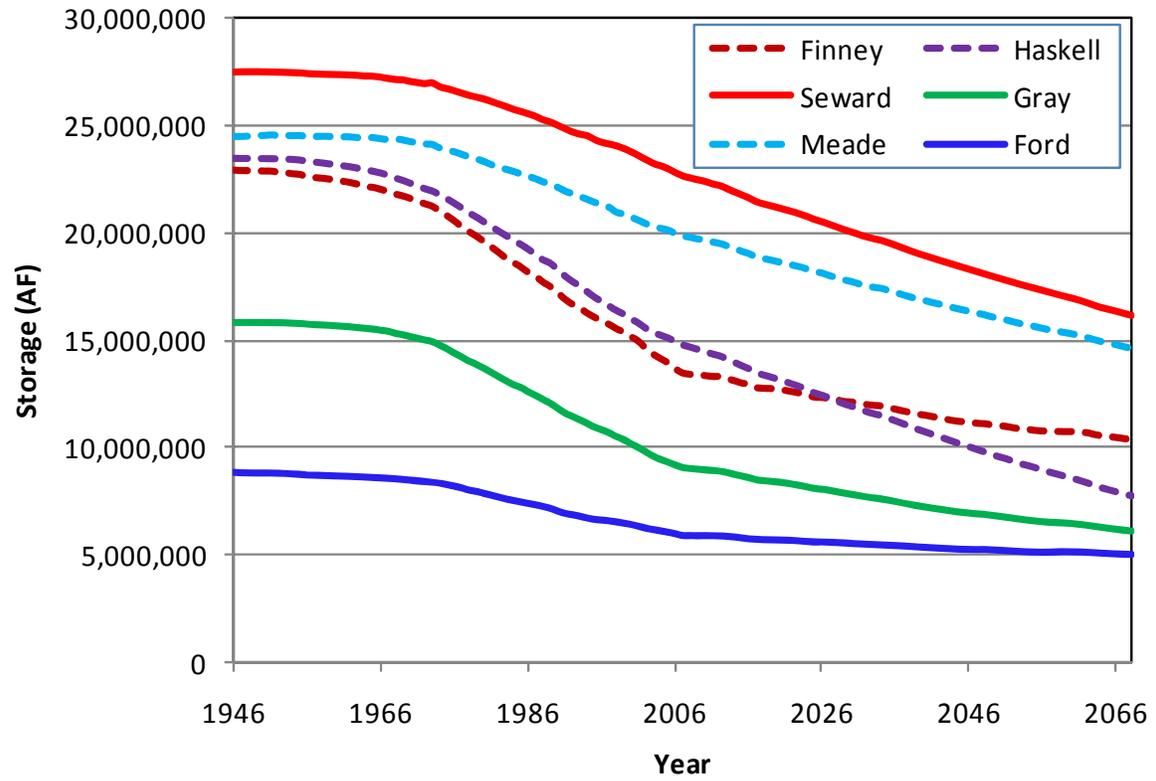
**Figure 48.** Changes in simulated aquifer storage for the six eastern counties in scenario 3a.
