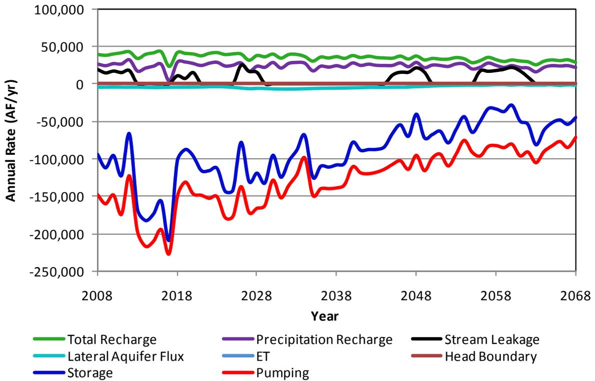
**Figure A10.** Components of the simulated aquifer budget for Gray County in scenario 1a.
