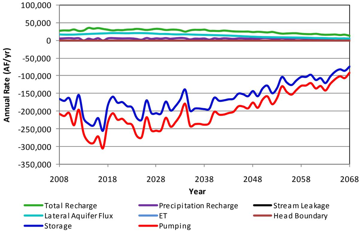
**Figure A20.** Components of the simulated aquifer budget for Haskell County in scenario 1b.
