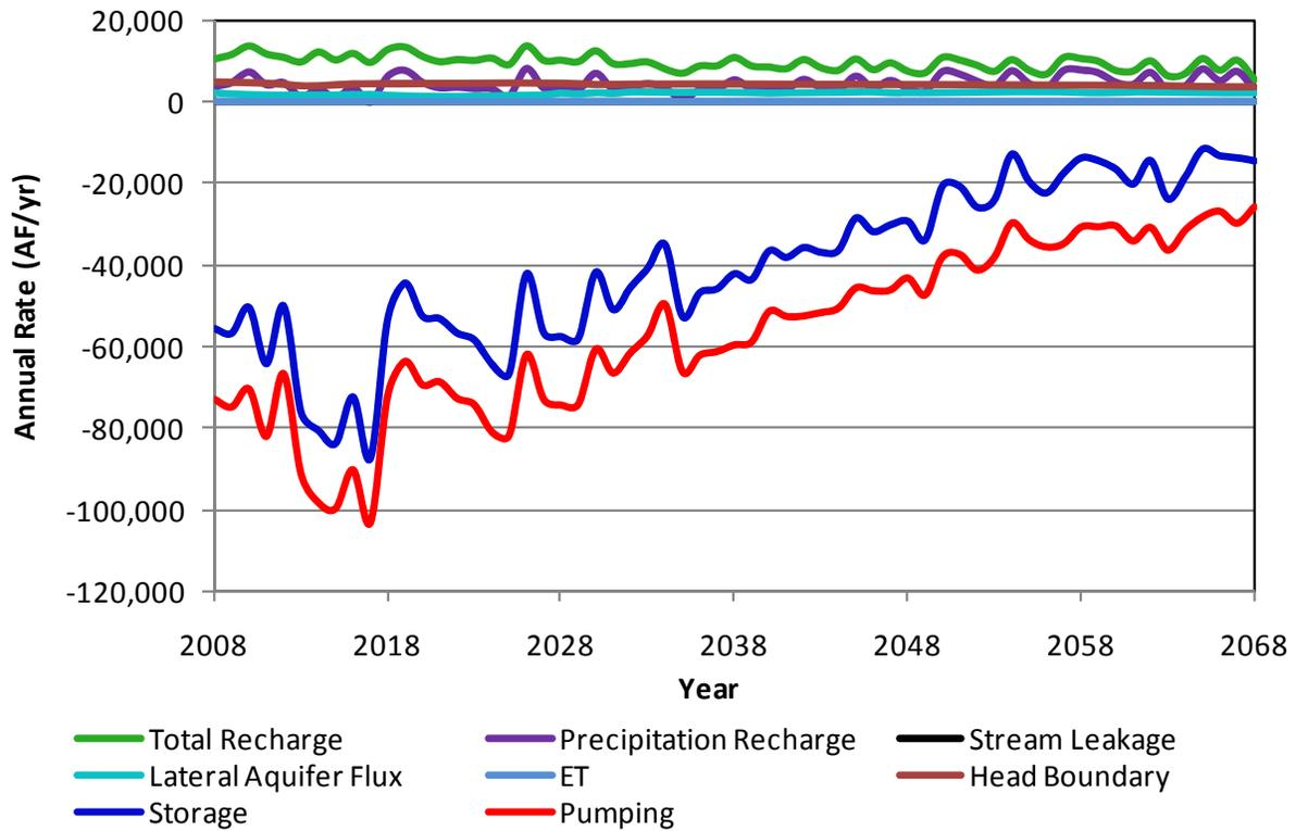
**Figure A3.** Components of the simulated aquifer budget for Stanton County in scenario 1a.
