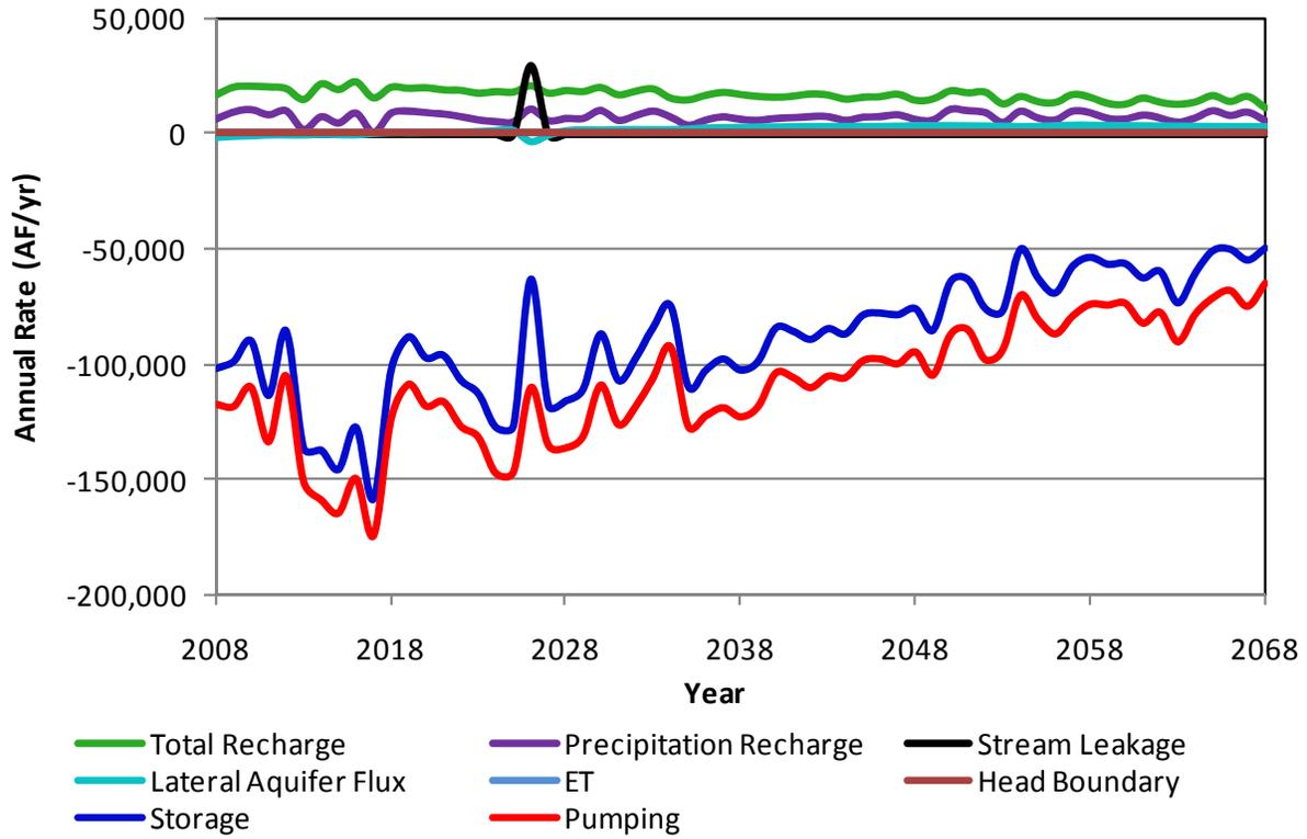
**Figure A5.** Components of the simulated aquifer budget for Grant County in scenario 1a.
