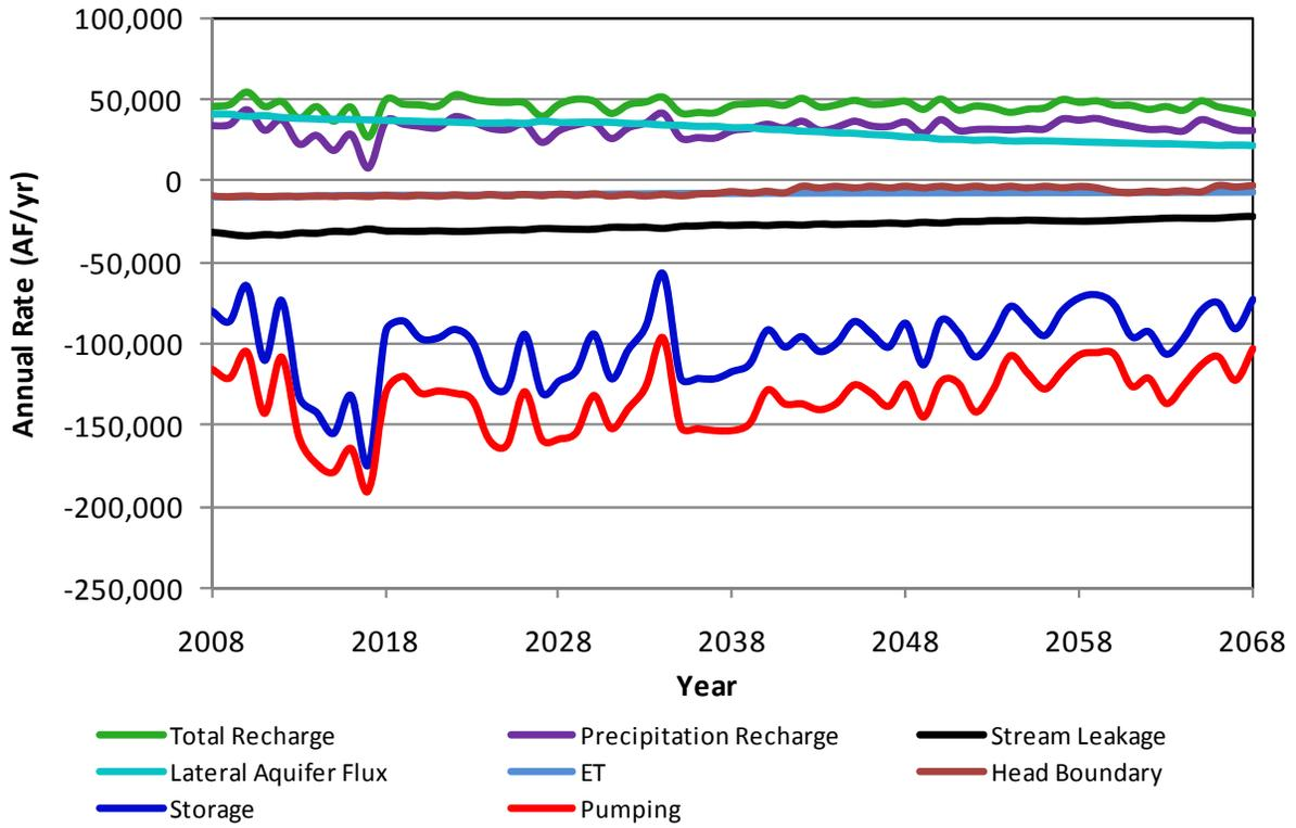
**Figure A9.** Components of the simulated aquifer budget for Meade County in scenario 1a.
