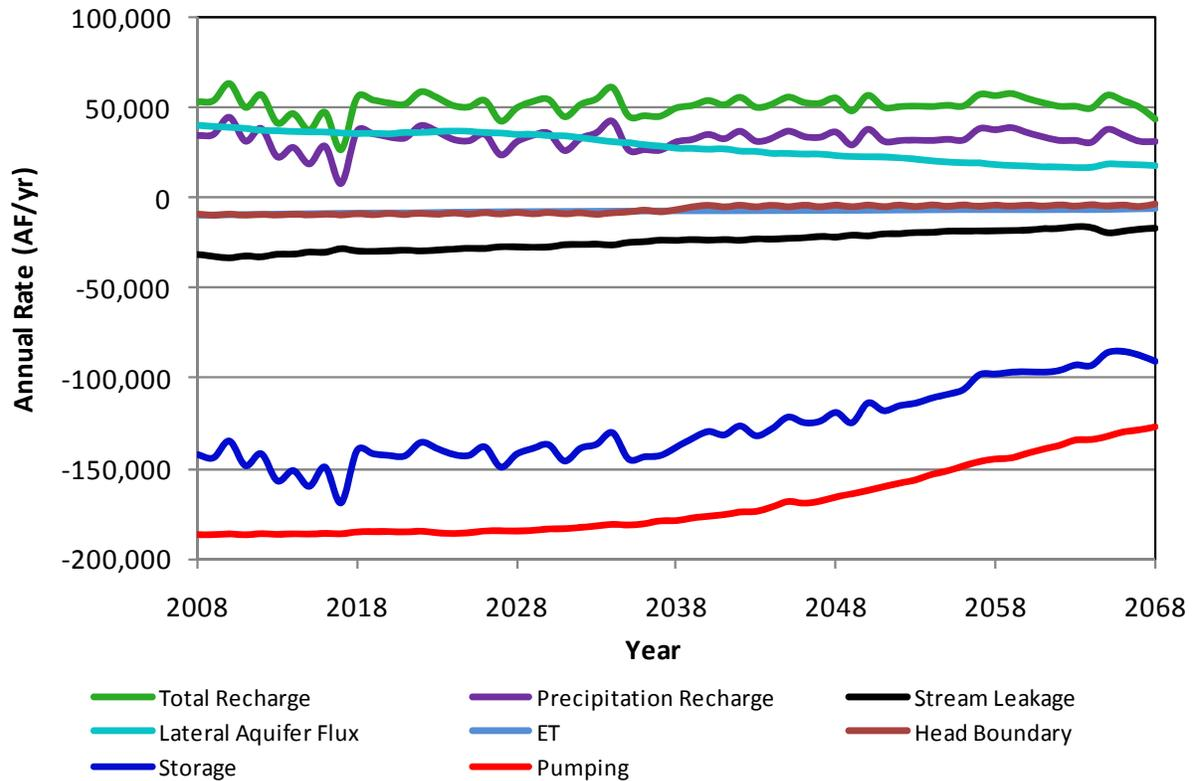
**Figure A45.** Components of the simulated aquifer budget for Meade County in scenario 3b.
