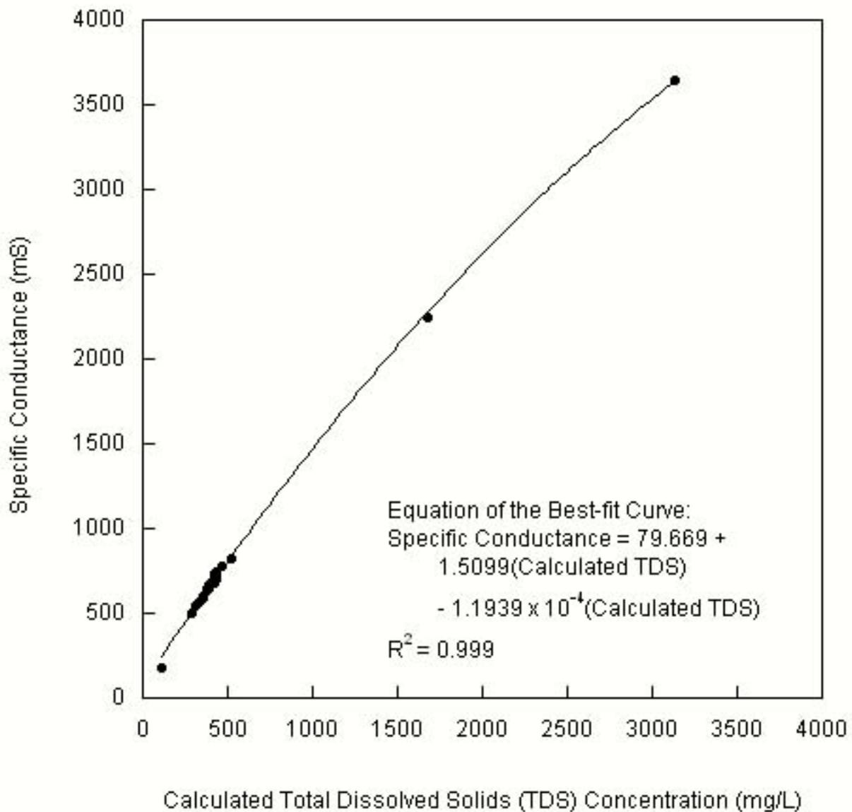
Figure 52. Calculated total dissolved solids concentration vs laboratory measured specific conductance with a best-fit curve from polynomial regression.
