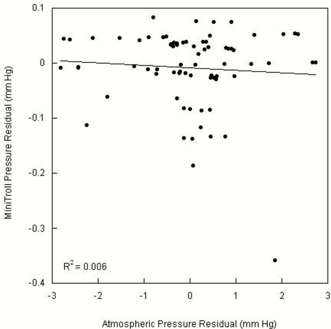
Figure 50. Atmospheric pressure residuals vs MiniTroll pressure residuals in mm Hg for the "out-of-water" test with a best-fit line from linear regression.
