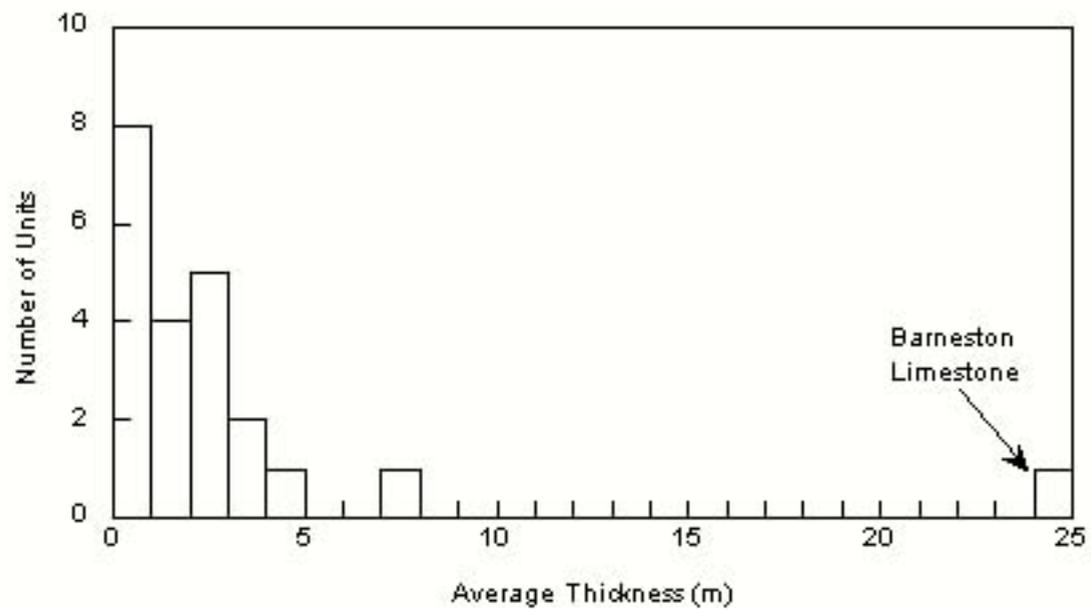
Figure 70. Histogram showing the average thickness of limestone units in the outcrop belt of the Council Grove and Chase Groups in Kansas based on average unit thicknesses in Zeller (1968).
