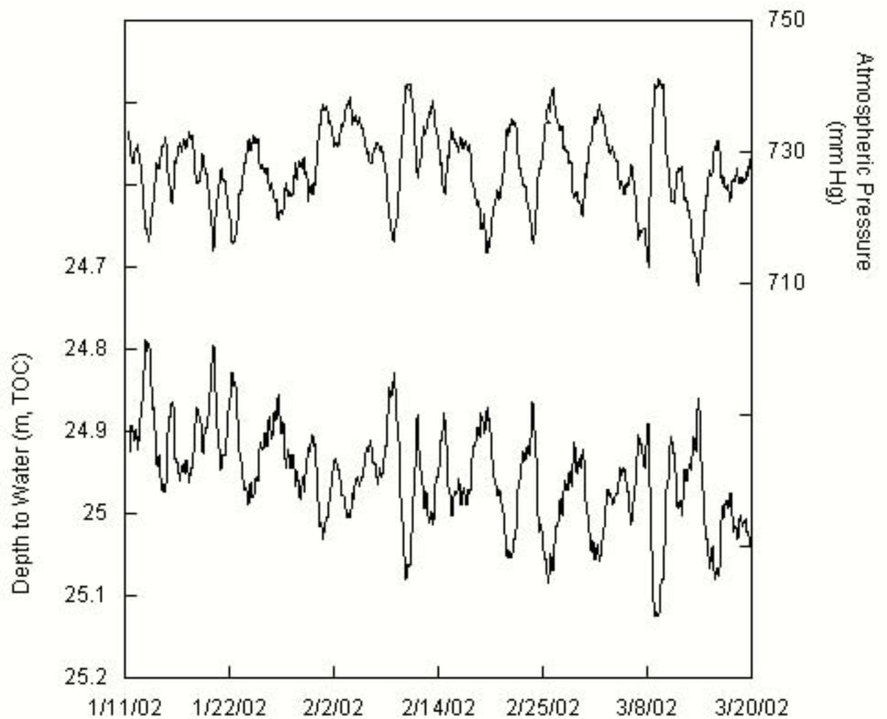
Figure 41. January-March 2002 monitoring well hydrograph with the record of atmospheric pressure fluctuations measured at the Mid-Continent Airport, Wichita, Kansas.
