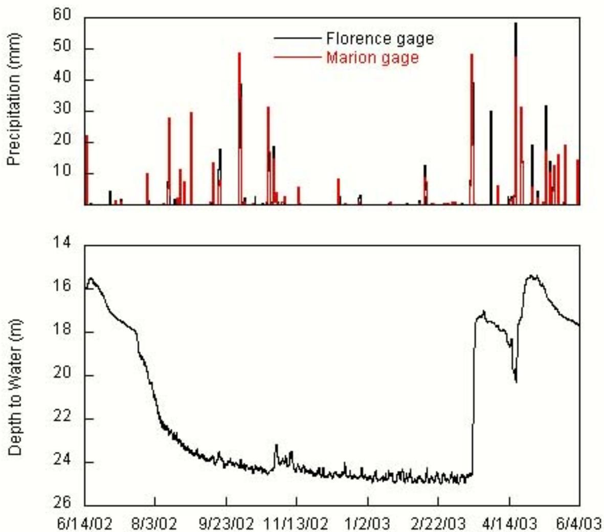
Figure 39. June 2002-June 2003 monitoring well hydrograph with precipitation for the period of record.
