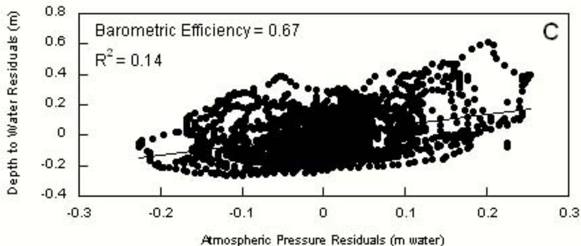
Figure 48. Scatterplots of the depth to water residuals vs atmospheric pressure residuals in m of water with a best-fit line from linear regression for the periods 1/11 - 3/20/2002 (A), 8/26 - 10/22/2002 (B), and 12/8/2002 - 3/13/2003 (C).
