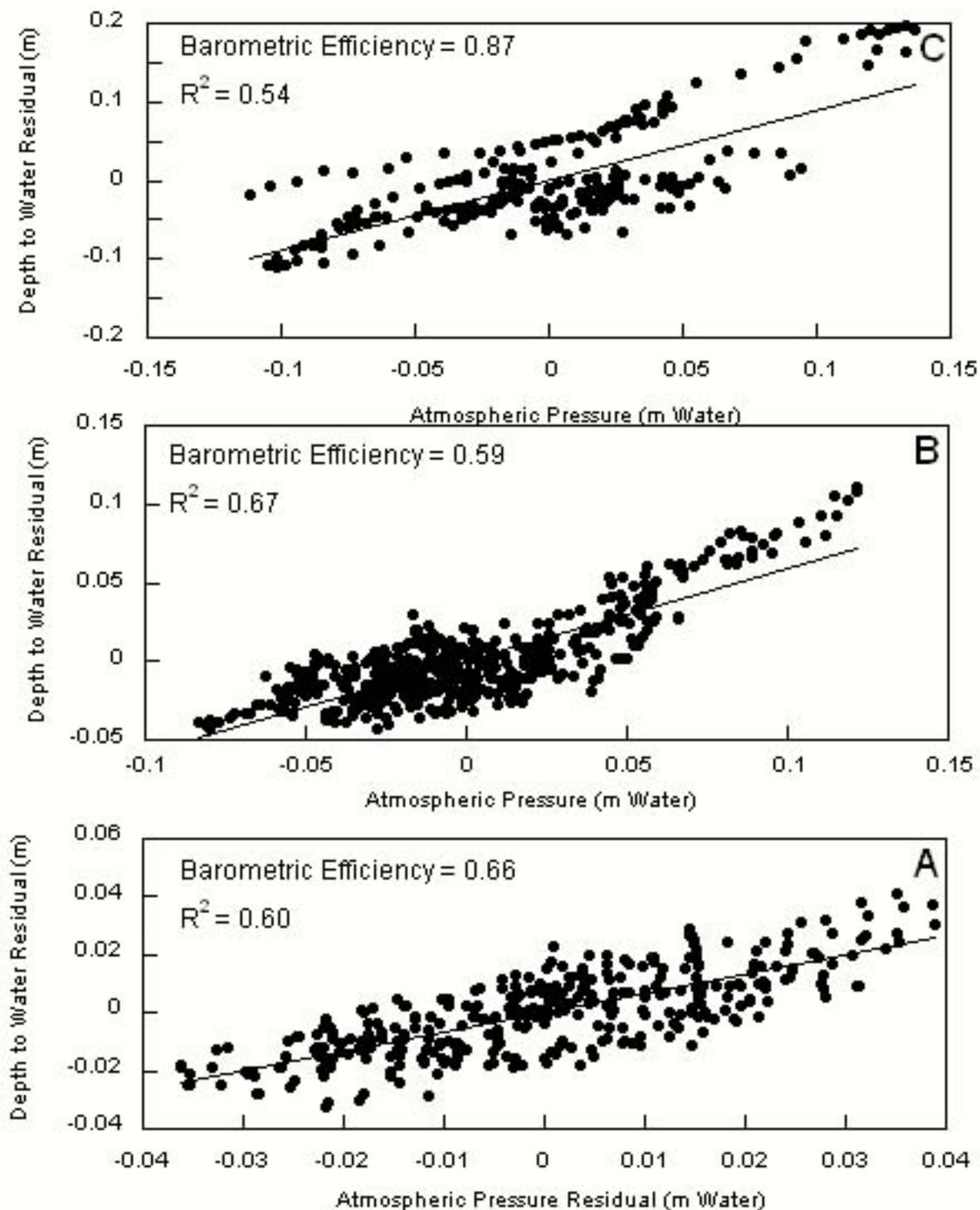
Figure 45. Scatterplots of the atmospheric pressure residuals in equivalent meters of water vs the depth to water residuals with a best-fit line through the points from linear regression for the periods 7/5 - 19/2002 (A), 5/21 - 6/11/2003 (B), and 5/10 - 19/2003 (C).
