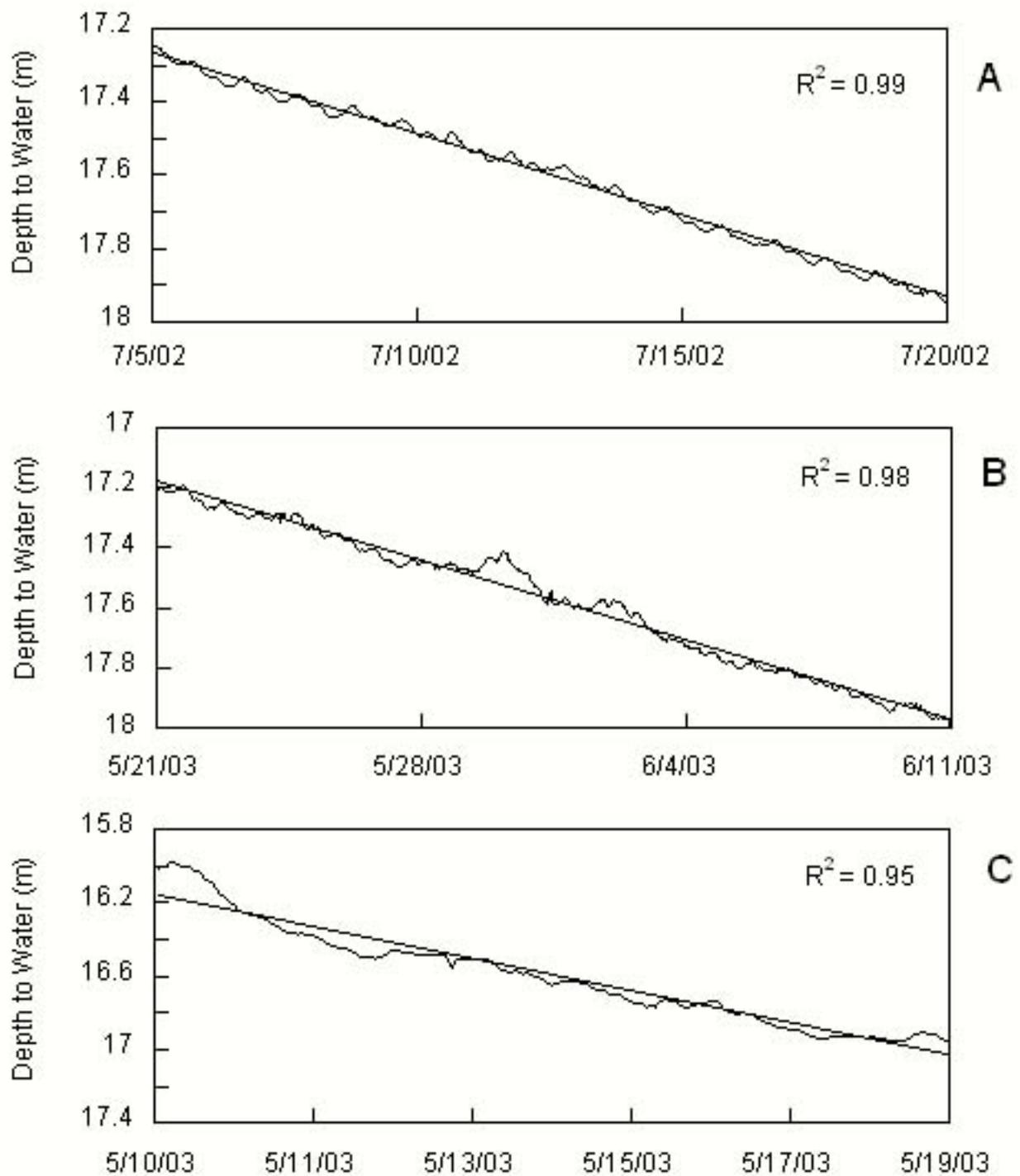
Figure 43. Trend lines from linear regression through the monitoring well hydrographs for 7/5-19/2002 (A), 5/21-6/11/2003 (B), and 5/10-19/2003 (C). All depth to water values are taken from the top of the well casing.
