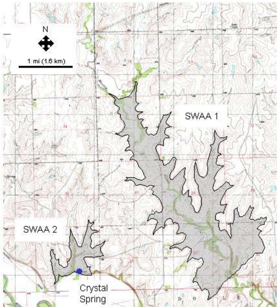
Figure 78. The Source Water Assessment Area (SWAA) for Crystal spring shown in a gray screen. The extent of the two SWAAs is defined by the outcropping Doyle Shale-Barneston Limestone contact and the approximate extent of the significant saturated thickness in the aquifer zones of the Barneston Limestone beneath Martin Creek.
