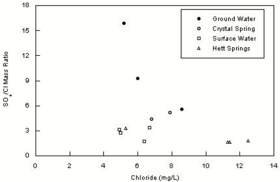
Figure 67. Dry season (August 2000 and Winter 2002) chloride and sulfate to chloride mass ratios for ground water, surface water, and spring samples.
