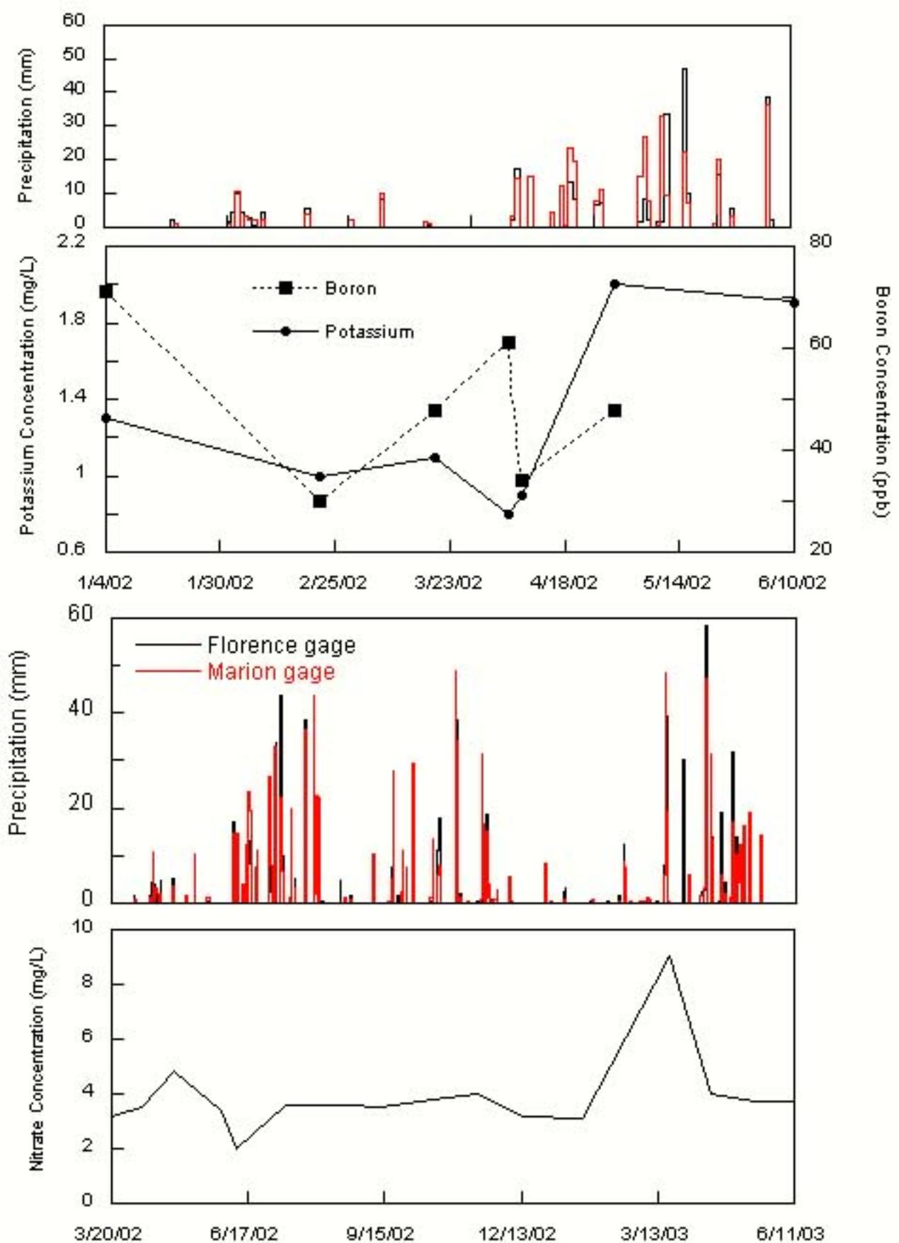
Figure 56. Time vs potassium, boron, and nitrate concentration also showing time distribution of precipitation at Marion (red) and Florence stream gages.
