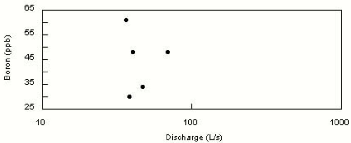
Figure 61. Discharge vs boron concentration for Crystal spring.
