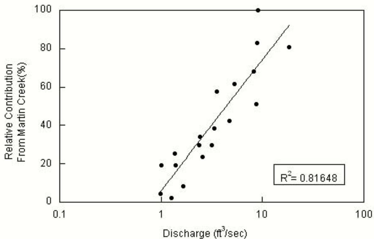
Figure 76. Scatterplot showing the percent of water from Martin Creek in the discharge from Crystal spring estimated from the chloride concentrations in spring discharge.
