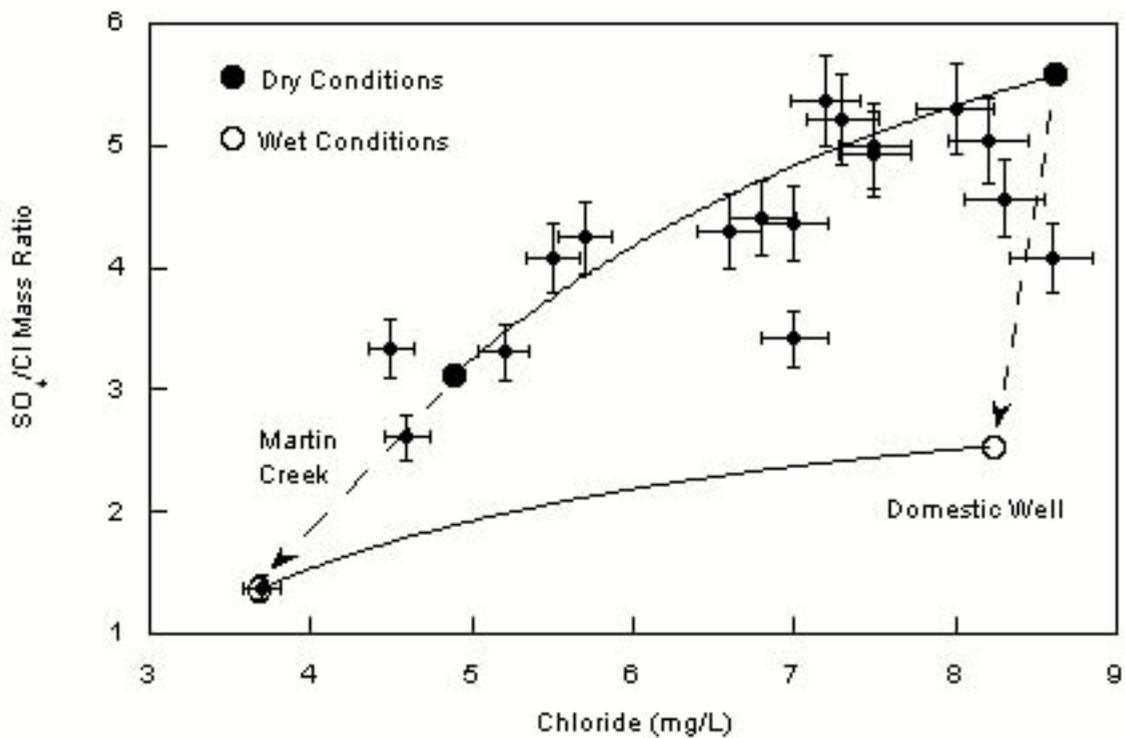
Figure 75. Geochemical mixing curves showing the mixing of surface water from Martin Creek with ground water from the Barneston aquifer in the discharge from Crystal spring using the chloride and sulfate to chloride mass ratios in the monthly samples with error bars.
