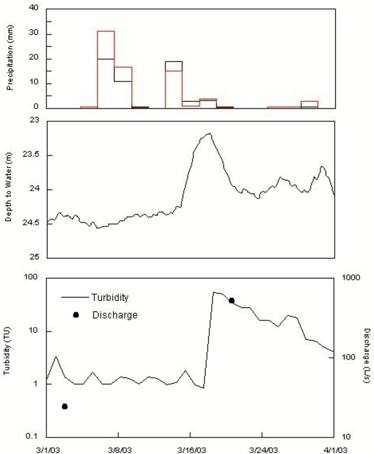
Figure 71. Precipitation, depth to water in the monitoring well, and turbidity in the discharge from Crystal spring for the period October 20 - November 6, 2002. Precipitation data are from the Marion (red) and Florence (black) stream gages on the Cottonwood River.
