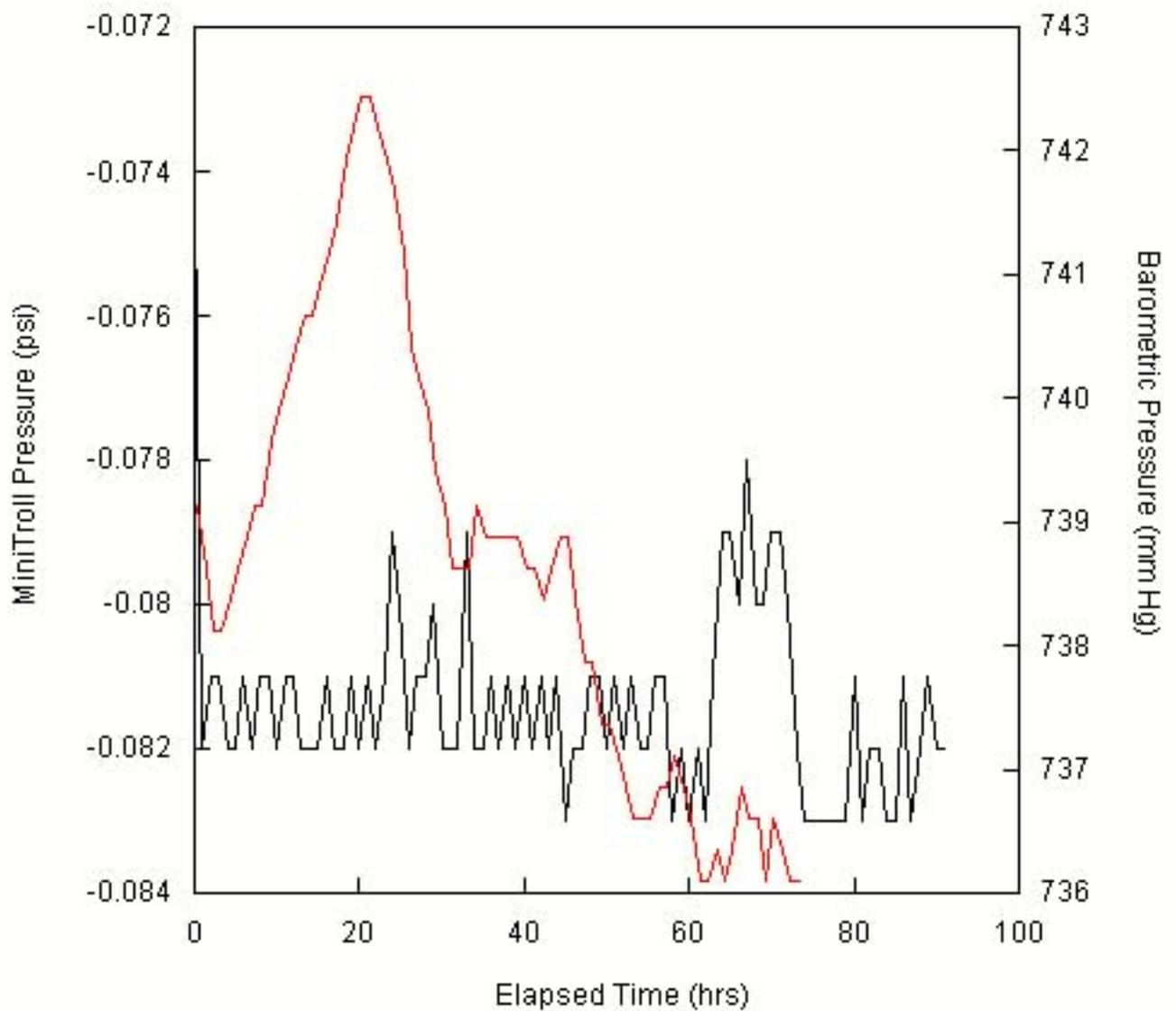
Figure 49. Elapsed time vs MiniTroll pressure (black) and atmospheric pressure (red) measured at the Municipal Airport, Lawrence, Kansas.
