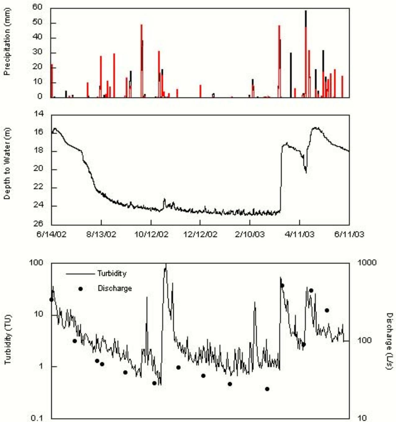
Figure 66. Time vs depth to water in the monitoring well, Crystal spring discharge and turbidity, and precipitation at the Marion (red) and Florence (black) stream gages on the Cottonwood River.
