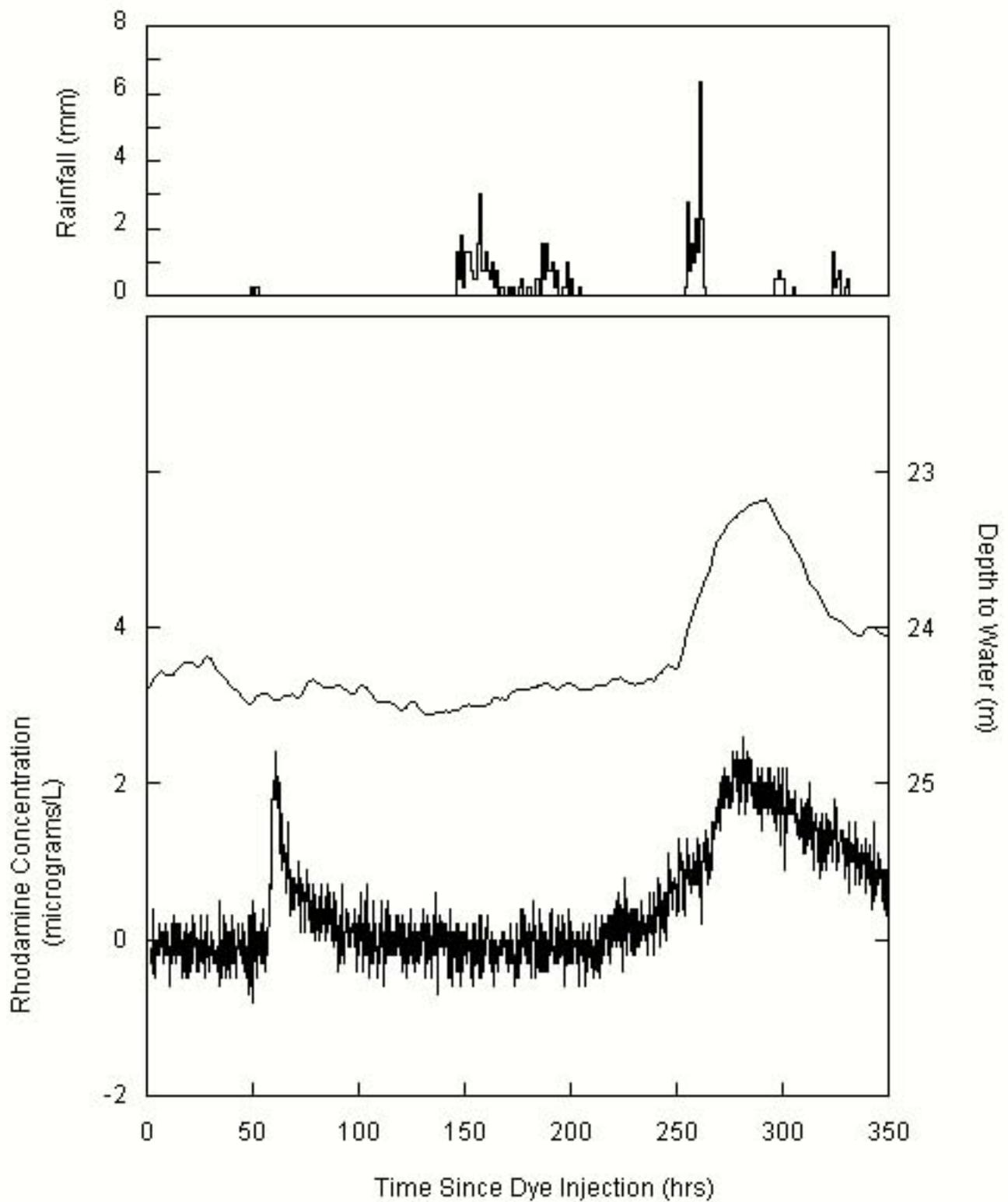
Figure 37. Time vs rhodamine-WT concentration in the discharge from Crystal spring and monitoring well depth to water.
