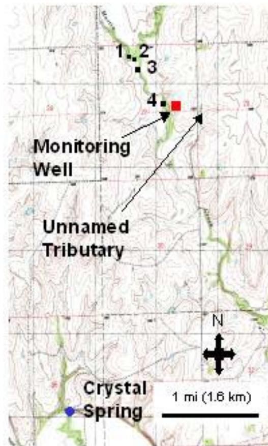
Figure 31. Location of the monitoring well with respect to the sinkholes in Martin Creek, an unnamed tributary east of the creek, and Crystal spring. The monitoring well is approximately 215 m east of Martin Creek and 400 m west of the unnamed tributary.
