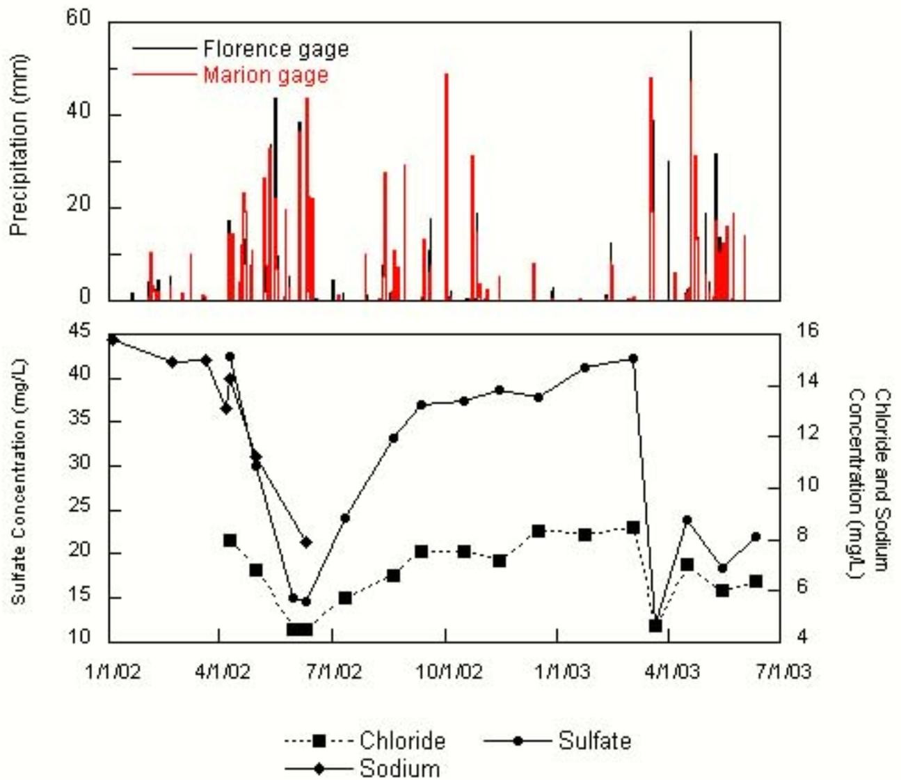
Figure 54. Time vs sodium, sulfate, and chloride concentration also showing time distribution of precipitation at Marion (red) and Florence stream gages.
