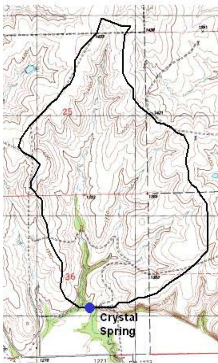
Figure 77. Extent of the unnamed drainage west of Crystal spring. The lower part of the drainage crosses the outcrop of the lower Ft. Riley Limestone and may contribute to the discharge from the spring.
