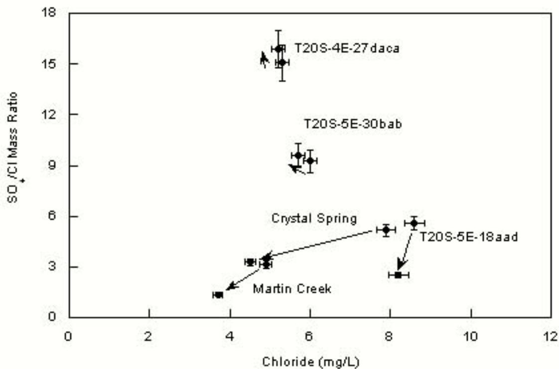
Figure 69. Changes in chloride and the sulfate to chloride mass ratio in ground water, Martin Creek surface water, and Crystal spring discharge between the Winter 2002 and Spring 2002 water sampling events. Also shown are the error bars associated with each parameter.
