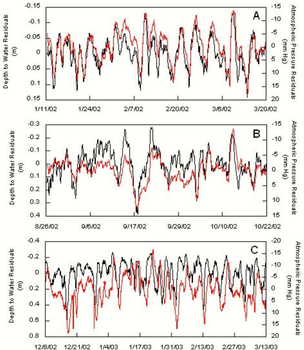
Figure 47. Time vs depth to water (black) and atmospheric pressure residuals (red) from linear regression for the periods 1/11 - 3/20/2002 (A), 8/26 - 10/22/2002 (B), and 12/8/2002 - 3/13/2003 (C).
