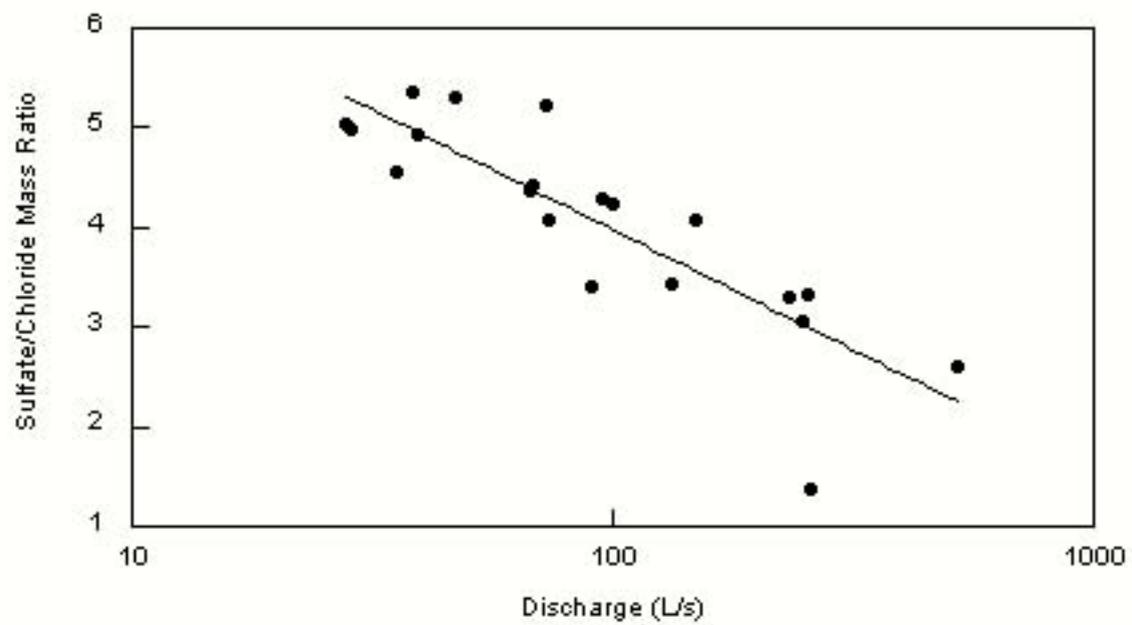
Figure 58. Discharge vs the sulfate/chloride mass ratio for Crystal spring.
