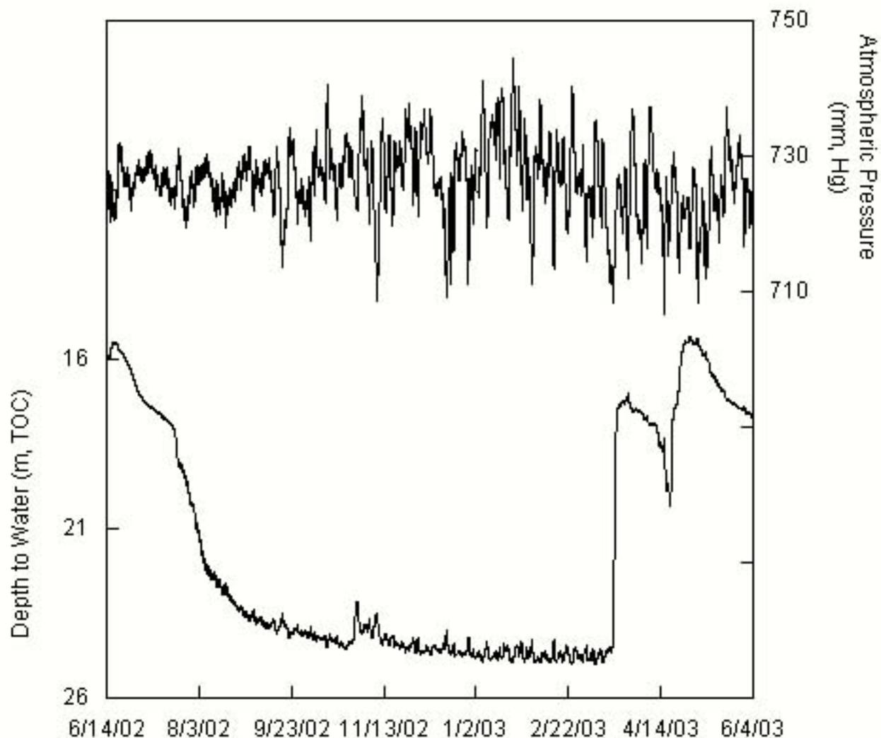
Figure 42. June 2002-June 2003 monitoring well hydrograph with the record of atmospheric pressure fluctuations measured at the Mid-Continent Airport, Wichita, Kansas. Depth to water is measured from the top of the well casing (TOC).
