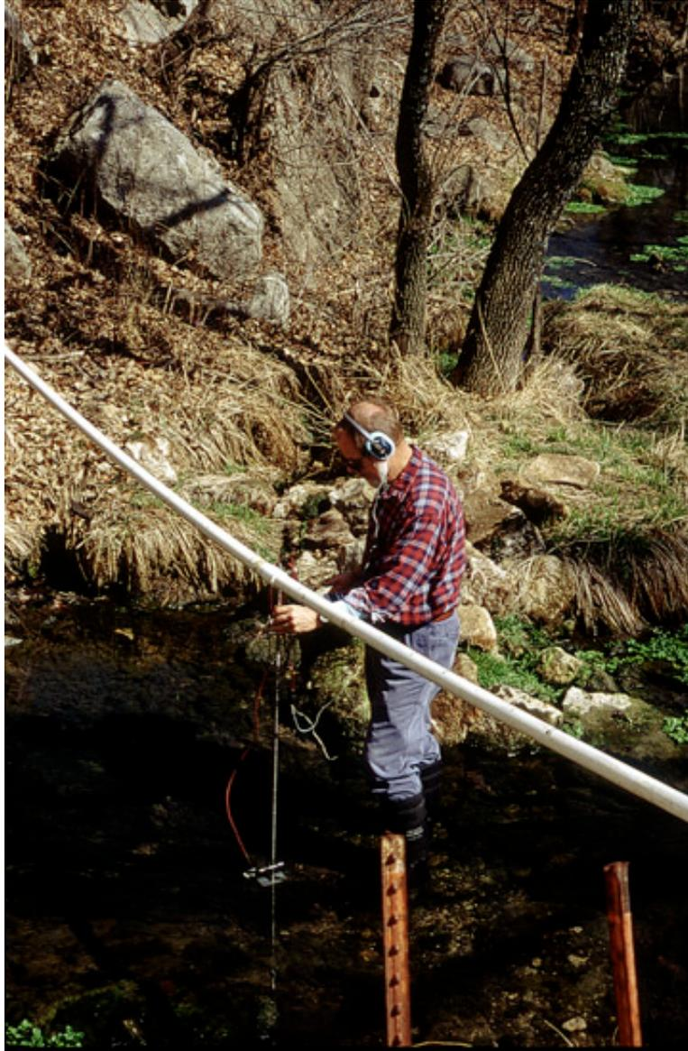
Figure 28. Spring discharge measurements at Crystal spring. Flow velocities and discharge pool depths were measured at points marked on the PVC plastic pipe and used to calculate spring discharge. Measurements were made using a Teledyne Gurley No. 625F pygmy current meter.
