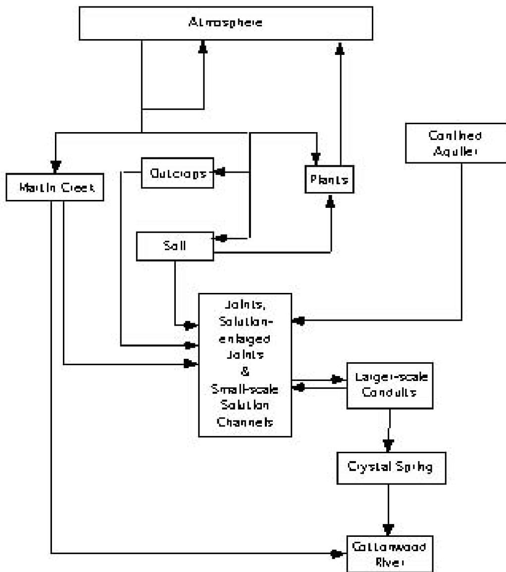
Figure 73. Schematic of a preliminary conceptual model showing the movement of water through the Crystal spring catchment to the Cottonwood River.
