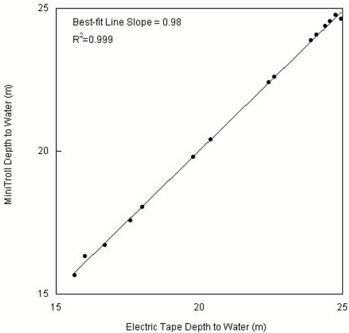
Figure 33. Depth-to-water measurements taken with the MiniTroll compared to measurements taken manually at the same time.
