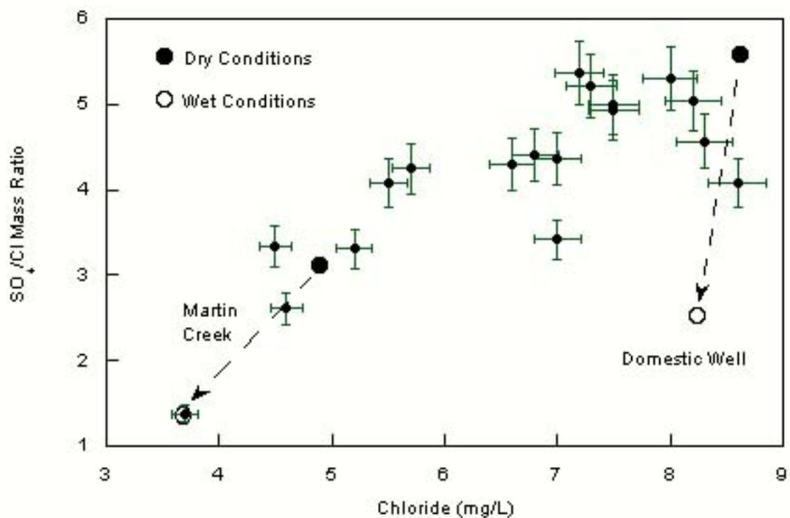
Figure 74. Changes in chloride and the sulfate to chloride mass ratio in the monthly samples of the discharge from Crystal spring with respect to the changes in these parameters in Martin Creek surface water and ground water between the Winter 2002 and Spring 2002 water sampling events.
