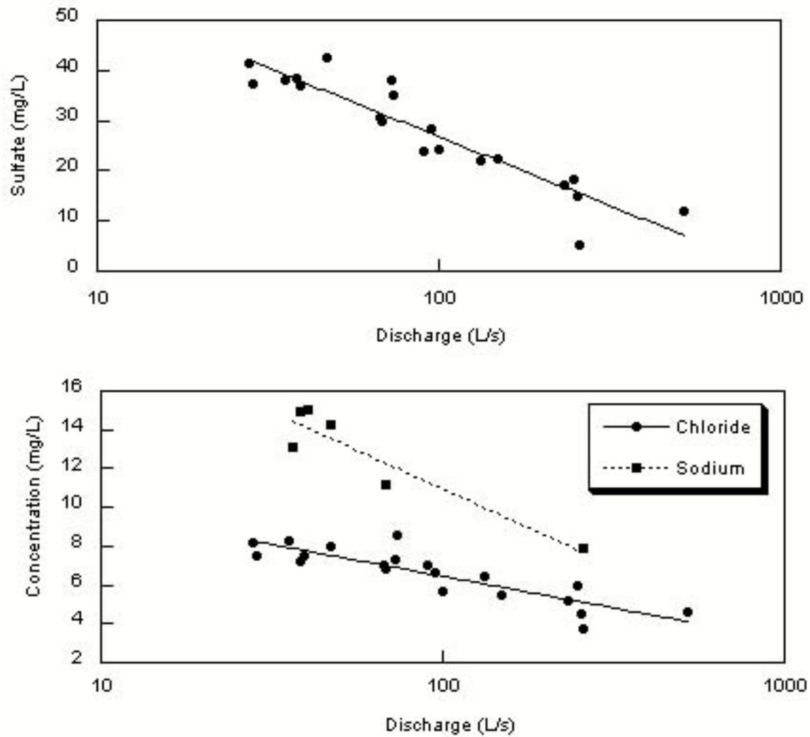
Figure 57. Discharge vs sulfate, chloride, and sodium concentration for Crystal spring.
