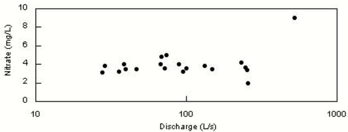
Figure 60. Discharge vs nitrate concentration for Crystal spring.
