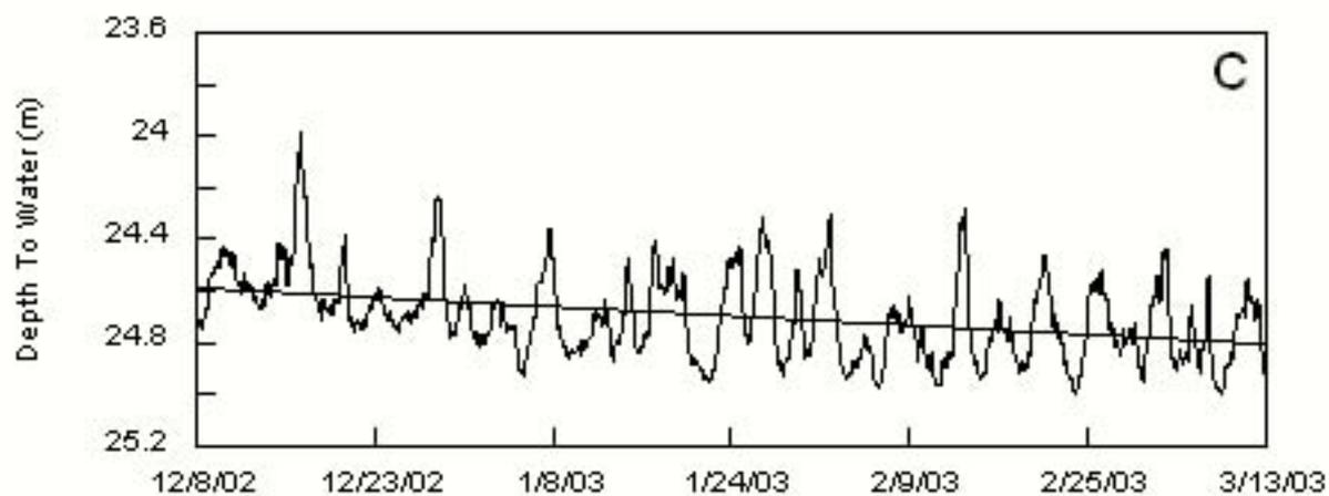
Figure 46. Time vs depth to water with trend lines from linear regression for the periods 1/11 - 3/20/2002 (A), 8/26 - 10/22/2003 (B), and 12/8/2002 - 3/13/2003 (C).
