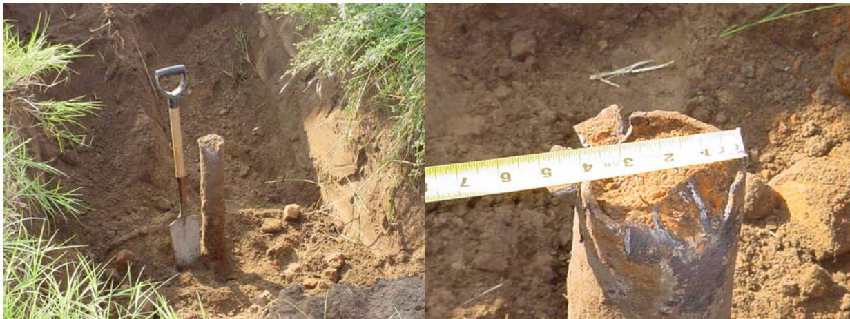
Figure 16. The total field component of the magnetic anomaly in grid I10 at the Ironhorse Equestrian Center site (top). The anomaly at (92, 62) is due to a suspected brine well (4-inch) at a depth of 2 ft (bottom). We dug down 4 ft to make sure it was not just a junk pipe.
