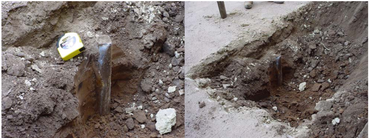
Figure 18. The total field component of the magnetic anomaly in grid T10 at the Trailer Park site (top). The anomaly at (10, 90) is due to a suspected brine well (2.5-inch) at a depth of 1 ft under a gravel pavement road (bottom). A 30' tape measure (3.5 inches tall) is shown for scale. We dug down 2.5 ft to make sure this was not just a junk pipe.
