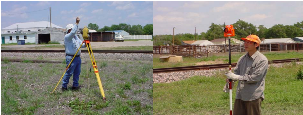
Figure 1b. A theodolite was used to define grids for high-resolution magnetic survey. David Laflen (left) and Gang Tian (right) are defining grids.
