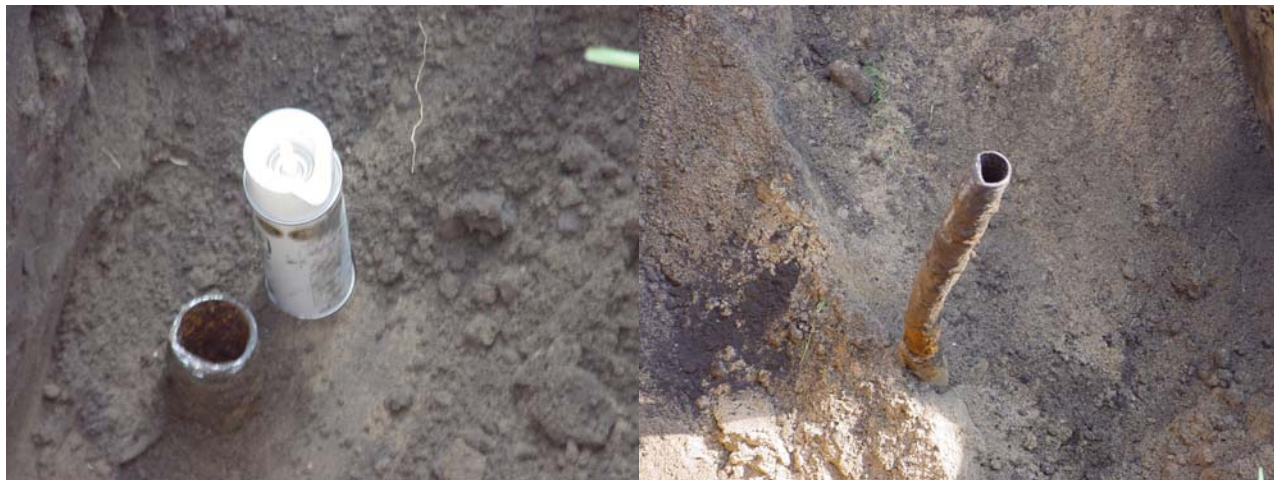
Figure 14. The total field component of the magnetic anomaly in grid U2 at the Union Salt site (top). The anomaly at (76, 55) is due to a suspected brine well (2.5-inch) at a depth of 4 ft (bottom). A spray paint can is shown for scale. We dug up to 7 ft deep to make sure it was not just a junk pipe.
