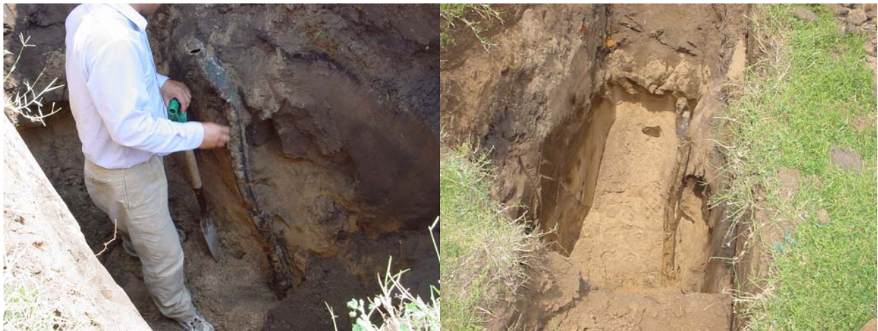
Figure 15. The total field component of the magnetic anomaly in grid S4 of at the Salvation Army Eagle Park site (top). The anomaly at (23, 55) is due to a suspected brine well (2.5-inch) at a depth of 2 ft (bottom). We dug up to 7 ft deep to make sure it was not just a junk pipe. Xia is checking the depth.
