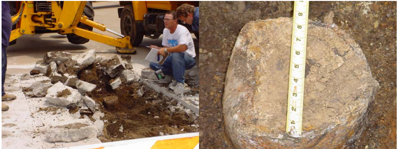
Figure 7. The total field component of the magnetic anomaly in grid U5 at the Union Salt site (top). The anomaly at (42, 23) is due to a brine well under 6 inches of concrete. Depth to the top of the well is 1 ft (bottom). Richard Harper of Kansas Department of Health & Environment is taking a note.
