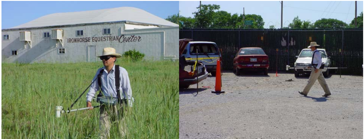
Figure 1a. A portable cesium magnetometer G858 was used to measure the total component of the geomagnetic field. Xia is performing the magnetic survey.
