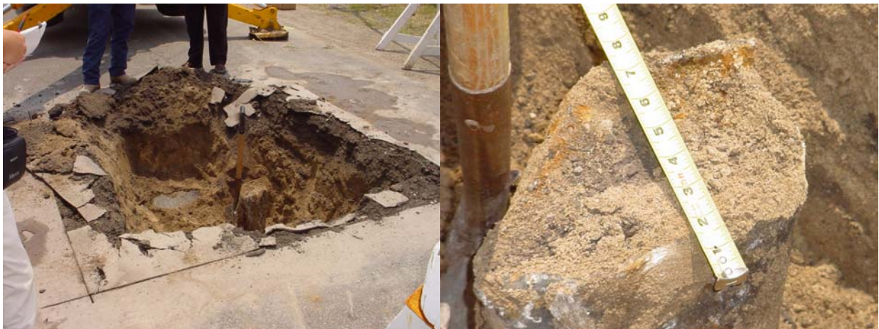
Figure 13. The total field component of the magnetic anomaly in grid M3 at Monroe & Avenues E and F (top). The anomaly at (62, 90) is due to a brine well at a depth of 2 ft under 1 ft of asphalt pavement (bottom).
