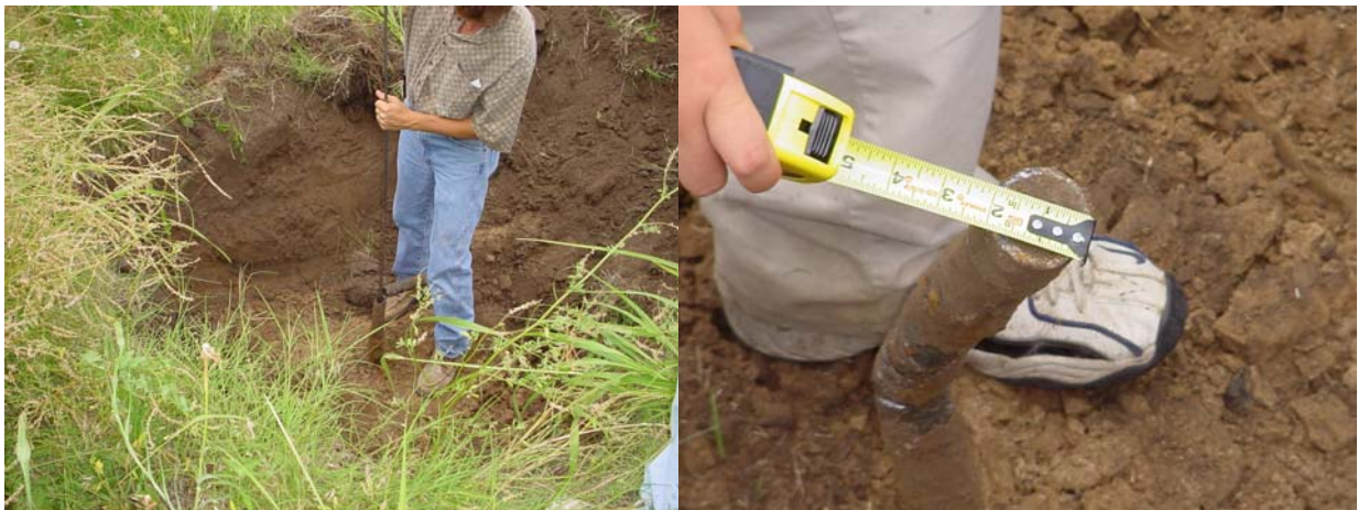
Figure 20. The total field component of the magnetic anomaly in grid C at the Chemical & 8 th Street site (top). The anomaly at (50, 123) is due to a probable water well (1.5-inch) at a depth of 1 ft (bottom). We dug down 4 ft to make sure this was not just a junk pipe. Kyle Parker (bottom left) of Kansas Department of Health and Environment is checking the well and Sihao Xia (bottom right) is measuring the diameter of the well.
