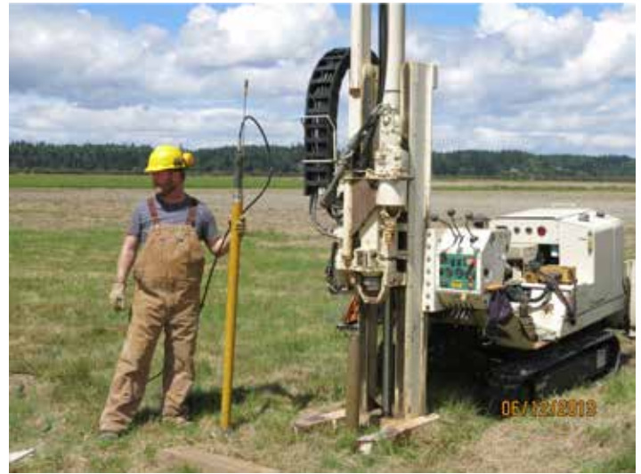
A KGS research assistant operates a Geoprobe direct-push rig as part of a DOE-funded project to assess the potential of nuclear magnetic resonance technology for shallow groundwater applications.
