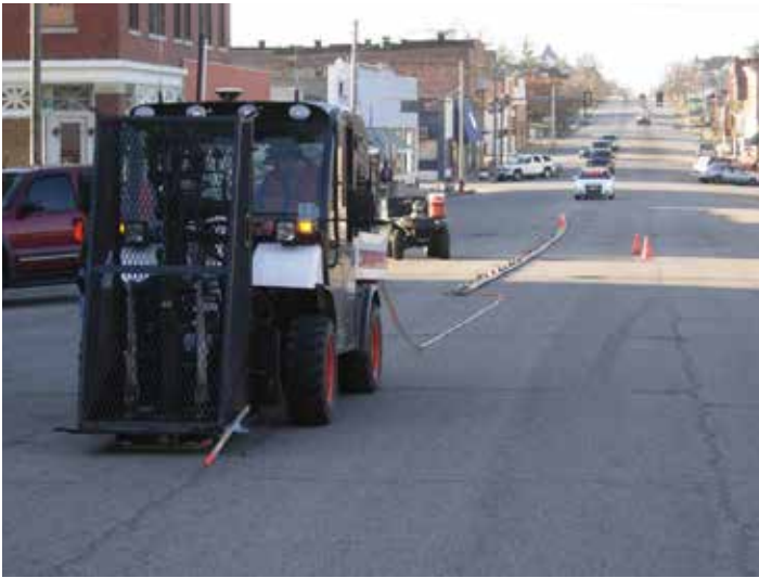
A bungee-assisted weight drop attached to the front of a Bobcat Toolcat (shown here in Galena, Kansas) is one example of active seismic sources used by scientists at the KGS.
