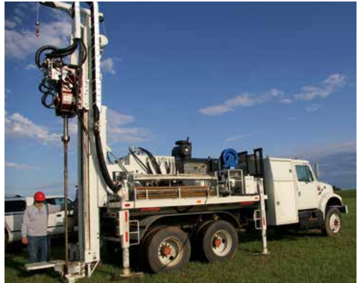
The S-27 RotoSonic drill rig, one of the three deep penetrating drill rigs operated by the Exploration Services section of the KGS.
