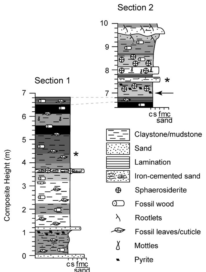
**Figure 1.** Two overlapping stratigraphic sections were combined in this study of Rose Creek Pit (RCP), Nebraska. Stars represent sample positions for palynological analysis. Arrow points to the  $D_2$  sequence boundary identified by this study in carbon isotopes; c—clay, s—silt, fmc—fine, medium, and coarse sand.
