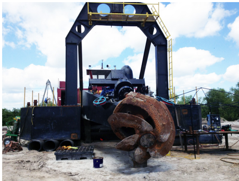
Figure 5—Cutter head on sediment dredge. Photo: Great Lakes Dredge and Dock Company.
