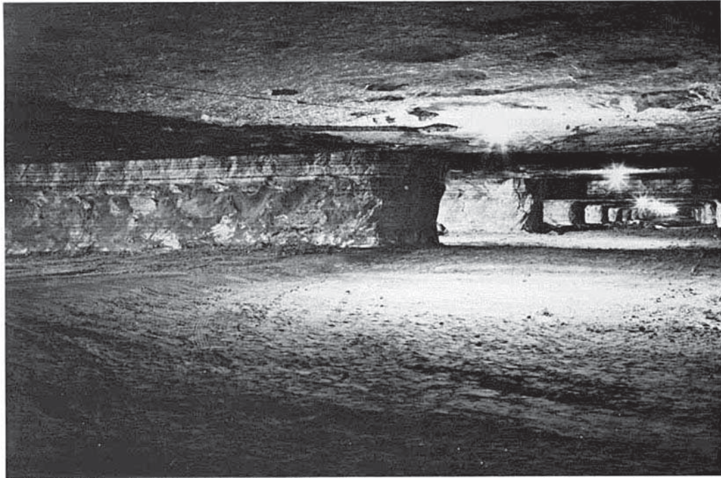
Figure 4–10. Carey Salt Company mine, Hutchinson, Kansas, showing light and dark banding in the Hutchinson Salt Member (from Walters, 1978). Photograph courtesy of Underground Vaults and Storage, Inc.
