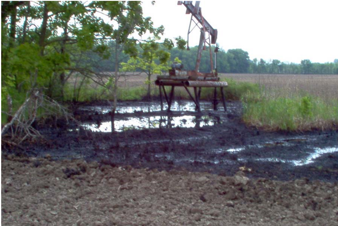
Figure 5-1. Abandoned well leaking saltwater, Verdigris River floodplain, Montgomery County, KS (photo by KCC).
