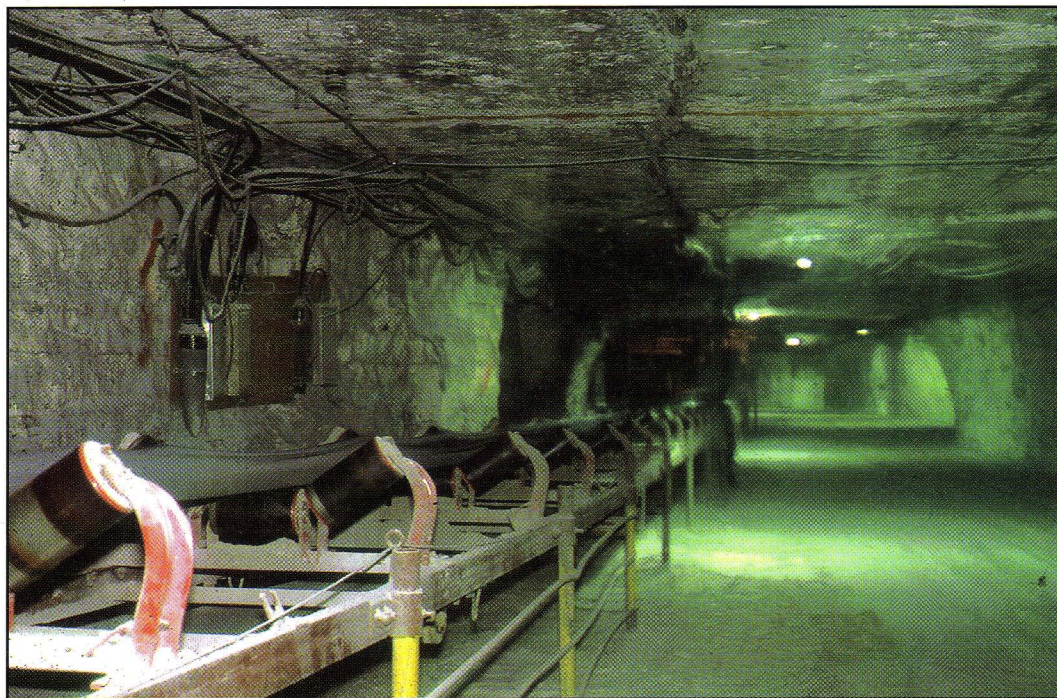
Figure 5—Underground salt mine at Hutchinson. Salt is mined in a room-and-pillar fashion, and moved along a conveyor belt and eventually to the surface.
