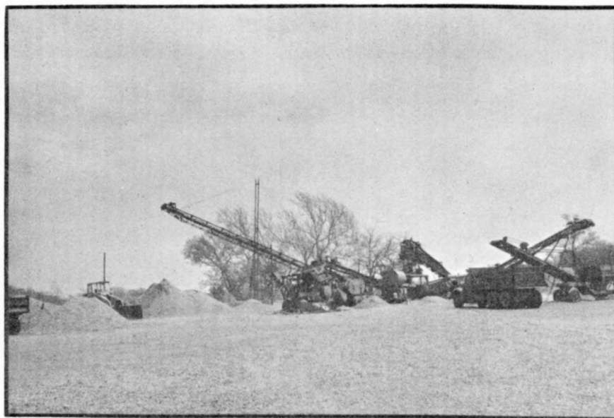
Figure 15. Alluvial chert gravel in a pit along Little Hickory Creek where the raw material is crushed, sorted, and washed, N \frac{1}{2} sec. 14, T28S, R6E.
