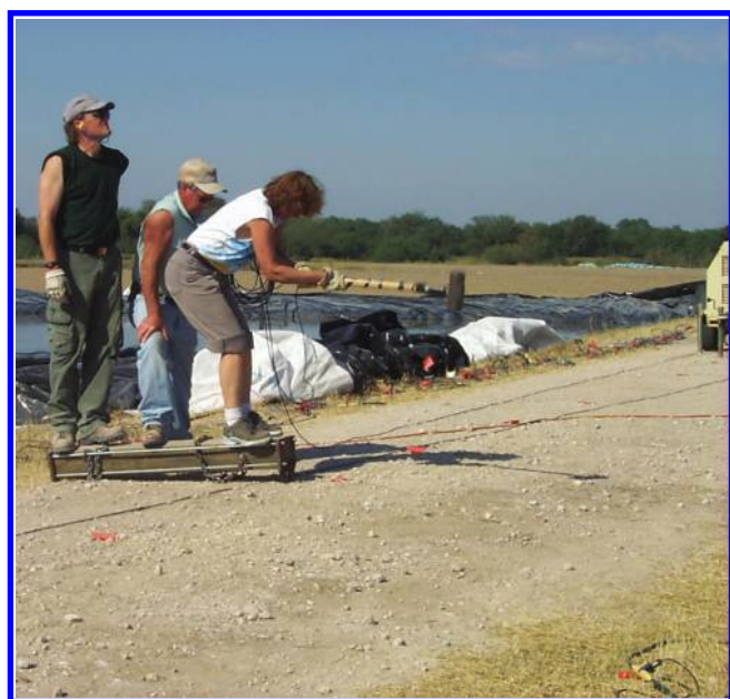
Figure 5. Shear-wave source operated along the crest at site 2.
