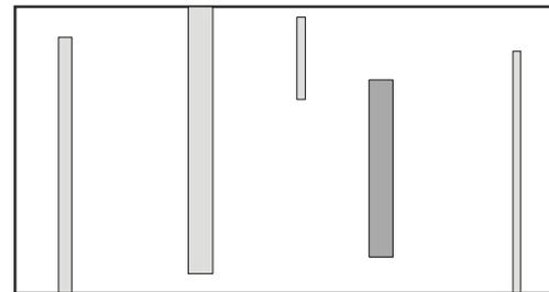
4) *Discontinuous series network ( $N_{s,d}$ )* - preferential non-sample-spanning orientation of pore sizes or beds of different  $N_p$  networks perpendicular to the invasion direction. Represents continuum between  $N$  and  $N_p$ .
