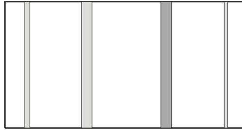
3) *Series network ( $N_s$ )* - preferential sample-spanning orientation of pore sizes or beds of different  $N_p$  networks perpendicular to the invasion direction.
