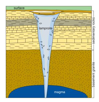
Fig. 6—Generalized diagram of a lamproite pipe.
