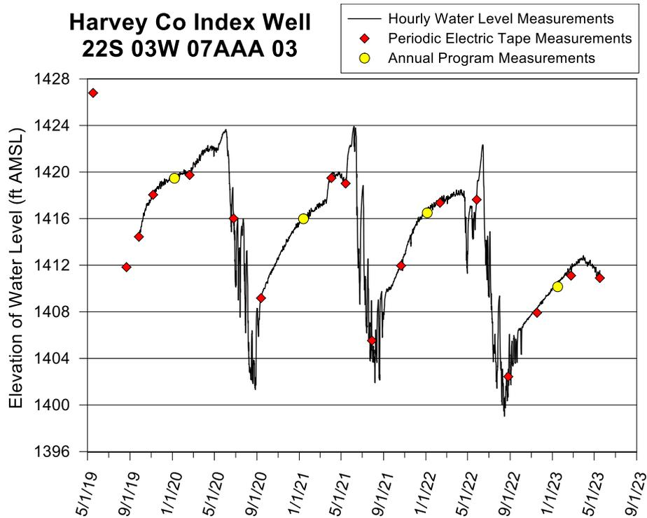
Figure 10—Harvey County index well hydrograph—total data run to 5/17/23. A water-level elevation of 1,416 ft corresponds to a depth to water of 39 ft below Isf. The top of the 10 ft screen is 198 ft below Isf (elevation of 1,257 ft), and the bottom of the aquifer is 206 ft below Isf (elevation of 1,249 ft).
