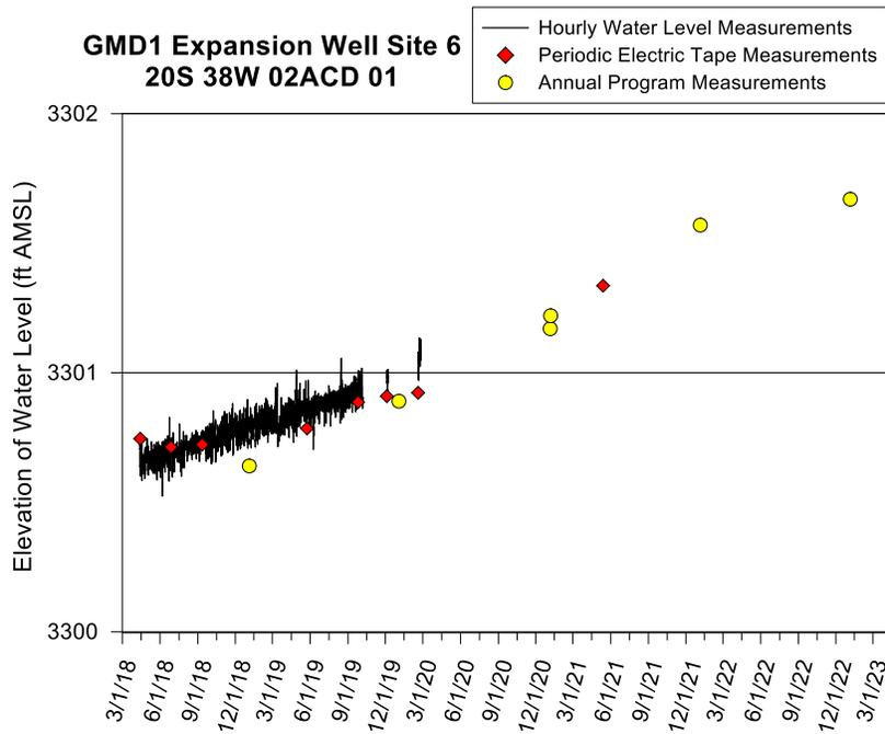
Figure 48—GMD1 Expansion Site 6 well hydrograph—total data run to 1/5/23; continuous hourly measurements ended on 10/6/19. A water-level elevation of 3,301 ft corresponds to a depth to water of 104 ft below lsf. Elevation of well bottom is not known. Bottom of aquifer is at an elevation of 3,221 ft (184 ft below lsf).
