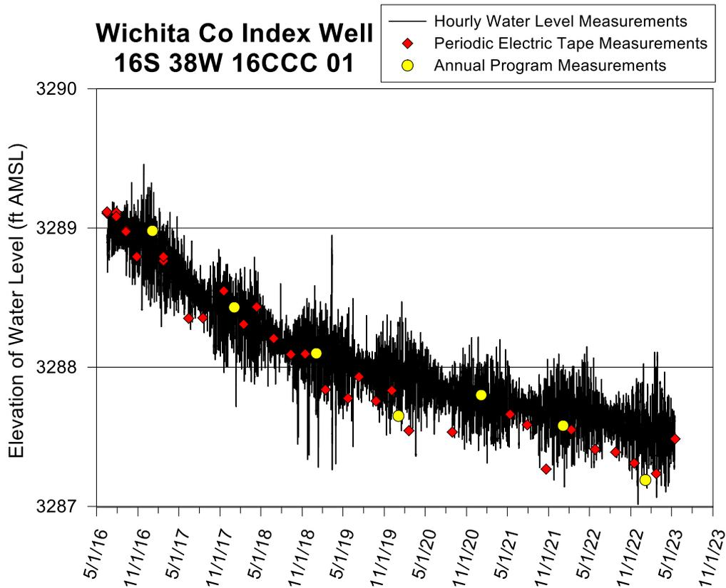
Figure 6—Wichita County index well hydrograph—total data run to 5/16/23. A water-level elevation of 3,288 ft corresponds to a depth to water of 160 ft below lsf. The top of the screen is 175 ft below lsf (elevation of 3,273 ft), and the bottom of the aquifer is 190 ft below lsf (elevation of 3,258 ft). The screen terminates 5 ft above the bottom of the aquifer.
