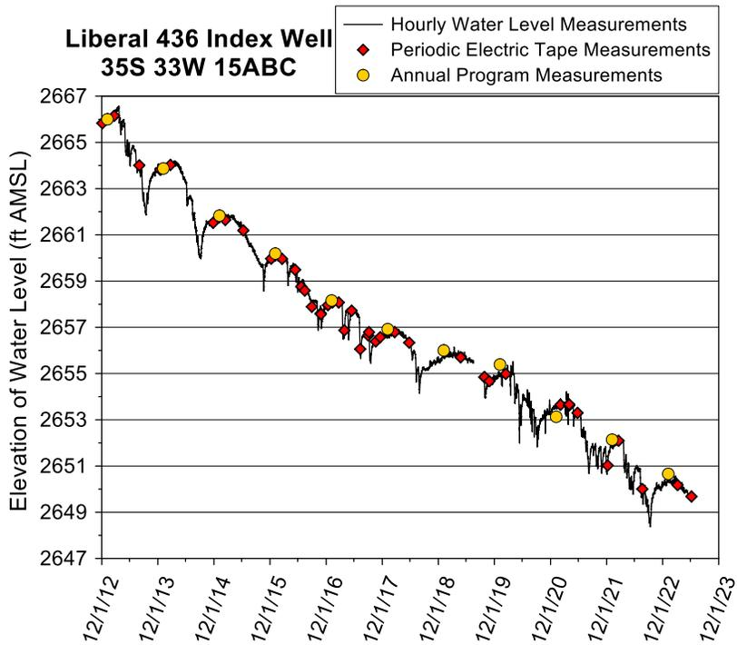
Figure 19—Hydrograph of Liberal 436 index well—total data run to 6/6/23. A water-level elevation of 2,651 ft corresponds to a depth to water of 170 ft below lsf. The top of the 10 ft screen is 426 ft below lsf (elevation of 2,395 ft). Sensor failed on July 6, 2019; a new sensor was installed on September 27, 2019.
