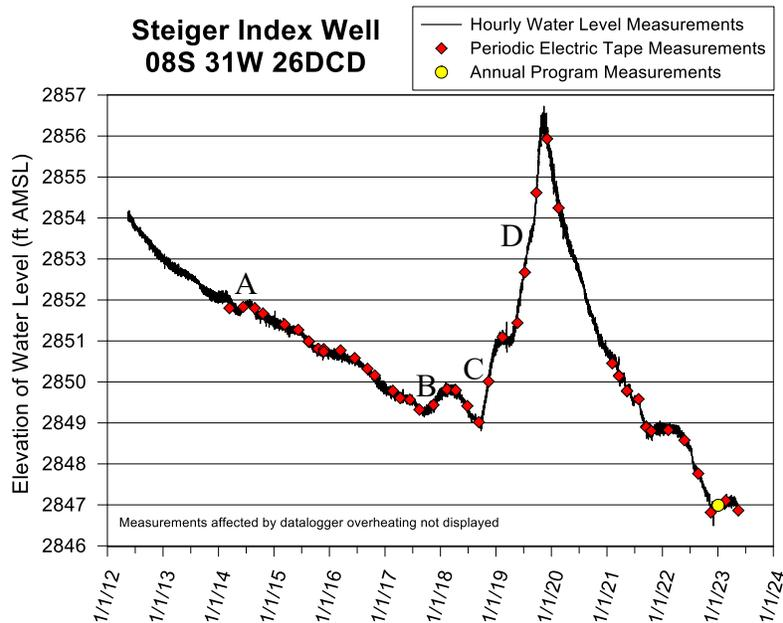
Figure 32—Steiger index well hydrograph—total data run to 5/15/23. A water-level elevation of 2,850 ft corresponds to a depth to water of 115 ft below Isf. The top of the 40 ft screen is 145 ft below Isf (elevation of 2,820 ft), and the bottom of the aquifer is 177 ft below Isf (elevation of 2,788 ft). A–D defined in text.
