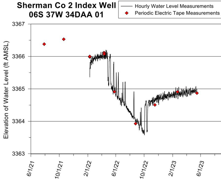
Figure 34—Sherman County 2 index well hydrograph—total data run to 5/16/23. A water-level elevation of 3,365 ft corresponds to a depth to water of 159 ft below Isf. The top of the 40 ft screen is 240 ft below Isf (elevation of 3,284 ft). The bottom of the aquifer is estimated to be 275 ft below Isf (elevation of 3,249 ft), and the bottom of the well is 276.3 ft below Isf (well appears to have 3.7 ft of material in the bottom – lower 5 ft of screen appear to be below the bottom of the aquifer).
