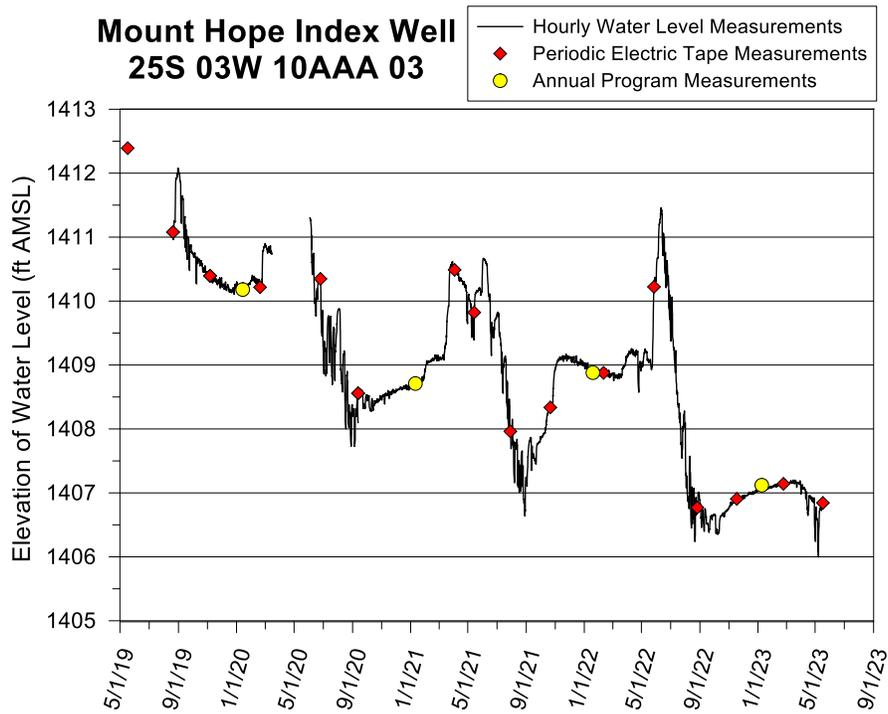
Figure 12—Mount Hope index well hydrograph—total data run to 5/17/23. A water-level elevation of 1,410 ft corresponds to a depth to water of 11.4 ft below Isf. The top of the 10 ft screen is 163 ft below Isf (elevation of 1,258.4 ft), and the bottom of the aquifer is 173 ft below Isf (elevation of 1,248.4 ft). Sensor failure produced the break in monitoring from 3/15/20 to 6/3/20.
