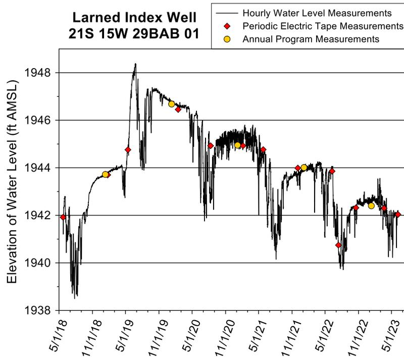
Figure 38—Larned index well hydrograph—total data run to 6/5/23. A water-level elevation of 1,944 ft corresponds to a depth to water of 11.3 ft below Isf. The top of the 5 ft screen is 66 ft below Isf (elevation of 1,889.3 ft), and the bottom of the screen, which is at the base of the aquifer, is 71 ft below Isf (elevation of 1,884.3 ft).
