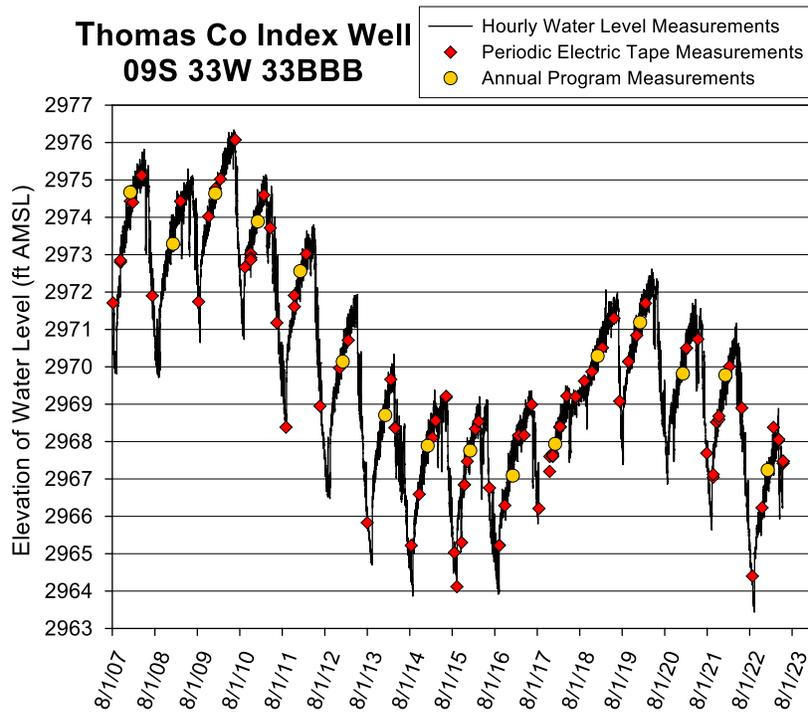
Figure 35—Thomas County index well hydrograph—total data run to 5/15/23. A water-level elevation of 2,967 ft corresponds to a depth to water of 220.6 ft below lsf. The top of the screen is 274 ft below lsf (elevation of 2,913.6 ft), and the bottom of the aquifer is 284 ft below lsf (elevation of 2,903.6 ft). The screen terminates at the bottom of the aquifer. No water-level data are available from 10/28/17 to 12/11/17 because of sensor failure.
