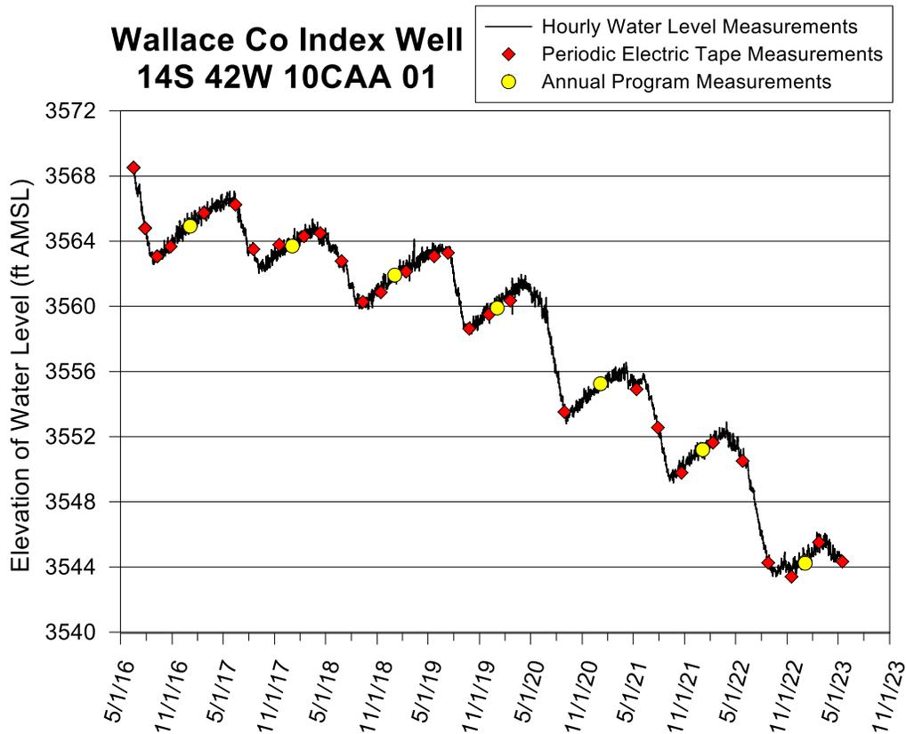
Figure 5—Wallace County index well hydrograph—total data run to 5/16/23. A water-level elevation of 3,544 ft corresponds to a depth to water of 284 ft below lsf. The top of the screen is 375 ft below lsf (elevation of 3,453 ft), and the bottom of the aquifer is 394 ft below lsf (elevation of 3,434 ft). The screen terminates 9 ft above the bottom of the aquifer.
