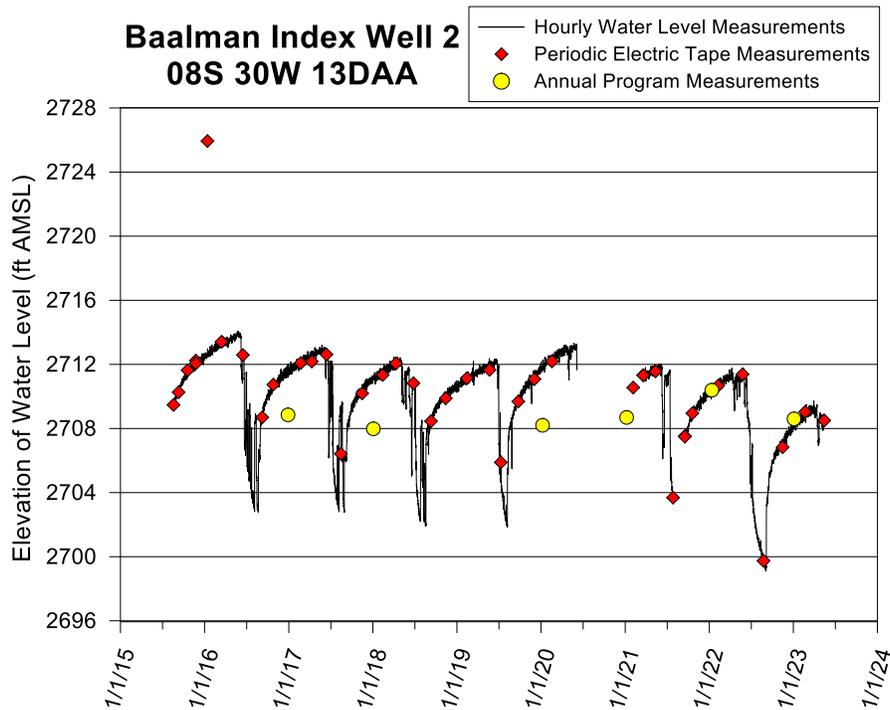
Figure 28—Baalman index well hydrograph—total data run to 5/15/23. A water-level elevation of 2,712 ft corresponds to a depth to water of 185 ft below Isf. The top of the 10 ft screen is 260 ft below Isf (elevation of 2,637 ft), and the bottom of the aquifer is 262 ft below Isf (elevation of 2,635 ft). The difference between the electric-tape and transducer measurements in January 2016 was caused by a malfunctioning electric tape.
