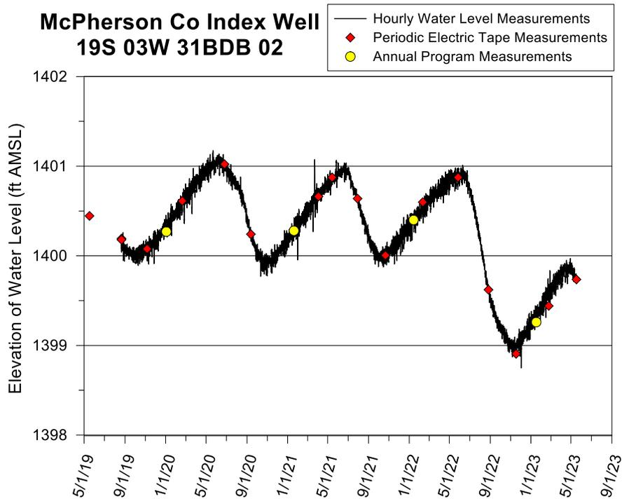
Figure 11—McPherson County index well hydrograph—total data run to 5/17/23. A water-level elevation of 1,400 ft corresponds to a depth to water of 94 ft below Isf. The top of the 44 ft screen is 139 ft below Isf (elevation of 1,355 ft), and the bottom of the screen is 183 ft below Isf (elevation of 1,311 ft). The bottom of the aquifer is 1 ft below the bottom of the screen (1,310 ft).
