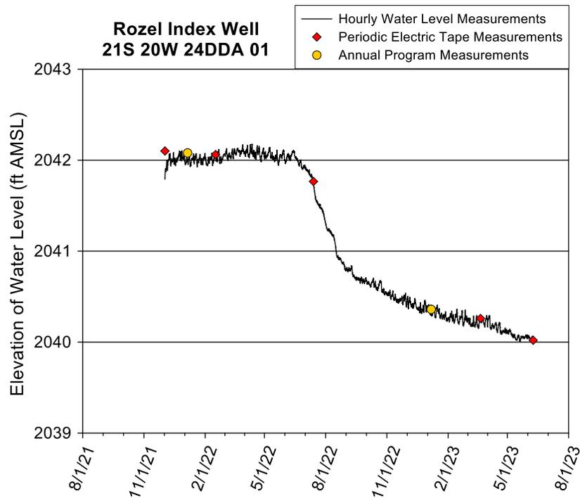
Figure 39—Rozel index well hydrograph—total data run to 6/8/23. A water-level elevation of 2,042 ft corresponds to a depth to water of 43 ft below lsf. There does not appear to have been a WWC5 form filed for this well so there are no well construction details. A camera survey found that the screen started at 40 ft below land surface and ended at a sand plug at 59 ft (elevation of 2,026 ft).
