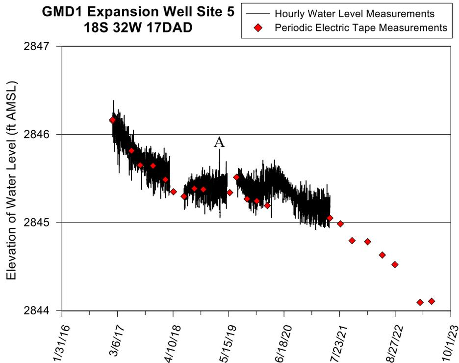
Figure 47—GMD1 Expansion Site 5 well hydrograph—total data run to 5/16/23. A water-level elevation of 2,845 ft corresponds to a depth to water of 131 ft below Isf. Elevation of well bottom is not known. A defined in text.
