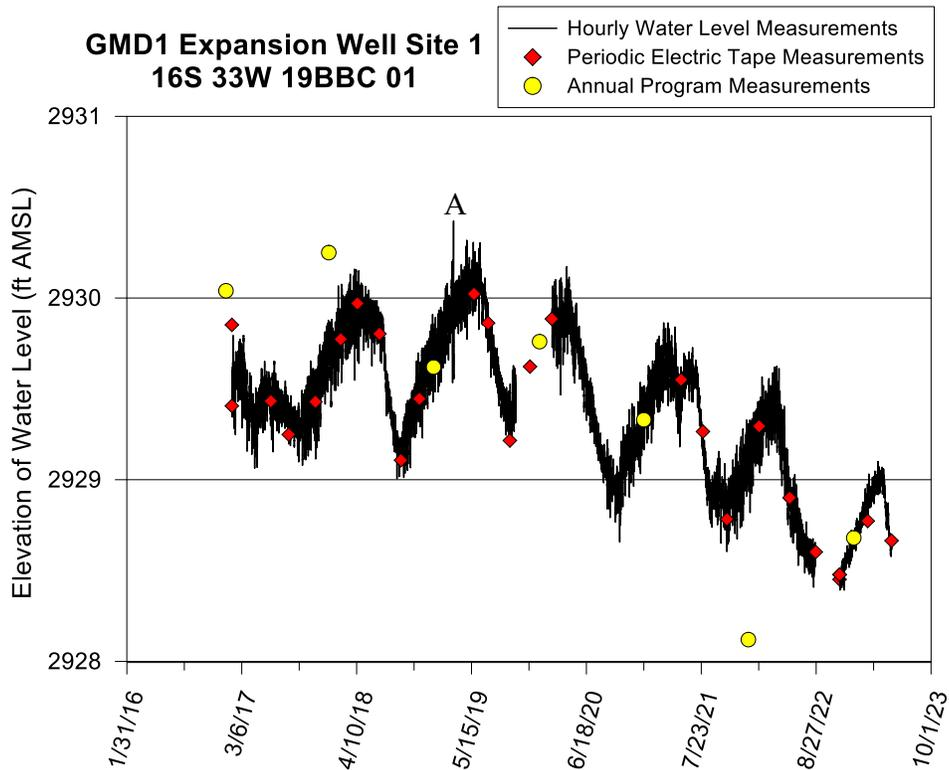
Figure 43—GMD1 Expansion Site 1 well hydrograph—total data run to 5/16/23. A water-level elevation of 2,930 ft corresponds to a depth to water of 168 ft below Isf. Bottom of well is 193.2 ft below Isf (elevation of 2,904.8 ft). A defined in text.
