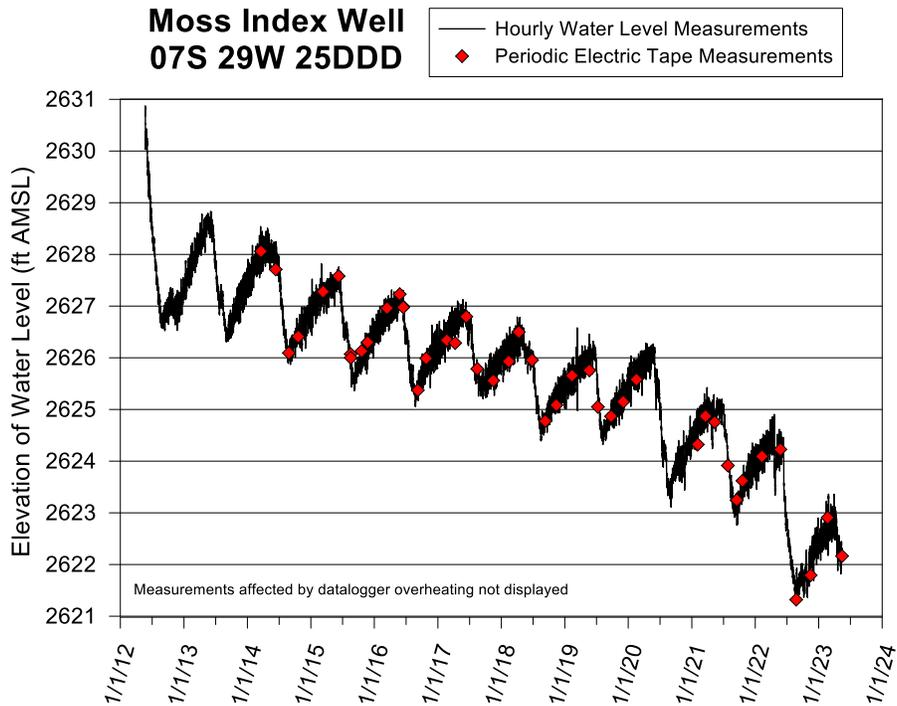
Figure 30—Moss index well hydrograph—total data run to 5/15/23. A water-level elevation of 2,625 ft corresponds to a depth to water of 191 ft below lsf. The top of the 40 ft screen is 205 ft below lsf (elevation of 2,611 ft), and the bottom of the aquifer is 243 ft below lsf (elevation of 2,573 ft).
