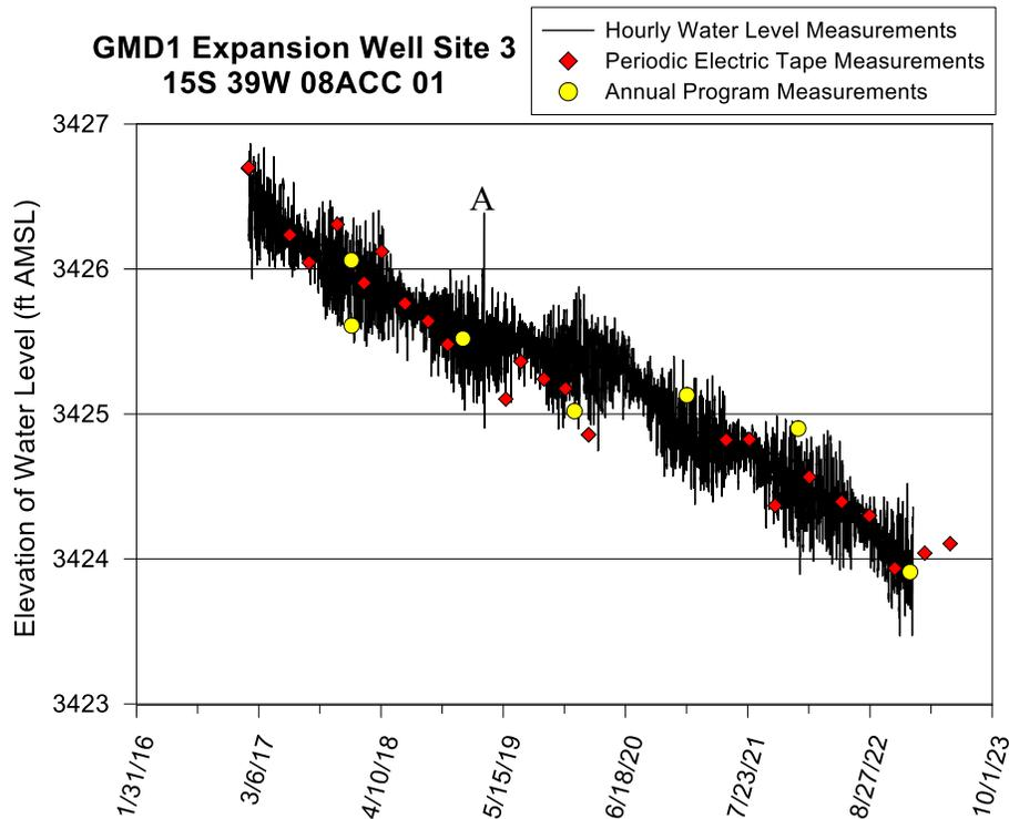
Figure 45—GMD1 Expansion Site 3 well hydrograph—total data run to 5/16/23. A water-level elevation of 3,426 ft corresponds to a depth to water of 197 ft below Isf. Bottom of well is 219.9 ft below Isf (elevation of 3,403.1 ft). A defined in text.
