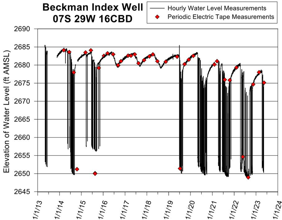
Figure 29—Beckman index well hydrograph—total data run to 5/15/23. A water-level elevation of 2,680 ft corresponds to a depth to water of 200.2 ft below lsf. The data gaps in 2013 and 2014 were caused by datalogger battery problems. The difference between the electric-tape measurement in the summer of 2015 and the hourly measurements from the transducer is thought to be caused by a change in transducer calibration specifications associated with the resumption of monitoring in late October 2014.
