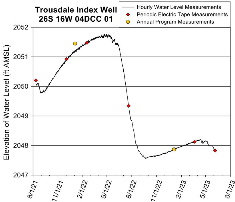
Figure 40—Trousdale index well hydrograph—total data run to 6/5/23. A water-level elevation of 2,051 ft corresponds to a depth to water of 33.8 ft below Isf. The top of the 10 ft screen is 47 ft below Isf (elevation of 2,037.8 ft). The bottom of the well is 57 ft below Isf (elevation of 2,027.8 ft); the base of the aquifer is at least 80 ft below the bottom of the well.
