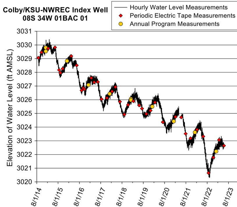
Figure 27—Colby index well hydrograph—total data run to 5/15/23. A water-level elevation of 3,024 ft corresponds to a depth to water of 153 ft below lsf. Total depth of the well is 175 ft below lsf (elevation of 3,002 ft). The screened interval extends from 156 to 175 ft below lsf. The base of the aquifer is estimated to be 250–300 ft below lsf (Butler, Whittemore et al., 2017). Sensor failed on 4/1/21 and was replaced on 5/12/21.
