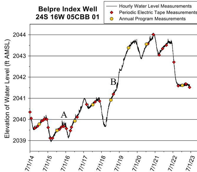
Figure 37—Belpre index well hydrograph—total data run to 6/5/23. A water-level elevation of 2,040 ft corresponds to a depth to water of 40 ft below Isf. The top of the 20 ft screen is 89 ft below Isf (elevation of 1,991 ft), and the bottom of the screen is 109 ft below Isf (elevation of 1,971 ft). The base of the aquifer is estimated to be 175–200 ft below Isf (elevation of 1,905–1,880 ft). A and B defined in text.
