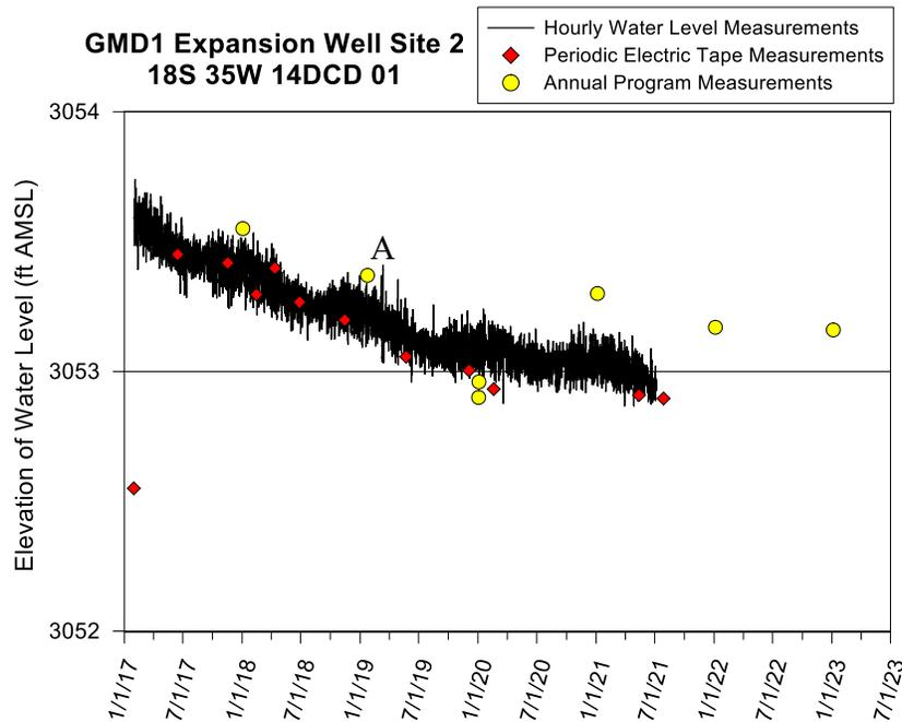
Figure 44—GMD1 Expansion Site 2 well hydrograph—total data run to 1/5/23. A water-level elevation of 3,053 ft corresponds to a depth to water of 118 ft below Isf. Bottom of well is 130.9 ft below Isf (elevation of 3,040.1 ft). First electric-tape measurement may be a transcription error. A defined in text.
