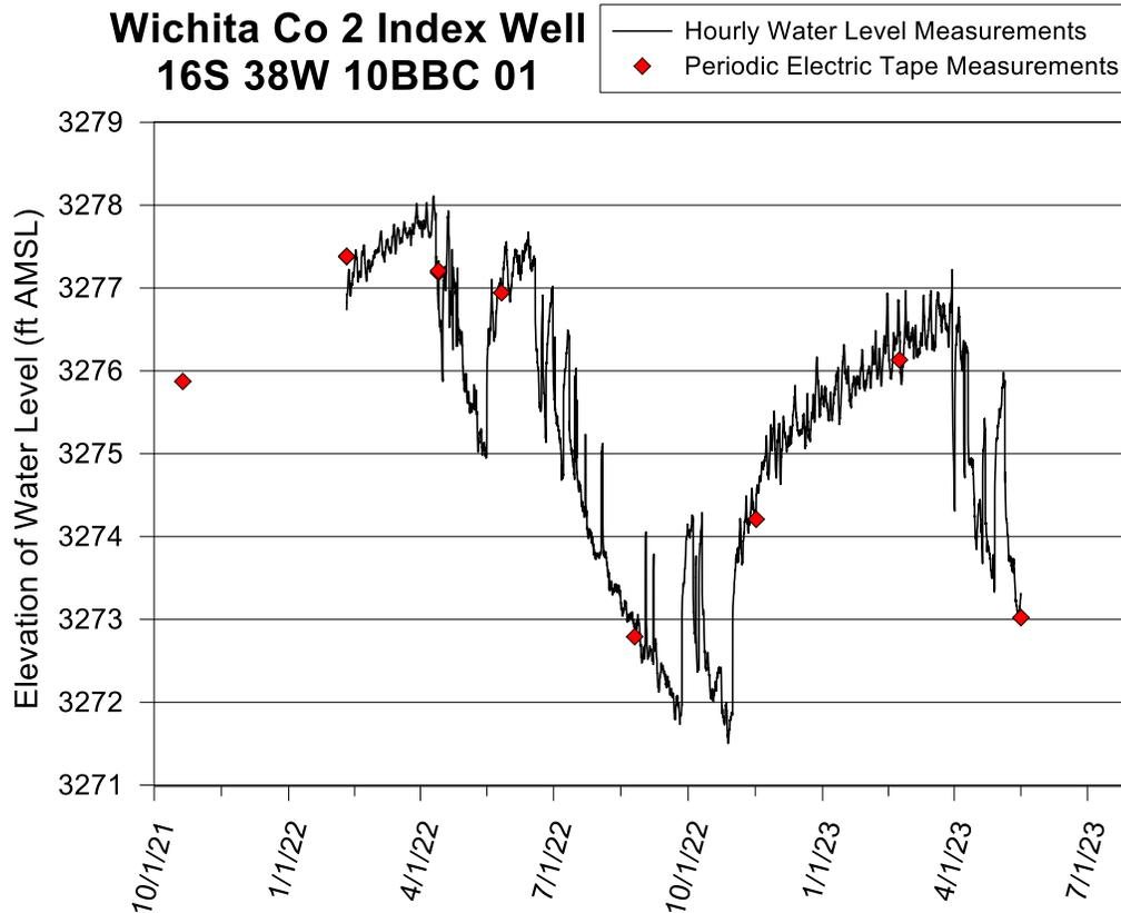
Figure 7—Wichita County 2 index well hydrograph—total data run to 5/16/23. A water-level elevation of 3,277 ft corresponds to a depth of water of 182 ft below Isf. The top of the screen is 189 ft below Isf (elevation of 3,270 ft), and the screen extends to the bottom of the well. The aquifer bottom is estimated to be 221 ft below Isf (elevation of 3,238 ft); the well bottom is 226.2 ft below Isf.
