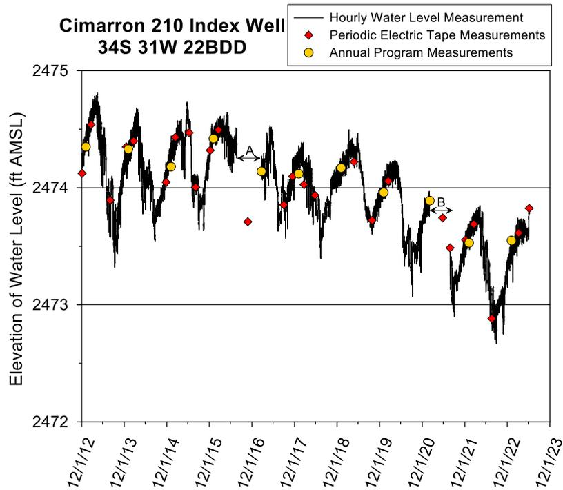
Figure 15—Cimarron 210 index well hydrograph—total data run to 6/6/23. A water-level elevation of 2,474 ft corresponds to a depth to water of 55 ft below Isf. The top of the 10 ft screen is 200 ft below Isf (elevation of 2,329 ft), and the bottom of the aquifer is 345 ft below Isf (elevation of 2,184 ft); A and B defined in text.
