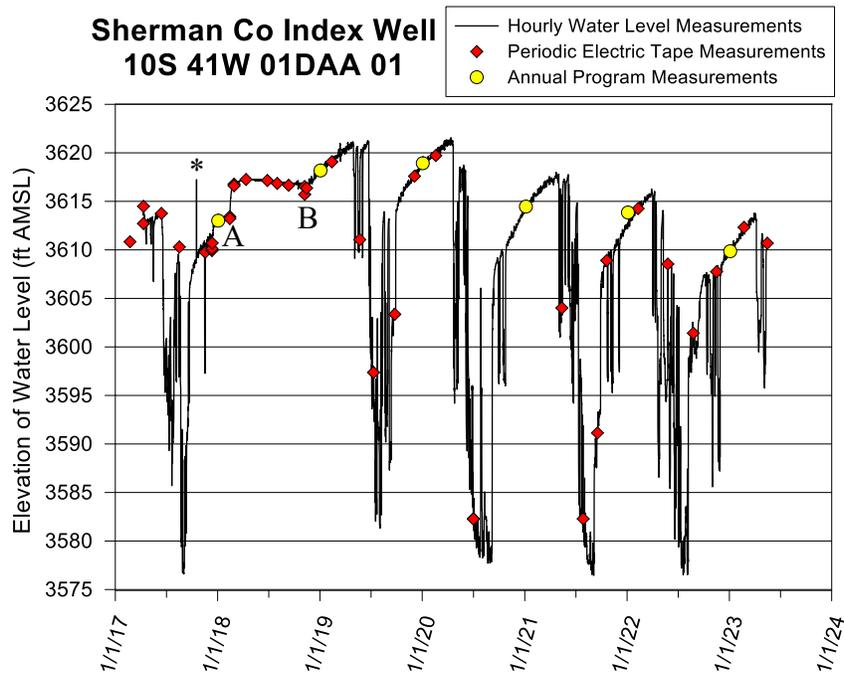
Figure 33—Sherman County index well hydrograph—total data run to 5/16/23. A water-level elevation of 3,615 ft corresponds to a depth to water of 179 ft below Isf. The top of the 10 ft screen is 310 ft below Isf (elevation of 3,484 ft), and the bottom of the aquifer is 323 ft below Isf (elevation of 3,471 ft). The well has a 10 ft sump that extends to 330 ft below Isf. The asterisk indicates a single spurious reading; A and B defined in text.
