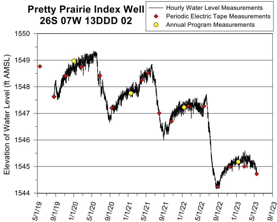
Figure 13—Pretty Prairie index well hydrograph—total data run to 5/17/23. A water-level elevation of 1,548 ft corresponds to a depth to water of 21 ft below lsf. The top of the 10 ft screen is 61 ft below lsf (elevation of 1,508 ft), and the bottom of the screen and aquifer is 71 ft below lsf (elevation of 1,498 ft).
