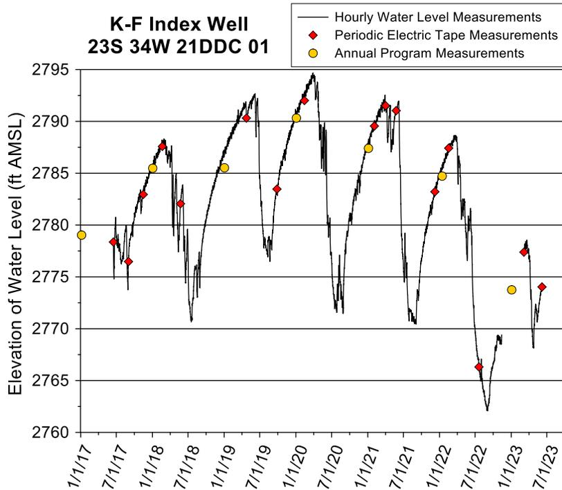
Figure 18—Kearny-Finney (K-F) index well hydrograph—total data run to 6/6/23. A water-level elevation of 2,785 ft corresponds to a depth to water of 176 ft below Isf. Nominal bottom of well is 300 ft below Isf (elevation of 2,661 ft), but the well is currently filled with sediments to 266 ft below Isf (elevation of 2,695 ft). Monitoring ceased on 11/13/22 after mice chewed through most of the sensor cable; cable was replaced and monitoring resumed on 3/6/23.
