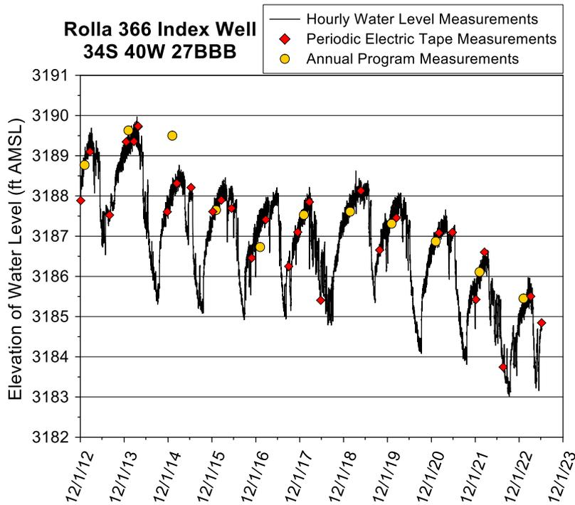
Figure 20—Rolla 366 index well hydrograph—total data run to 6/6/23. A water-level elevation of 3,188 ft corresponds to a depth to water of 187 ft below Isf. The top of the 10 ft screen is 356 ft below Isf (elevation of 3,019 ft), and the bottom of the aquifer is 399 ft below Isf (elevation of 2,976 ft). Note the suspect 2015 and 2017 annual program measurements.
