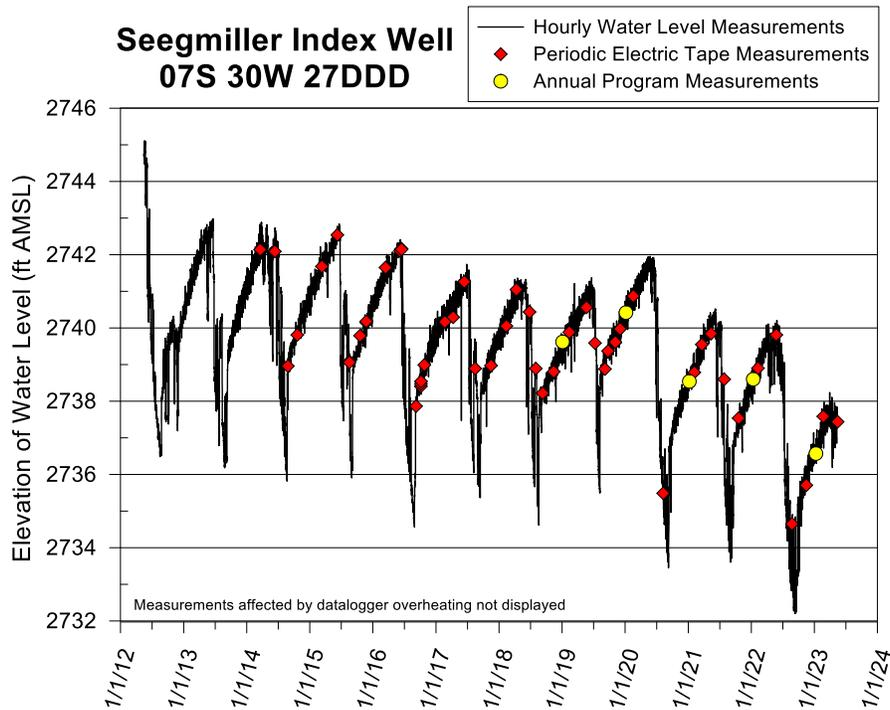
Figure 31—Seegmiller index well hydrograph—total data run to 5/15/23. A water-level elevation of 2,740 ft corresponds to a depth to water of 193 ft below Isf. The top of the 40 ft screen is 225 ft below Isf (elevation of 2,708 ft), and the bottom of the aquifer is 265 ft below Isf (elevation of 2,668 ft).
