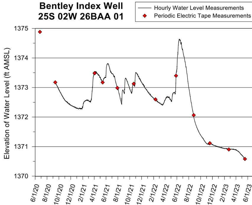
Figure 9—Bentley index well hydrograph—total data run to 5/17/23. A water-level elevation of 1,373 ft corresponds to a depth to water of 8.0 ft below Isf. The top of the 10 ft screen is 23 ft below Isf (elevation of 1,358 ft). The bottom of the aquifer is approximately 216 ft below Isf (elevation of 1,165 ft), and the bottom of the well is 33.0 ft below Isf (elevation of 1,348.0 ft).
