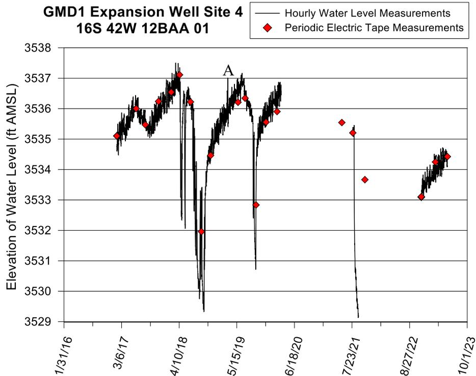
Figure 46—GMD1 Expansion Site 4 well hydrograph—total data run to 5/16/23, hourly measurements to 3/17/20, from 7/28/21 to 9/5/21, and from 11/16/22 on. A water-level elevation of 3,537 ft corresponds to a depth to water of 236 ft below Isf. Bottom of well is 264.5 ft below Isf (elevation of 3,508.5 ft). A defined in text.
