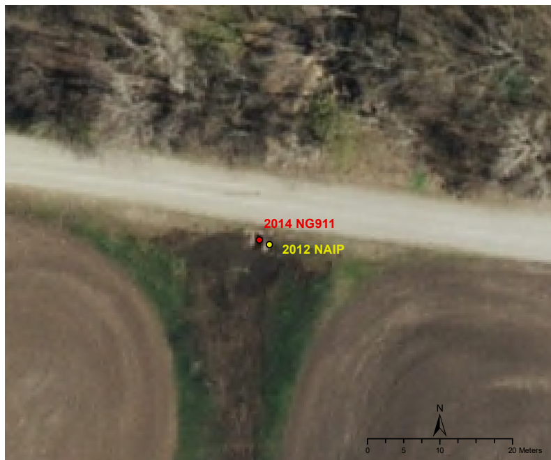
Figure 10. Image showing displacement of a fixed object (road culvert) between subsequent sets of historical imagery. Background image is 2014 NG911.
