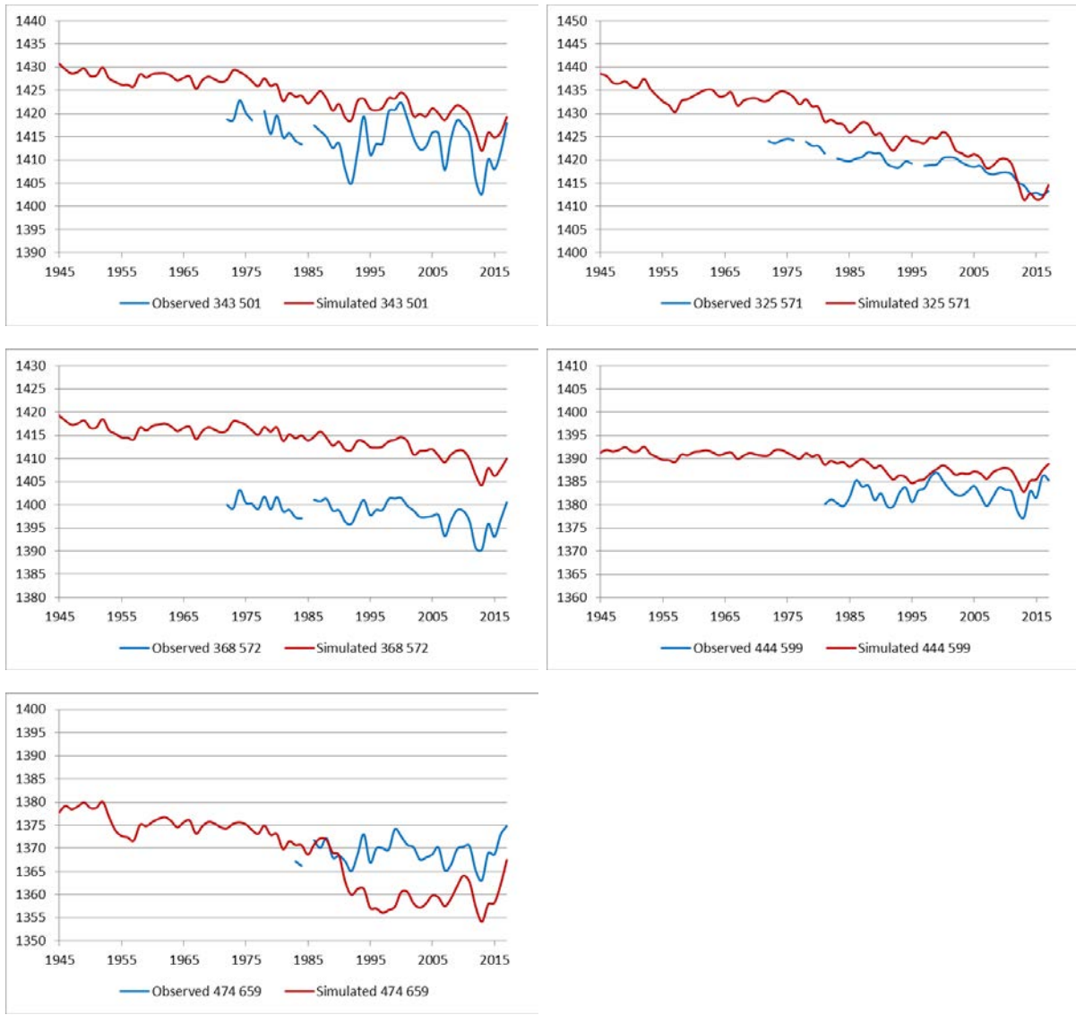
Figure 51. Simulated versus observed well hydrographs, Harvey County, north of the Little Arkansas River.
