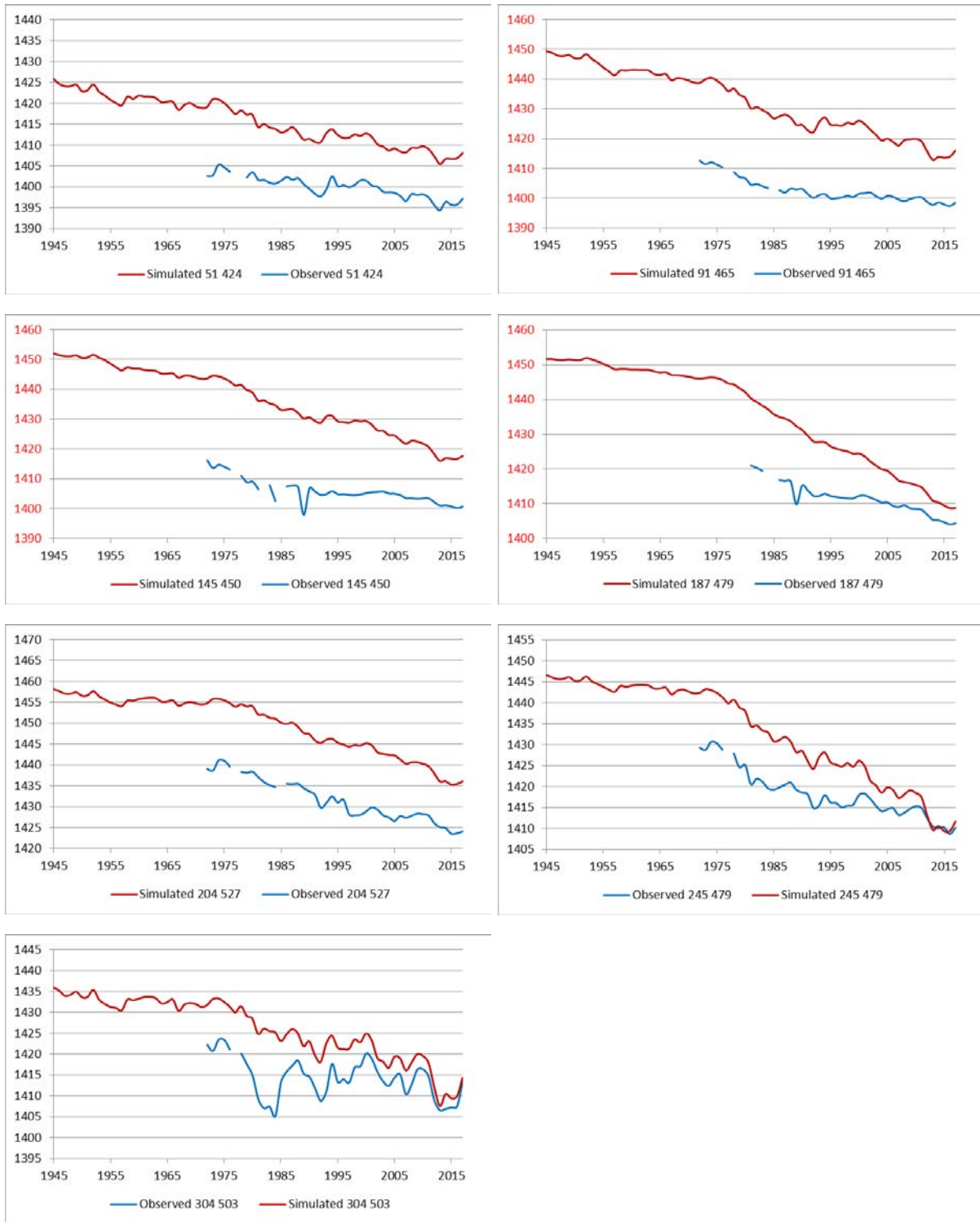
Figure 49. Simulated versus observed well hydrographs, central McPherson County.
