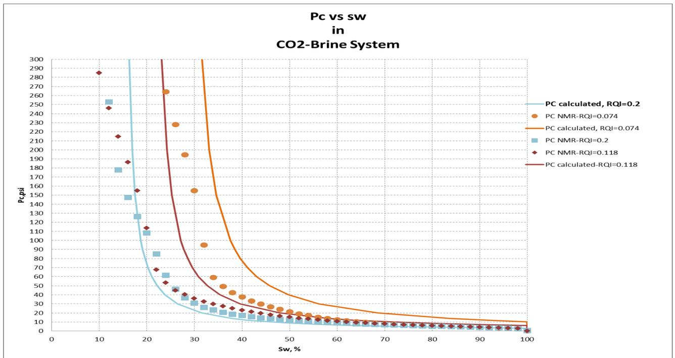
Figure 6: Calculated Pc compared with generated Pc from NMR
