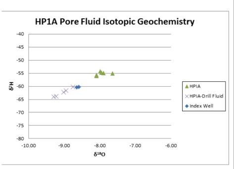
**Figure 6.** Stable isotopic analyses of pore fluids captured at depth via the Rotosonic drill rig showing that ground water from the upper (triangles) aquifer is isotopically distinct from that of the lower aquifer (crosses).
