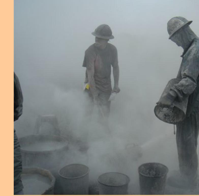
Obtaining cuttings at the blewie line at an air-drilled CBM well in eastern Kansas
