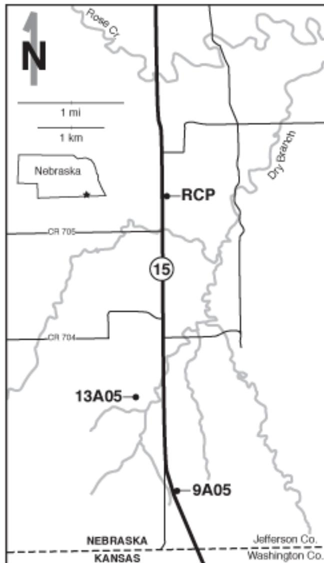
**Figure 1.** Geographic position of the three cores drilled in Jefferson County, Nebraska, as part of the involvement of the University of Nebraska–Lincoln Conservation and Survey Division in the U.S. Geological Survey's STATEMAP cooperative geologic mapping project. RCP = Rose Creek Pit. Core 9A05 will not be discussed in this study.
