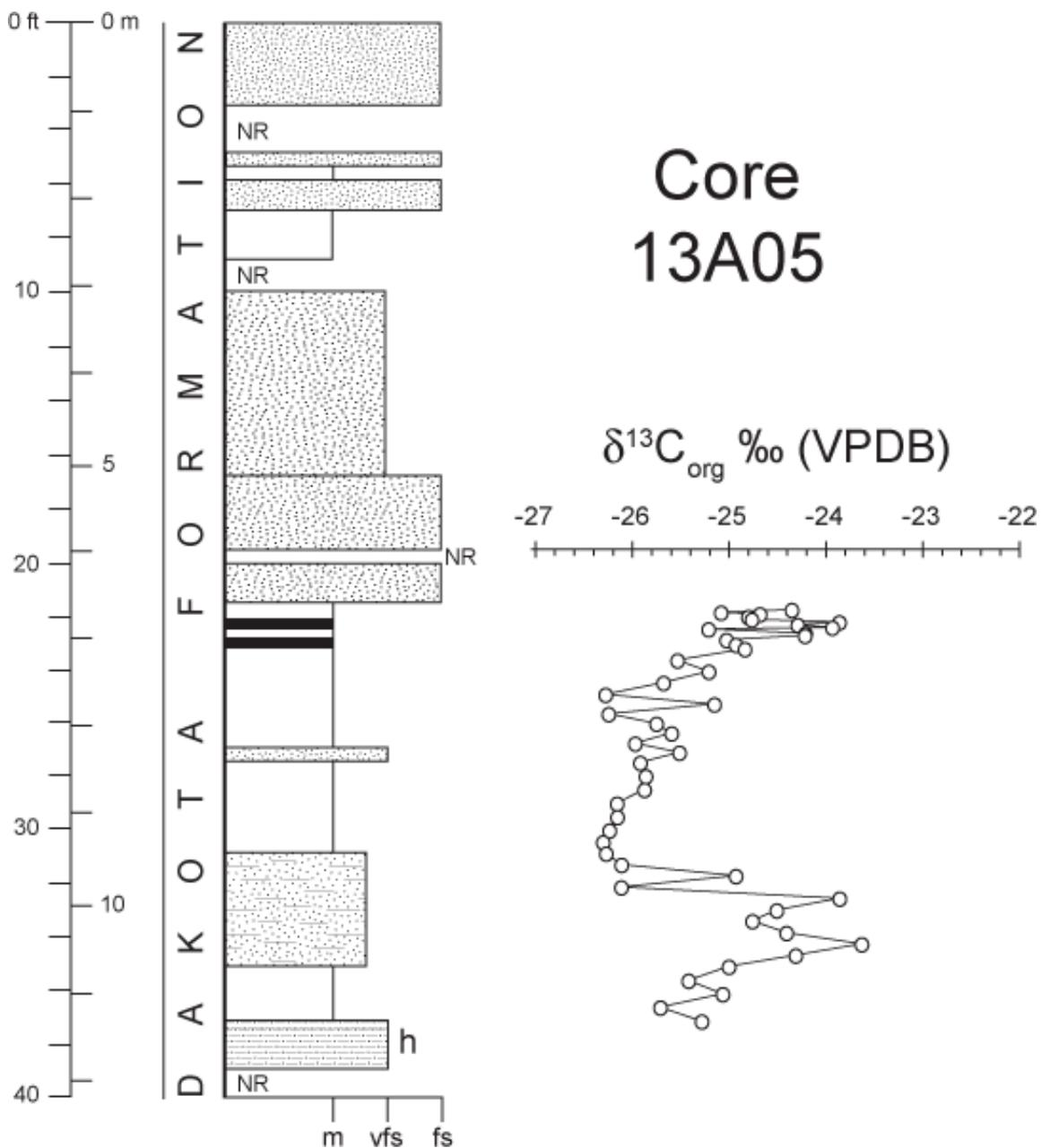
**Figure 3.** Stratigraphic section and  $\delta^{13}\text{C}_{\text{org}}$  record of core 13A05 spanning the upper part of the Dakota Formation, Nebraska. The  $\delta^{13}\text{C}_{\text{org}}$  curve was only produced for the lower segment of this core: see text for details. See fig. 2 for key.
