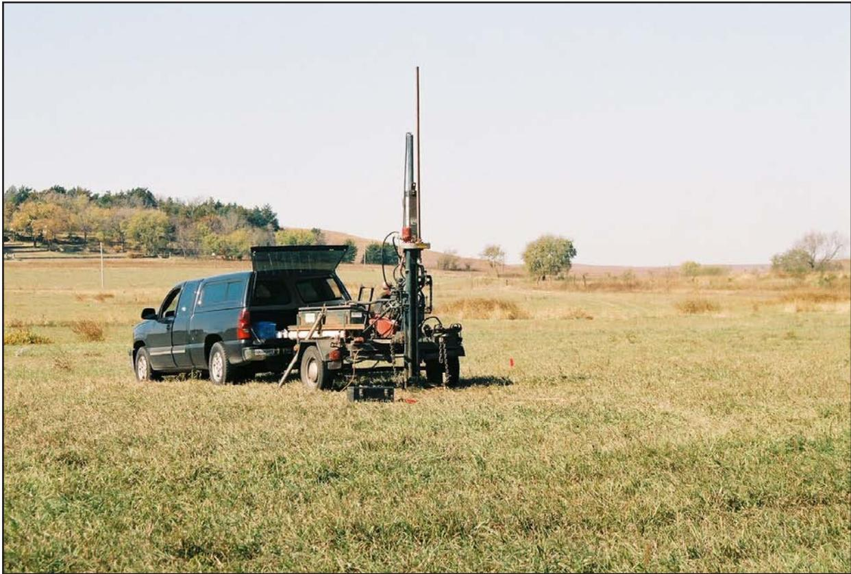
Figure 2. The trailer-mounted Giddings hydraulic soil probe used to collect cores in Fox Creek valley.
