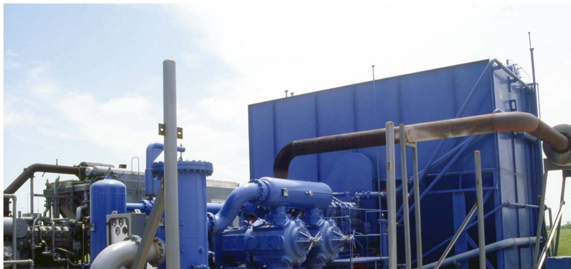
Figure 3. Dehydrator tower used by Dart Cherokee Basin Operating Co. to remove moisture, and minor impurities from the coal gas prior to passing through the Tallman Compressor Station. The tower is adjacent to the Tallman compressor.
