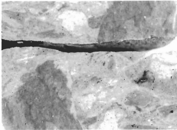
FIGURE 7—Burrow-mottled matrix sandstone from Collins conglomerate contains tiny fragments of white chert and Mississippian limestone; 4,455 ft. Scale in centimeters.
