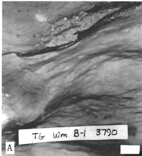
FIGURE 10A—Core slab of marlstone (unit 4) at 3,790 ft in the #1 Williamson "B" well. Lighter areas are carbonate mud rich and darker areas are green silty shale laminiae. The marlstone is very similar to that of unit 7 in figure 9A (scale is 1 cm).
