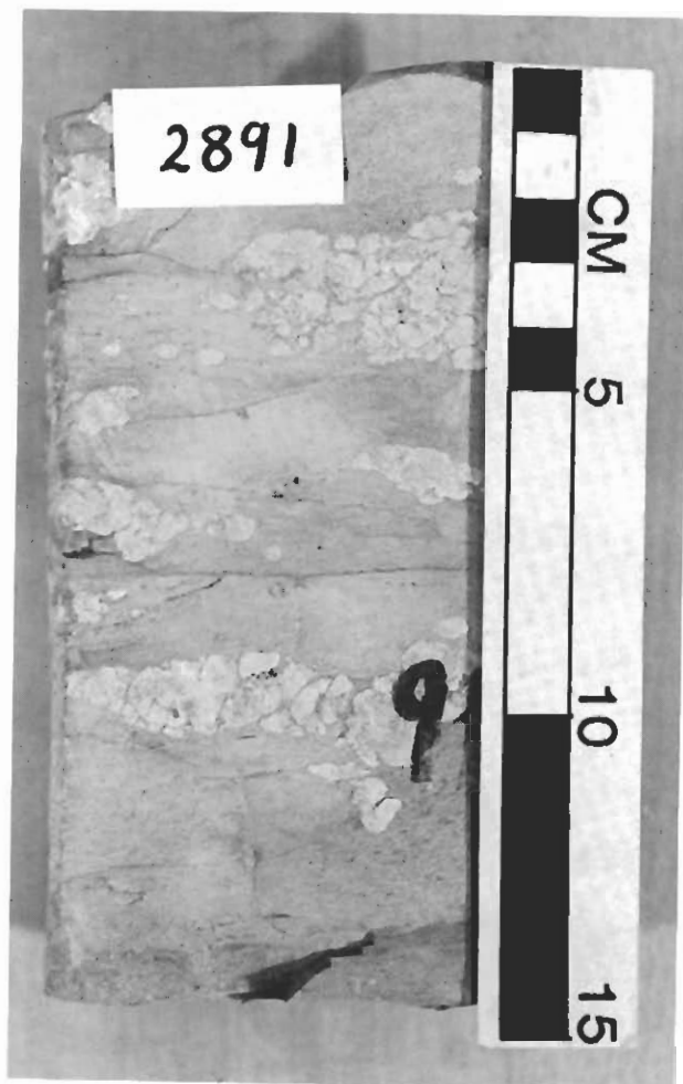
FIGURE 9—Core slab of lithofacies 6 (2,891 ft; Anadarko #C-1 Rhinehart Estate). Silty fossiliferous shale with chert nodules. Scale is in centimeters.
