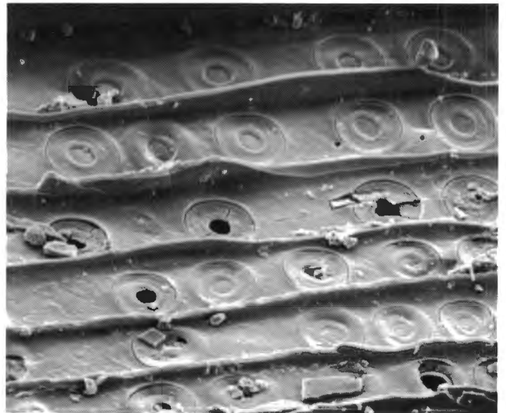
b) uniseriate-bordered pits with tori, from (a) x 512.
