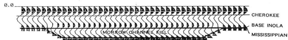
FIGURE 10—TWO-DIMENSIONAL MODEL DERIVED FROM SONIC AND DENSITY LOGS, Mesa Petroleum Seacat 7–19, 1,900 ft (570 m) FSL and 510 ft (153 m) FEL, sec. 19, T. 31 S., R. 21 W. Maximum channel thickness = 106 ft (31 m); Morrow thickness outside channel = 8 ft (2.4 m).
