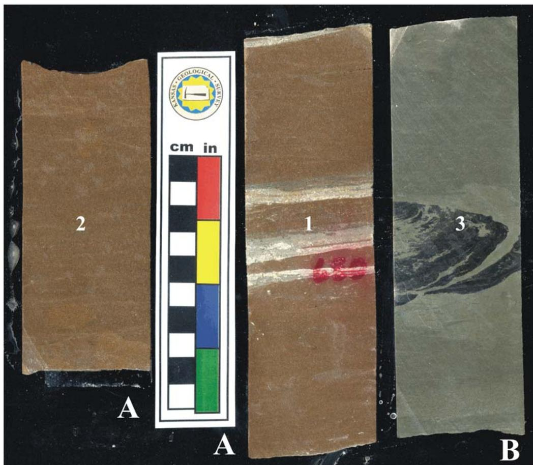
Figure 2.13 *Interbedded Sandstone and Siltstone Facies* (A) Continuous, scanned core image from the Franklin County well (left, 649.3'-649.7'; right, 649.7'-650.3'; upper Cherokee Group) displaying parallel, inclined sandstone and siltstone interbeds (1) coarsening upwards into very faint bidirectional ripple laminae (2). (B) Convolute sandy siltstone laminae (3) slightly lower in the same core (662.0'-662.5'; Appendix A).
