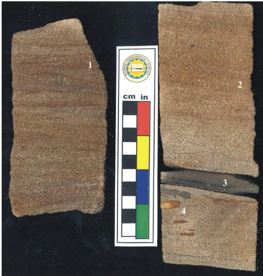
Figure 2.12 *Cross-Bedded Sandstone Facies* Scanned core image (nearly adjacent samples; left, 1039.1'-1039.7'; right, 1040.0'-1040.8') from the Rose Hill #1-6 well displaying faint thickly laminated to very thinly bedded trough- (1) and planar (2) - cross stratification (Johnson, 2004). Intermittent shale seams (3) and siderite mud clasts (4) are present in the facies.
