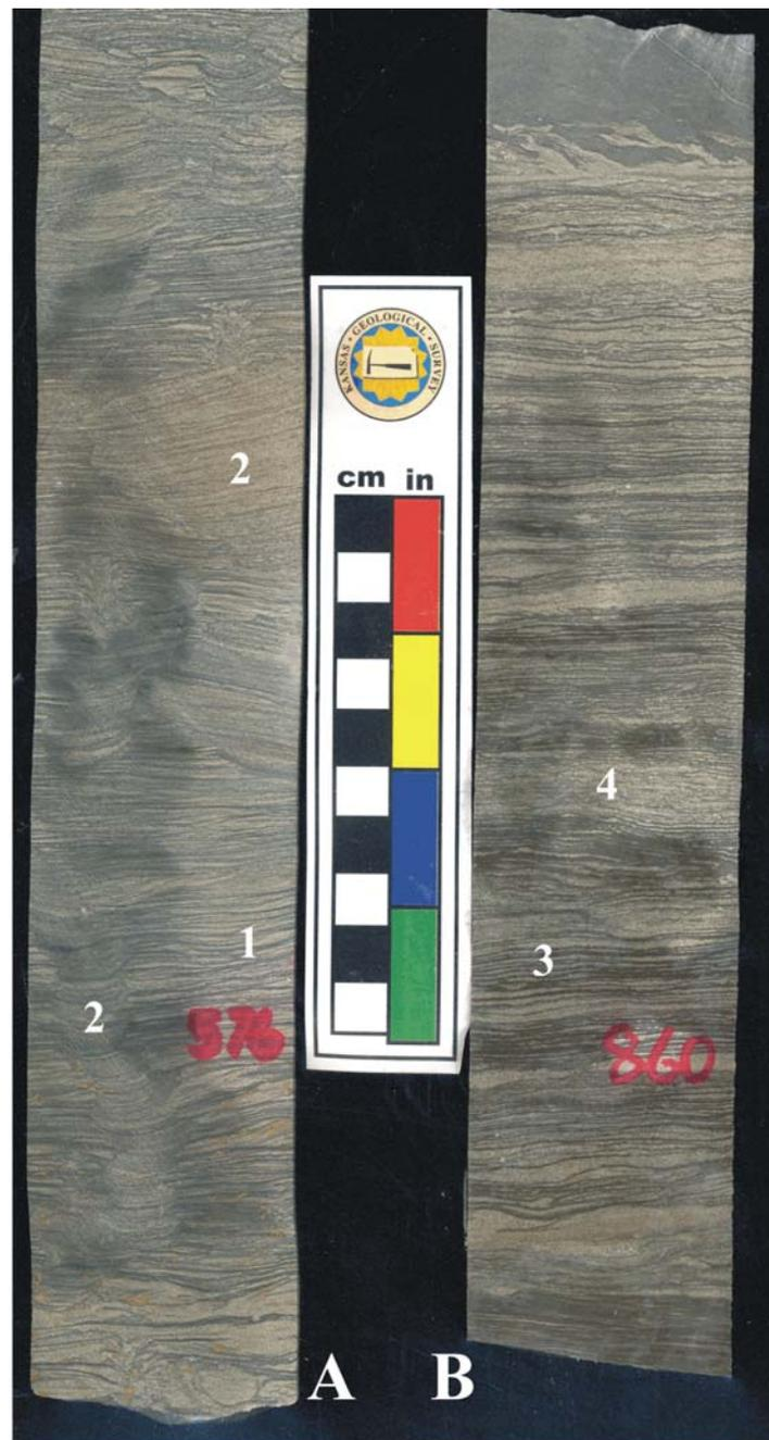
Figure 2.06 *Heterolithic Sandstone Facies* (A) Heterolithic sandstone facies within the Bandera Quarry Sandstone interval of the Franklin County core (575.1'-576.2') with heterolithic wavy laminae (1) and abundant *Teichichnus* burrows (2; Appendix A). (B) Scanned core image within the Upper Bluejacket sandstone interval of the Franklin County core (859.3'-860.2') displaying wavy laminae with sand-mud bundles (3) and thickening-thinning bundle sequences (4; Appendix A).
