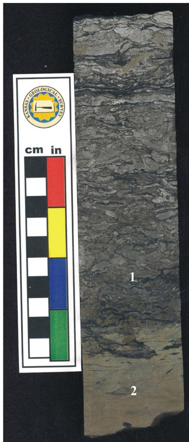
Figure 2.14 *Bioturbated Sandstone Facies* Scanned core image from the Franklin County well (973.1'-973.8') displaying extensively bioturbated sandstone facies (1) overlying the underclay facies (2; Appendix A). Sand and mud-filled burrows penetrate into the underclay facies.
