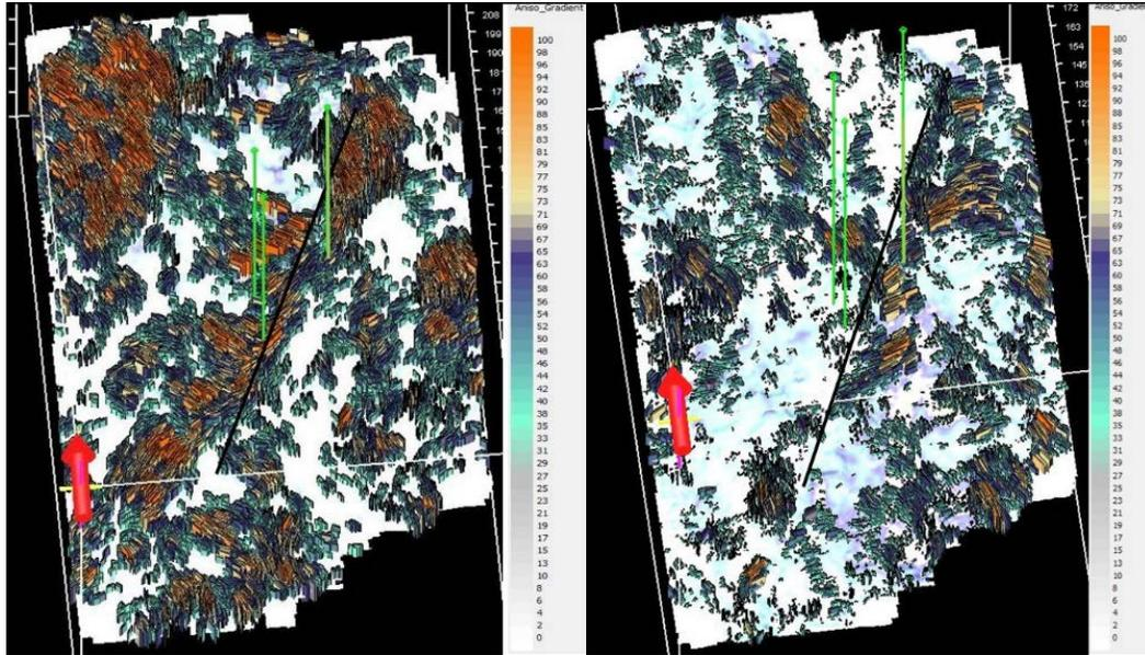
Figure 5. Tilted perspective of the azimuthal planes of isotropy at the Mississippian reservoir (anisotropy gradient 33%-100% in color) (left) and the Arbuckle (anisotropy gradient 25%-100% in color) (right). The orientation can be interpreted as fractures and stress direction, and the size and color is the degree of anisotropy. The black line delineates a fault mapped in the 3D seismic. Wells KGS# 1-32, 2-32 and 1-28 are shown in green (from left to right).
