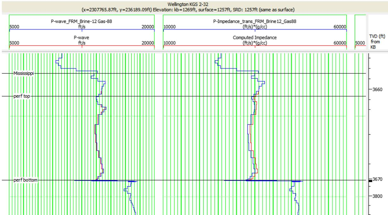
Figure 4. Fluid substitution model of P-wave velocity (left) and acoustic impedance (velocity \* density) (right) for the Mississippian CO<sub>2</sub> injection interval in KGS 2-32. Measured well curves are shown in red. Modeled curves in blue. Impedance and P-wave velocity decrease due to the presence of CO<sub>2</sub>
