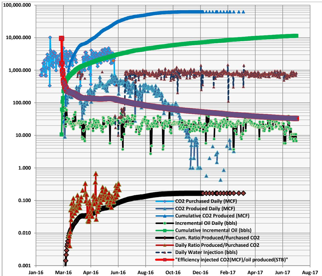
Figure 2. CO<sub>2</sub> injected and CO<sub>2</sub> and oil recovered in pilot scale injection in the Mississippian oil reservoir in Wellington Field.
