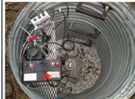
Housing setup for Sercel (Mark Products) L-22D-3D sensors, ~5 ft below surface to minimize surface noise; installed below frost line in bedrock
