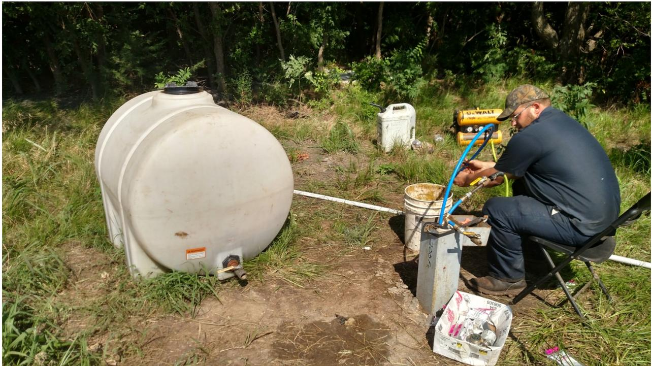
**Figure 9. Photo taken while purging the last 3' of fluid from SW-2.**
