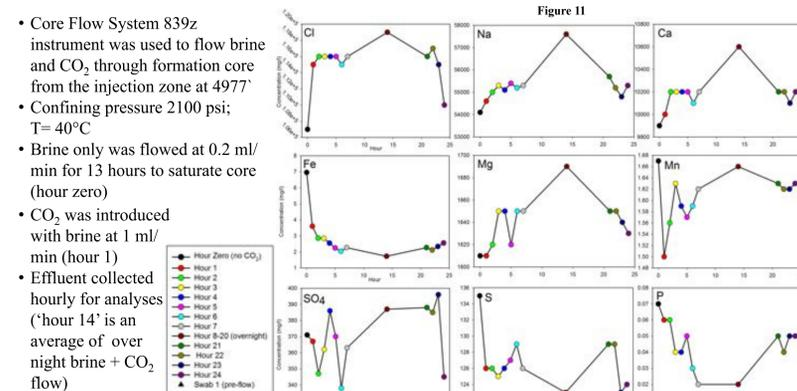
**Figure 11:** Time series (24 hour) analysis for CO<sub>2</sub>-brine flow-through experiment using formation water (swab 1; 5000-5020') and using core from 4977'. The values for pre flow brine were either higher (SO<sub>4</sub>, S, Mg, Ca, Na) or lower (Cl, Fe, Mn, P). The difference in brine compositions could be due to contamination or chemical changes prior to CO<sub>2</sub> introduction.
