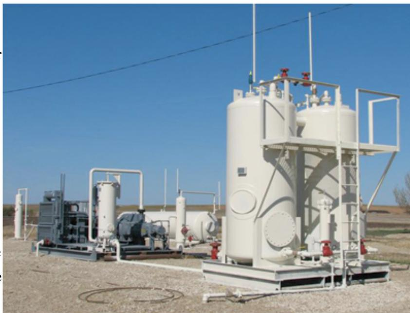
The micro-scale PSA upgrade unit at Elmdale field, Chase County, Kansas, is designed to handle up to 250 Mcf/d. The two towers are the vessels in which activated charcoal is placed to upgrade low-BTU feed gas using PSA (pressure swing adsorption) process. The surge tank that accepts the sales gas is in the background.
