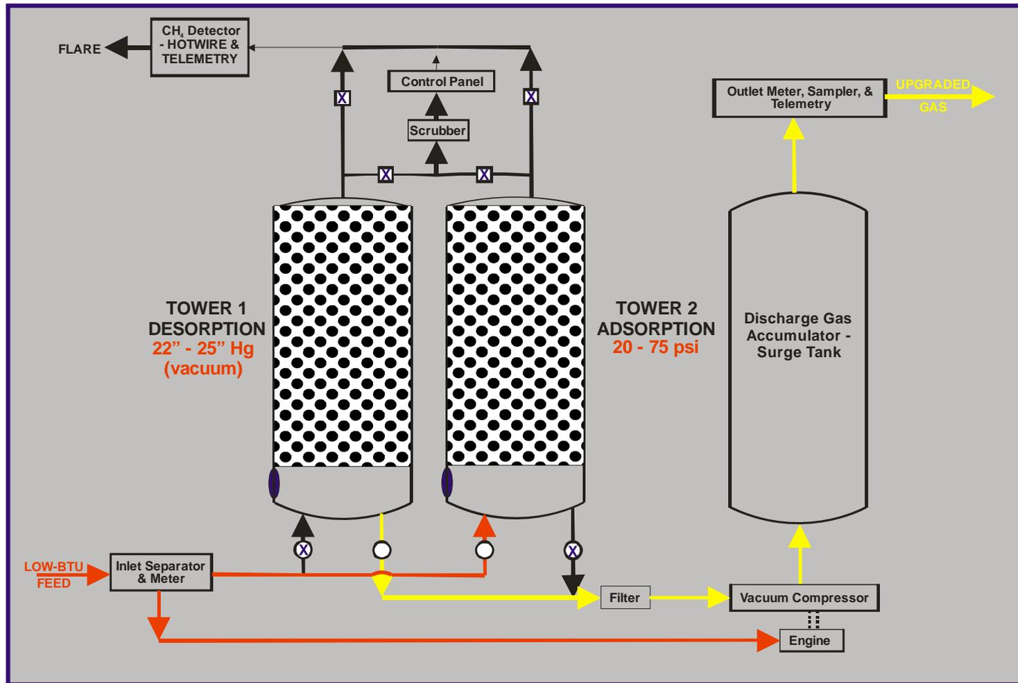
Figure 3: Third stage of operation - Tower 1 (after completion of the venting) is put under vacuum to evacuate the CH<sub>4</sub>-rich gas adsorbed in the activated bed while Tower 2 is connected to the feed line and gets charged.
