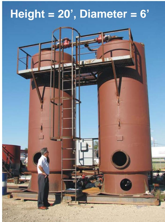
**Figure 14: Photograph of the new and larger plant that has been built by American Energies Corporation for installation in one of their low-BTU fields where the wells are currently shut for lack of availability of rich gas for blending.**
