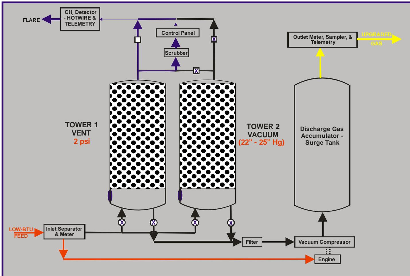
**Figure 2: Second step of operation - Tower 1 is vented to 2 psi after having been charged to the set pressure thus allowing the removal of N<sub>2</sub>-rich unadsorbed gas from the tower. This venting results in some loss of CH<sub>4</sub> but also prevents the unadsorbed N<sub>2</sub> from ending up in the surge tank during the desorption process. The vent period is very short (less than a minute for a plant of this size) and Tower 2 remains under vacuum during this time.**
