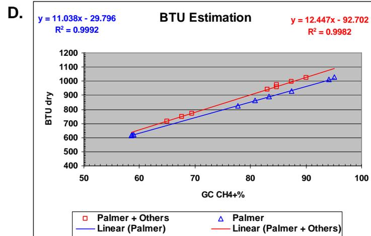
Figure 4: A) Portable gas meter that detects total hydrocarbons (handheld CH<sub>4</sub>+ %). B) Field sampling of the feed stream using portable meter. C) Correlation between portable meter (handheld CH<sub>4</sub>+ %) and gas chromatographic analyses (GC-CH<sub>4</sub>+ %). D) Correlation between gas chromatographic analyses and heat content.
