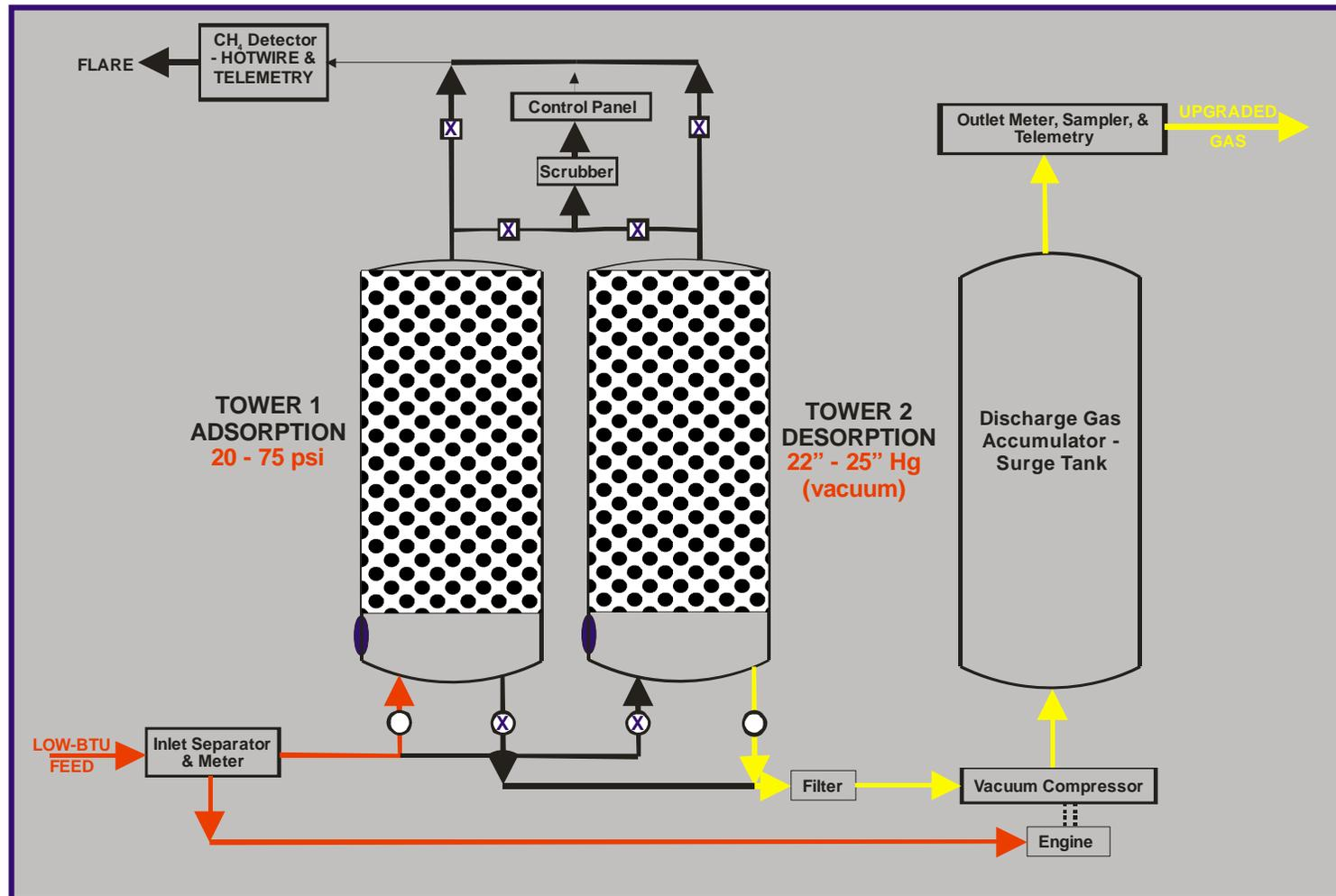
Figure 1: First step of operation - the feed gas charges up the evacuated Tower 1 to the set pressure (between 25 to 75 psi) depending on the plant settings determined by the feed gas quality, while Tower 2 is going through the evacuation process to vacuum ranging between 22 to 25 inches of Hg.
