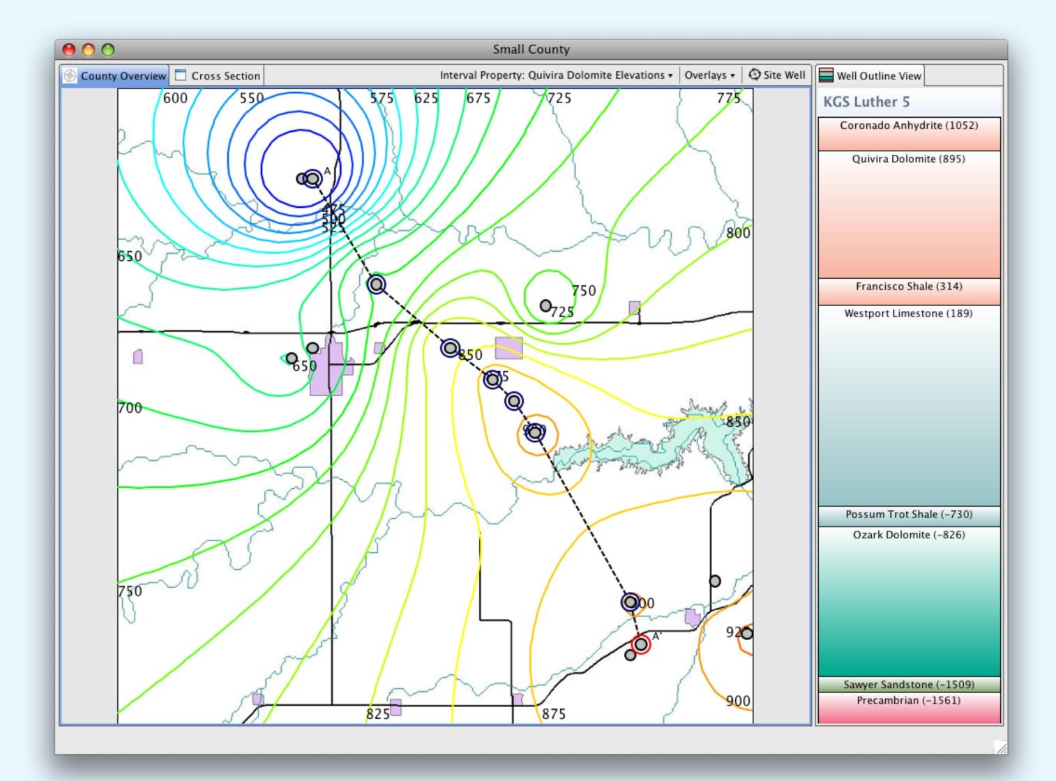
Figure 2 - County Overview wih set of wells for cross section (Figure 3) selected.
