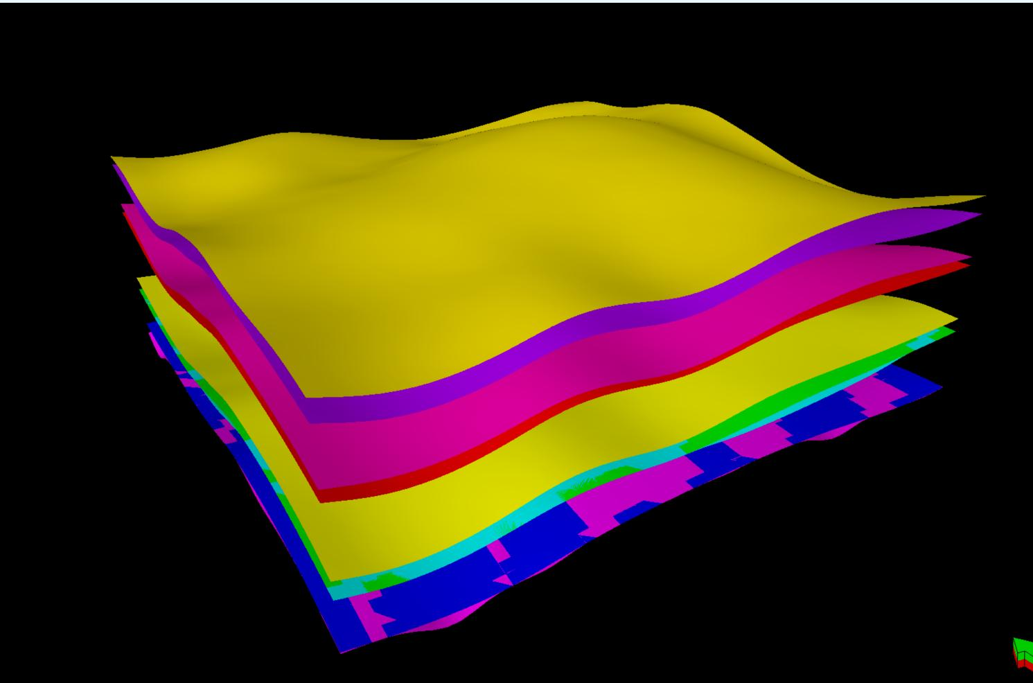
Figure 1 - One possible realization of major horizon elevations in the Small County subsurface. Elevations of the 9 horizons range from roughly 1500 feet below sea level to 1000 feet above sea level and the areal extent is 30 miles in each direction.
