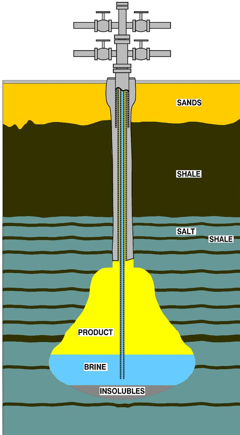
**Figure 2.** Schematic Illustration of a NGL/LPG Storage Cavern in a Bedded Salt Formation.
