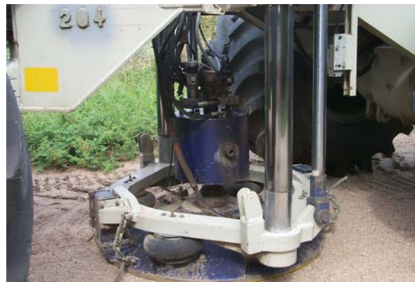
Figure A3. 300 lb mass and 300 lb baseplate with new prototype Atlas rotary valve.
