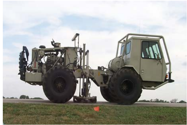
Figure A2. IVI minivib with Atlas rotary valve. Approximately 800 ft-lbs of force can be applied at 100 Hz, while around 2000 ft-lbs are possible in some conditions at 250 Hz.
