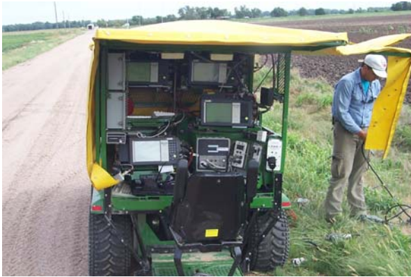
Figure A1. 240 channel Geometrics StrataView with support electronics (line checker, IVI source synchronizer, time break conditioner, etc.).
